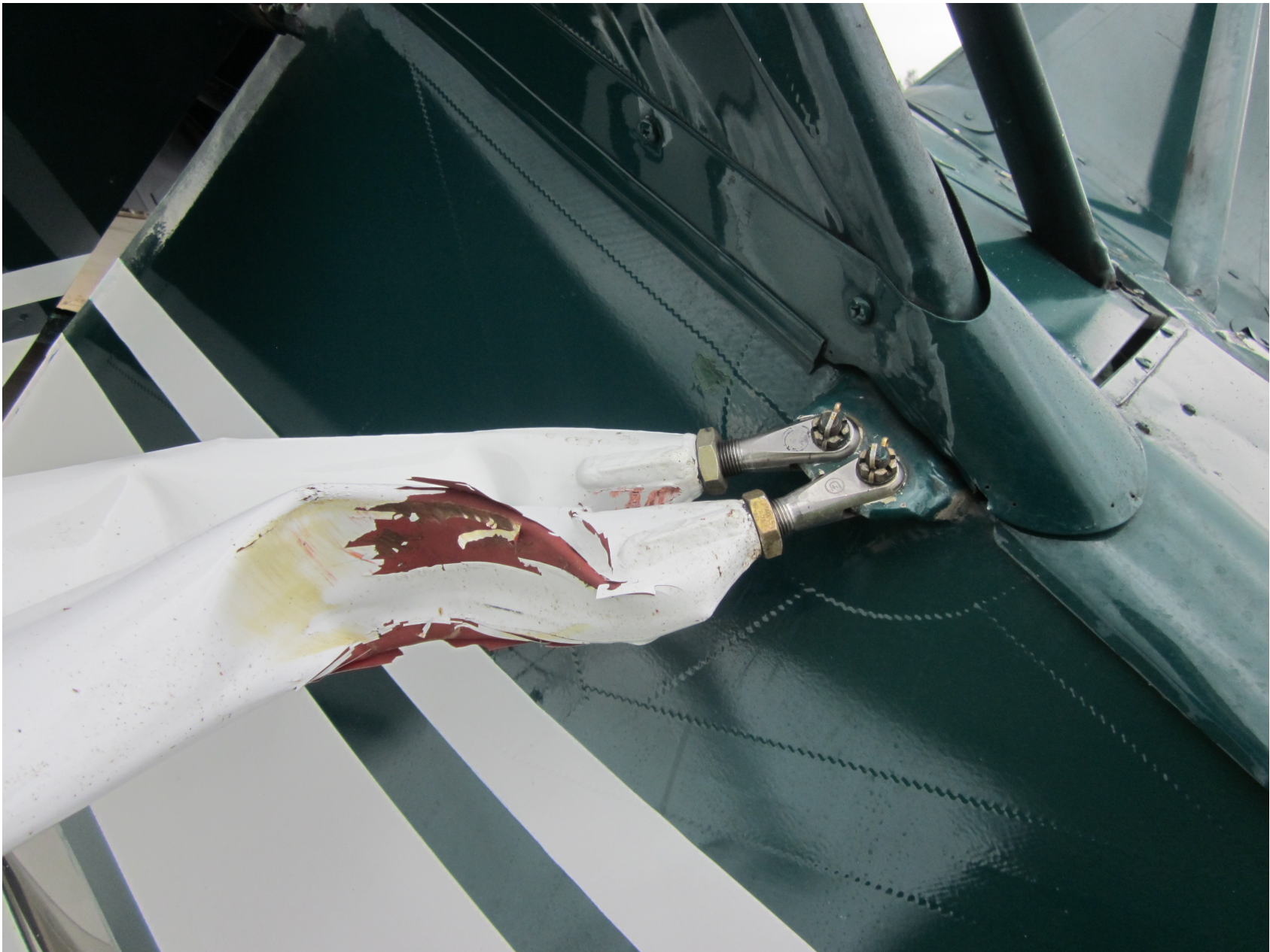
Photo 3 – View of Damaged Wing Strut (FAA)
