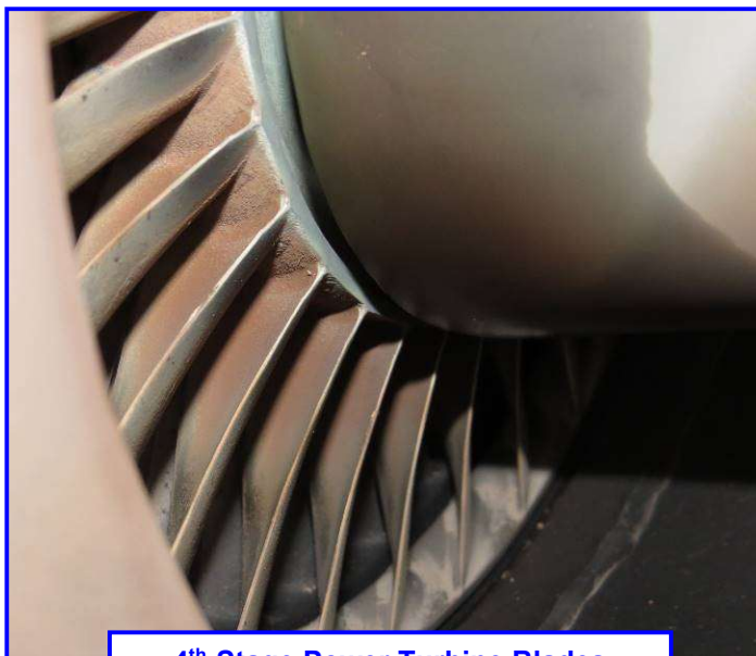
4 th -Stage Power Turbine Blades
