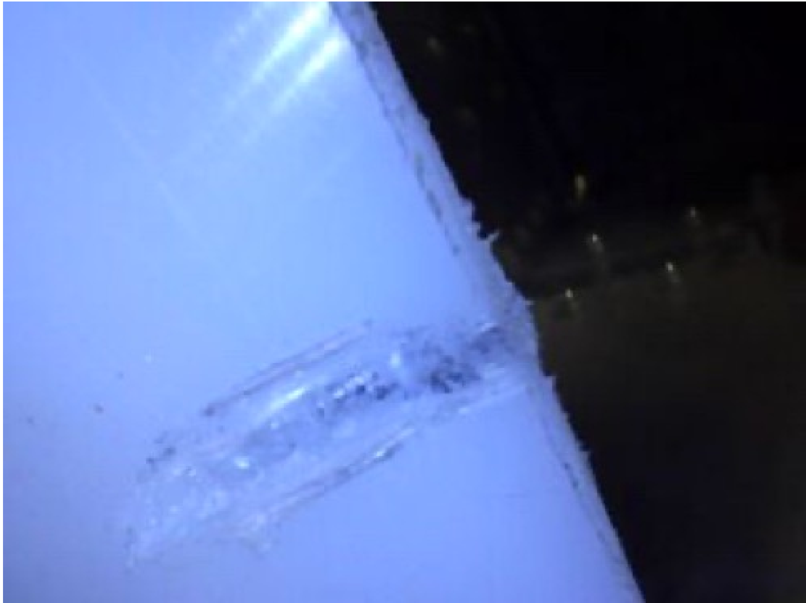
Photo 5– top view of nylon stop with elevator bracket impressions
