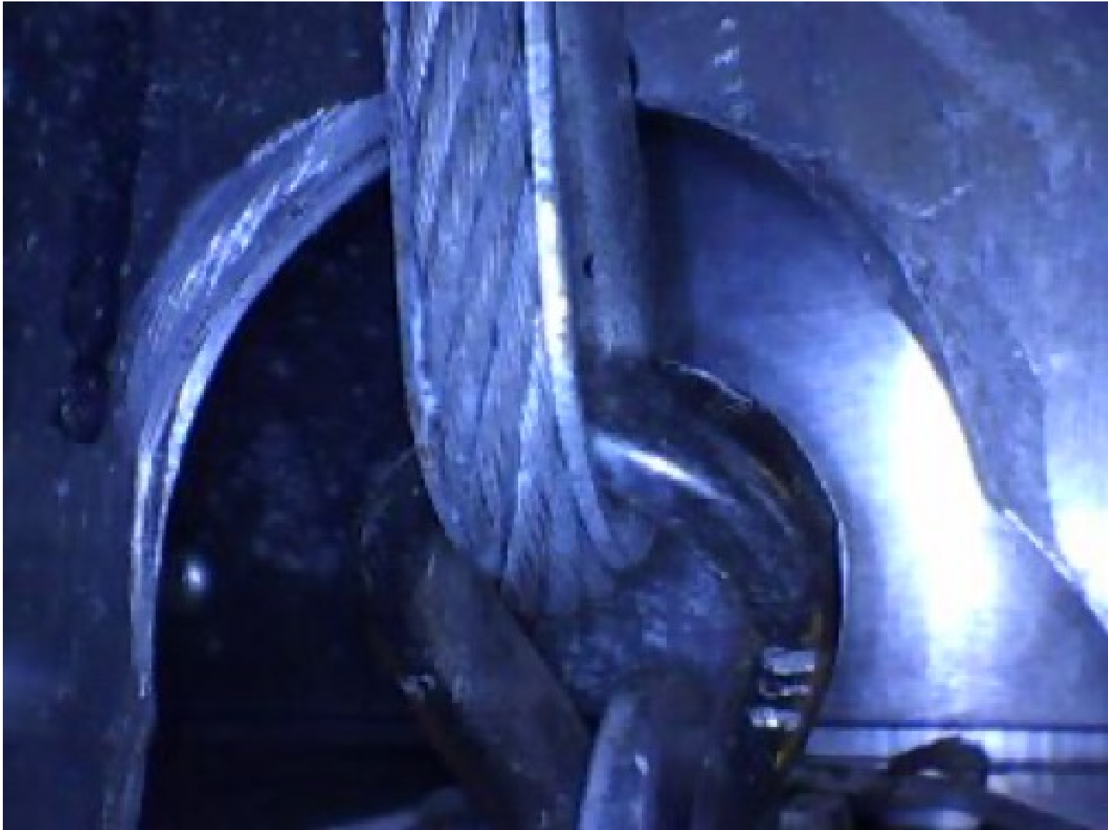
Photo 8 – tail section damage by loose cables
