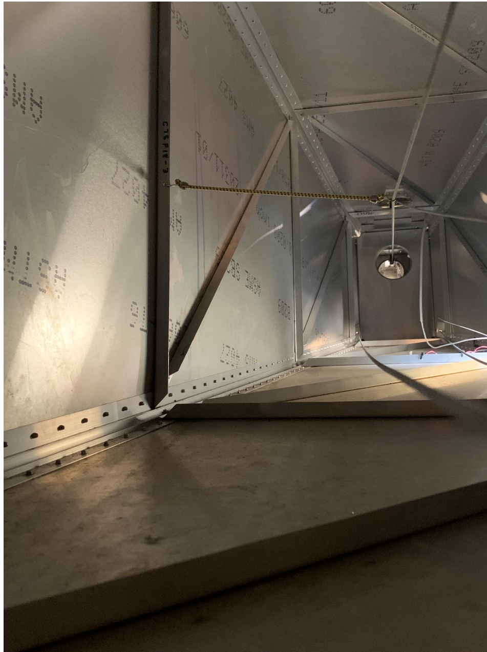
Photo 9 – Elevator and rudder cables loose and held with bungy cord
