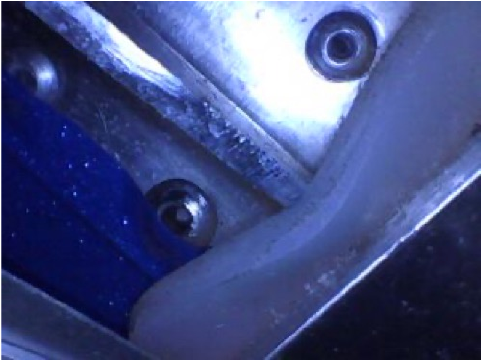
Photo 3 – bottom view of elevator bracket jammed on nylon stop
