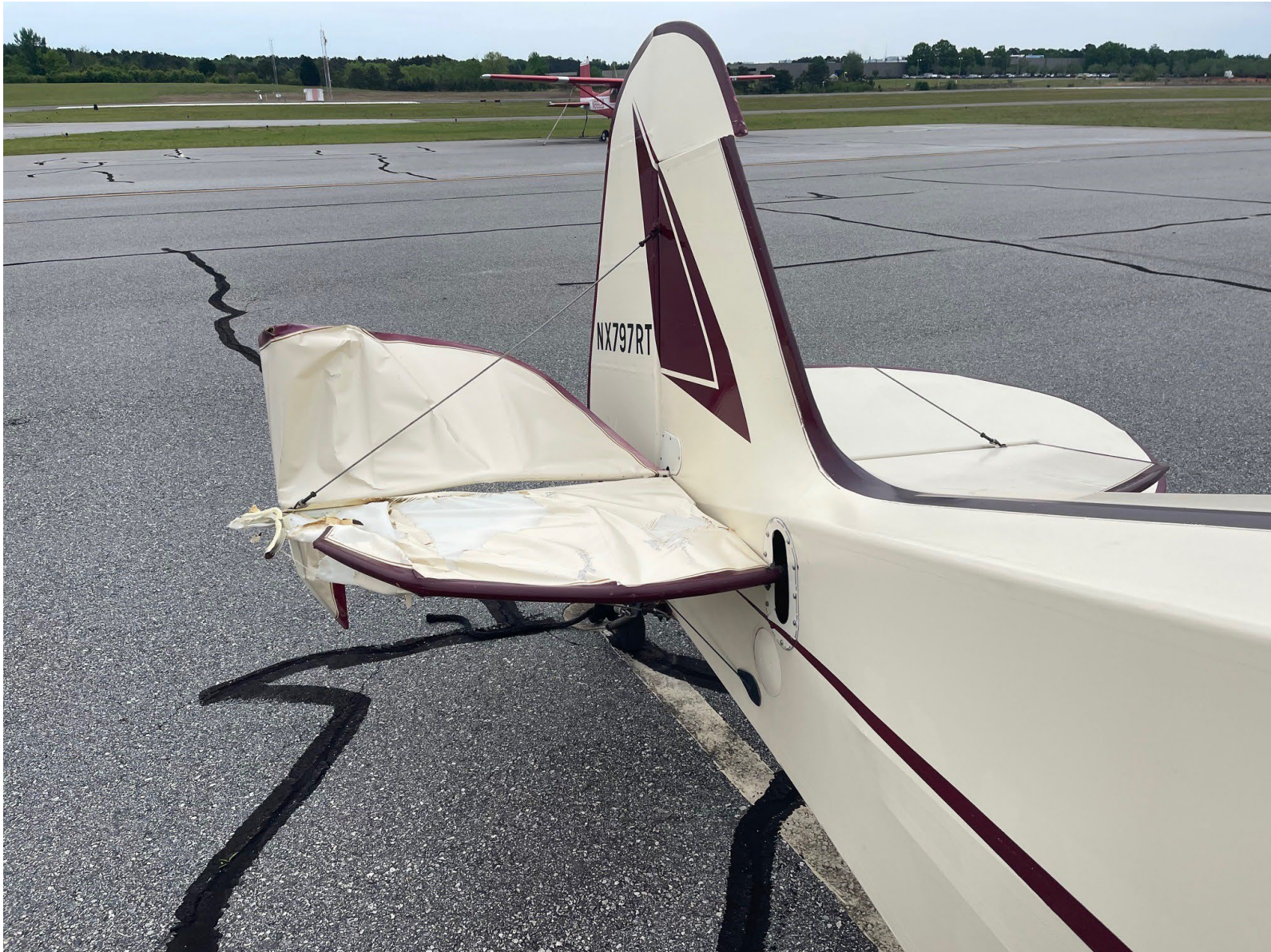
Photo 2 – Photo of right horizontal stabilizer and elevator damage. (Courtesy of FAA)
