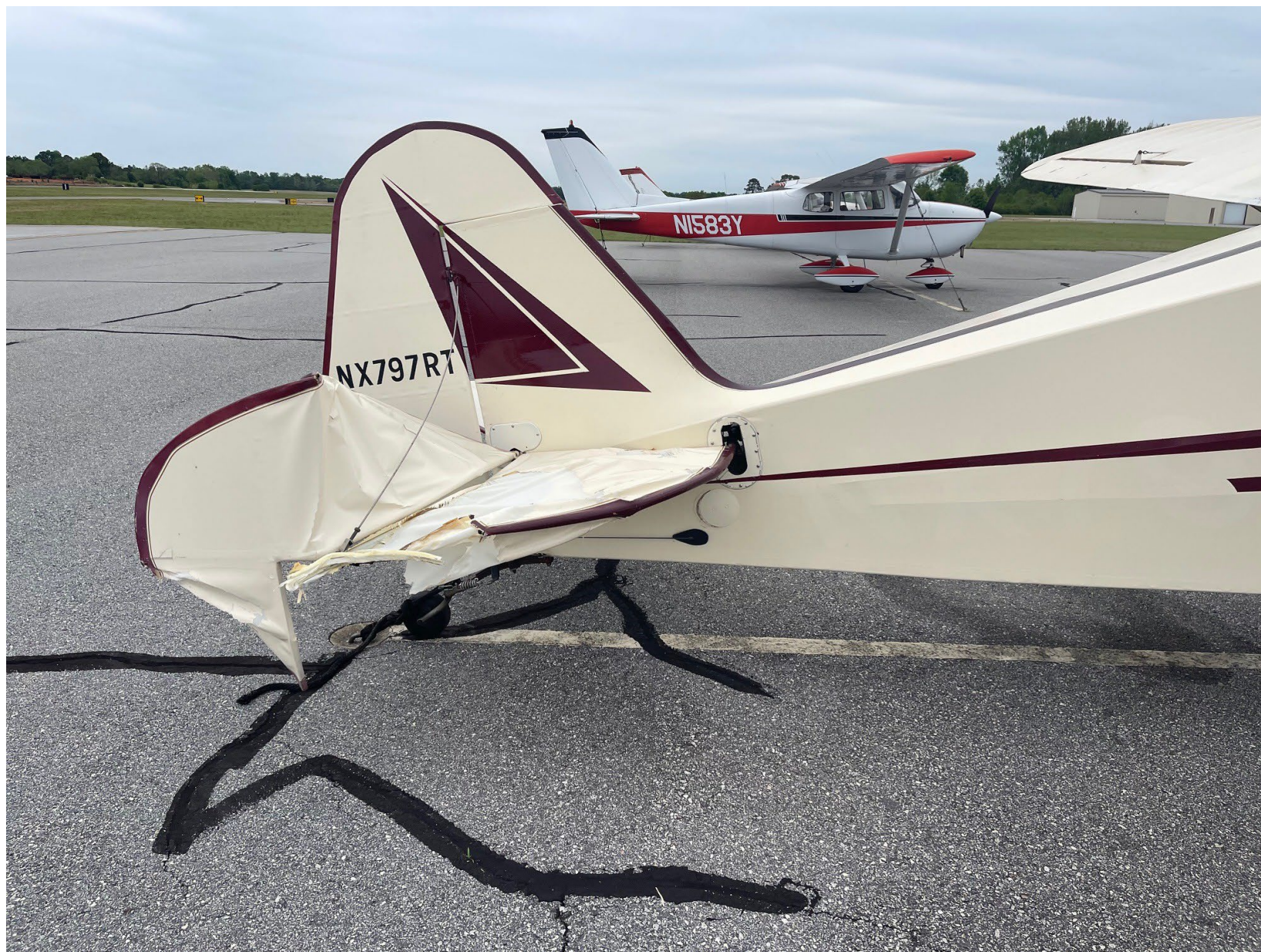
Photo 3 – Photo of side view of elevator and stabilizer damage. (Courtesy of FAA)
