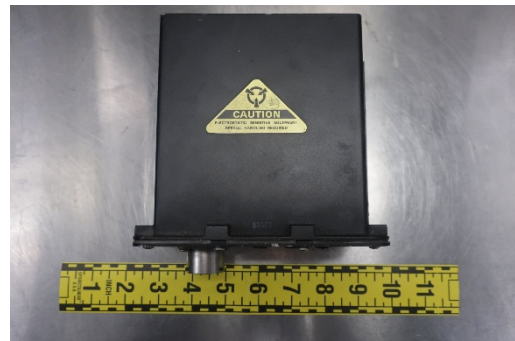
Photo 9 - Overhead view of the digital skid control box.
