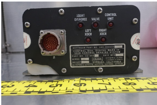
Photo 8 - Front face of the digital skid control box.
