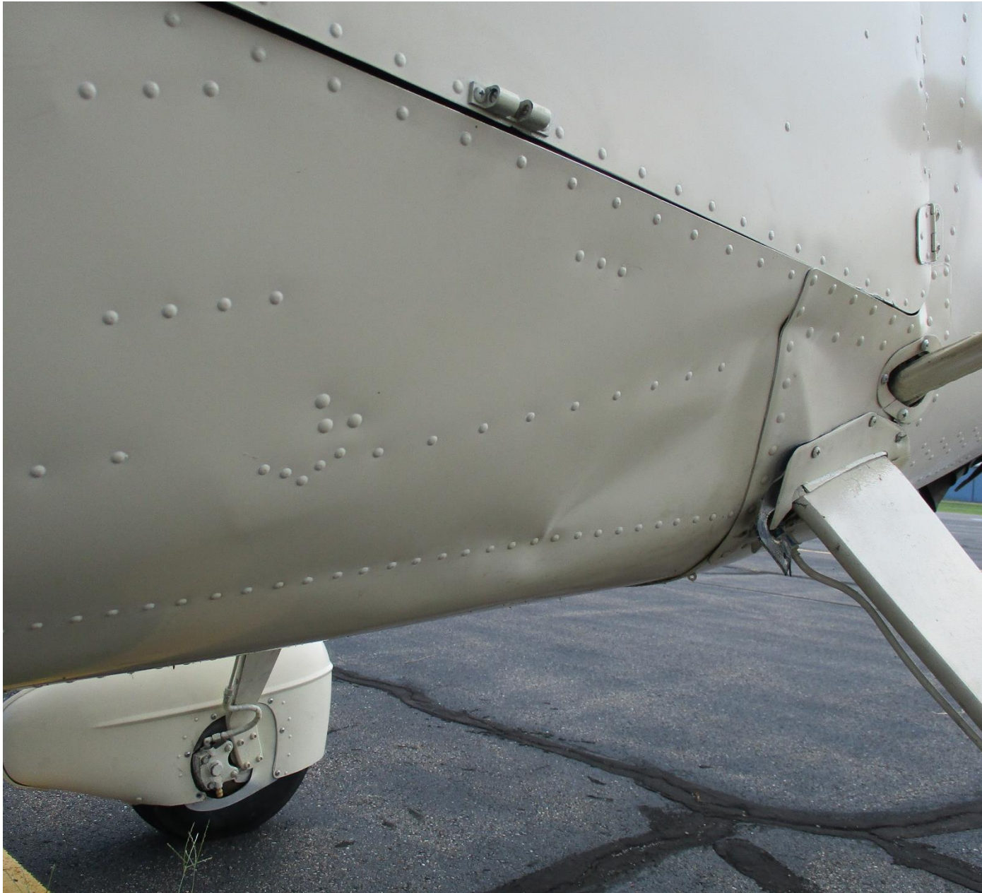
Photo 2 – Airplane – View of Fuselage Buckling (photo courtesy FAA)
