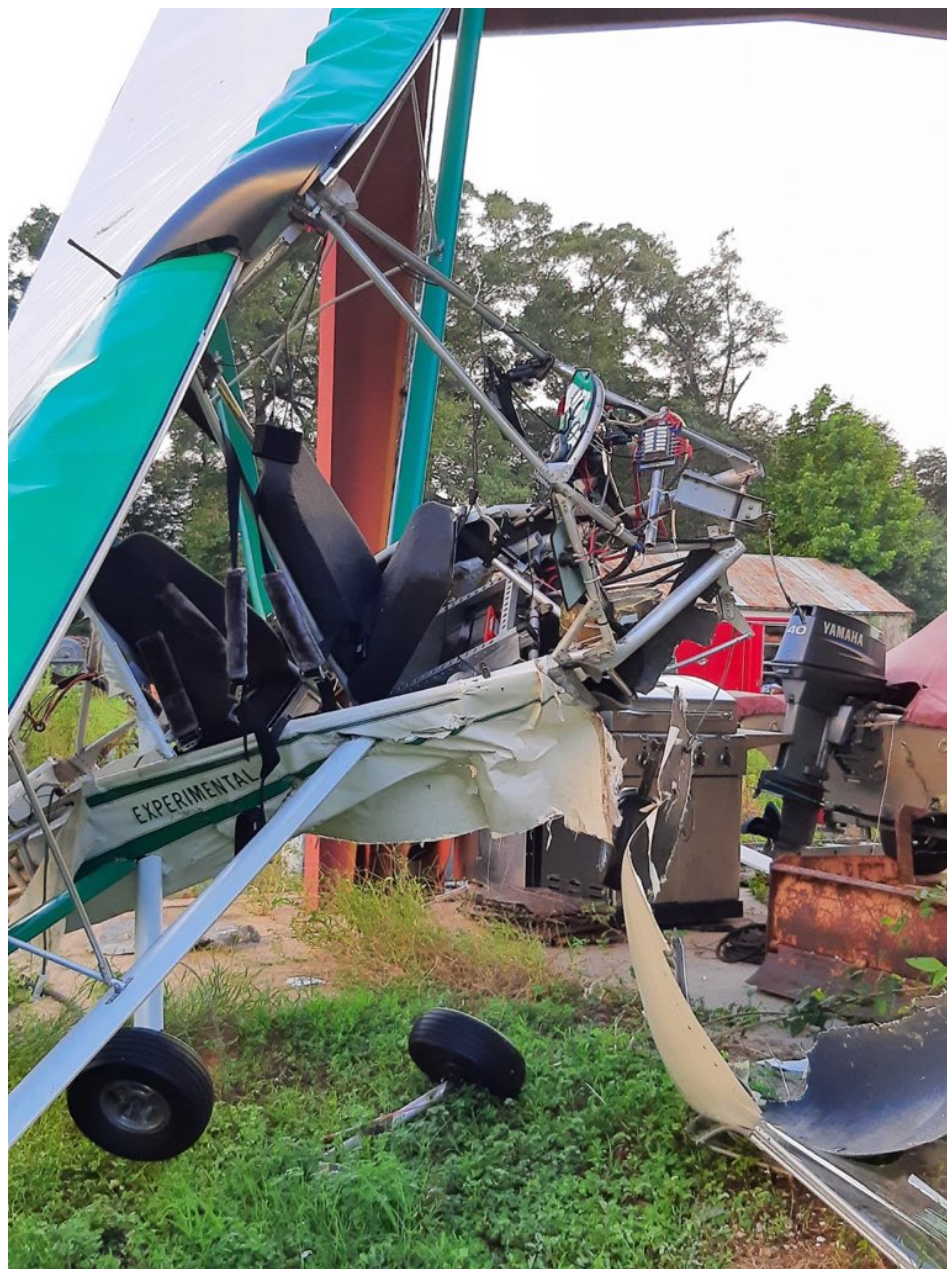
Photo 2 -Front view of aircraft showing damage (FAA photo)
