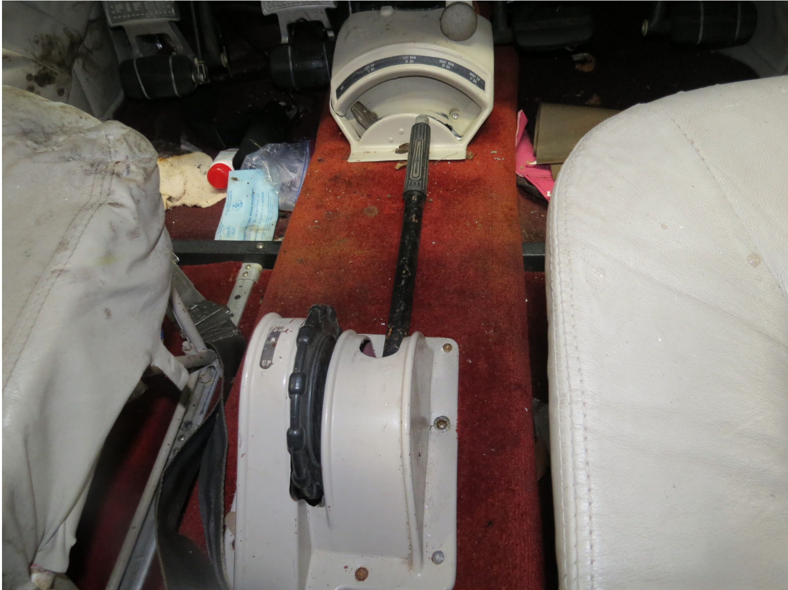
Photo 9 – View of flap, trim and fuel selectors. Note fuel selector in off position, but after the accident it was found on the Left tank. (Courtesy of Piper)
