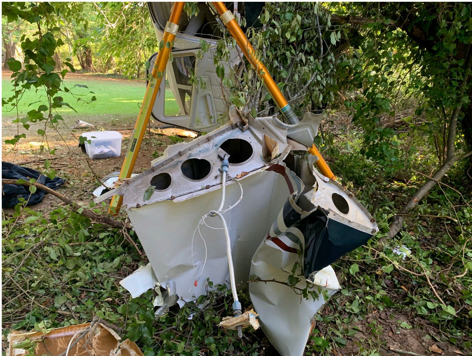
Photo 5 – Closeup view of left wing damage. (Courtesy of FAA)
