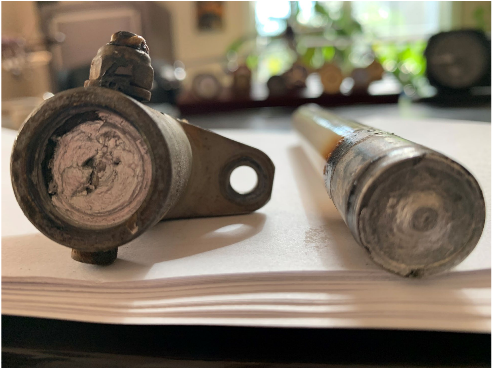
Photo 5 – driveshaft coupling, plug
