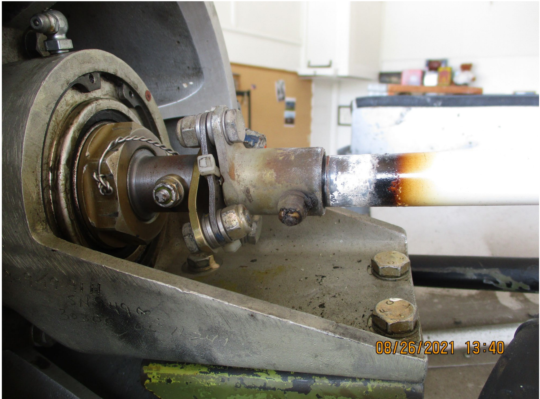
Photo 4 – driveshaft with burn pattern
