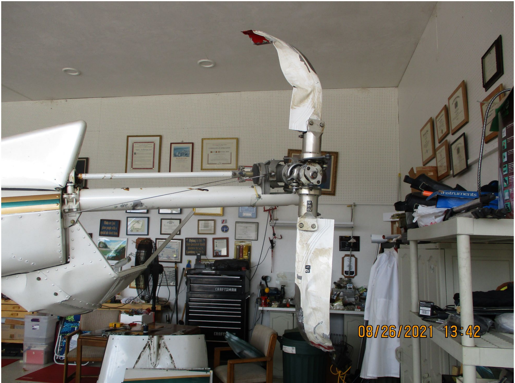
Photo 3 – tail rotor strike, bent blades
