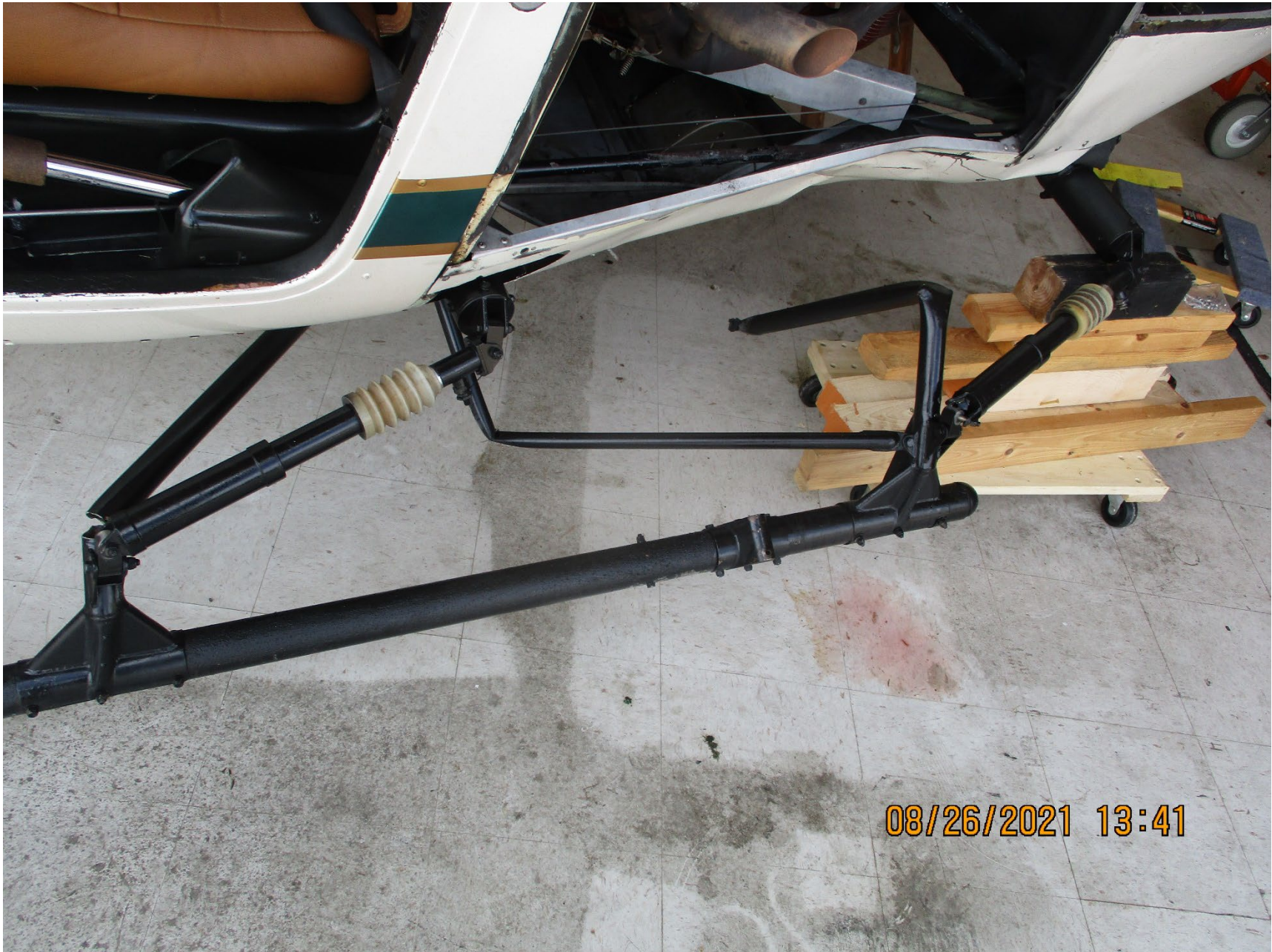
Photo 2 – skid, fuselage damaged
