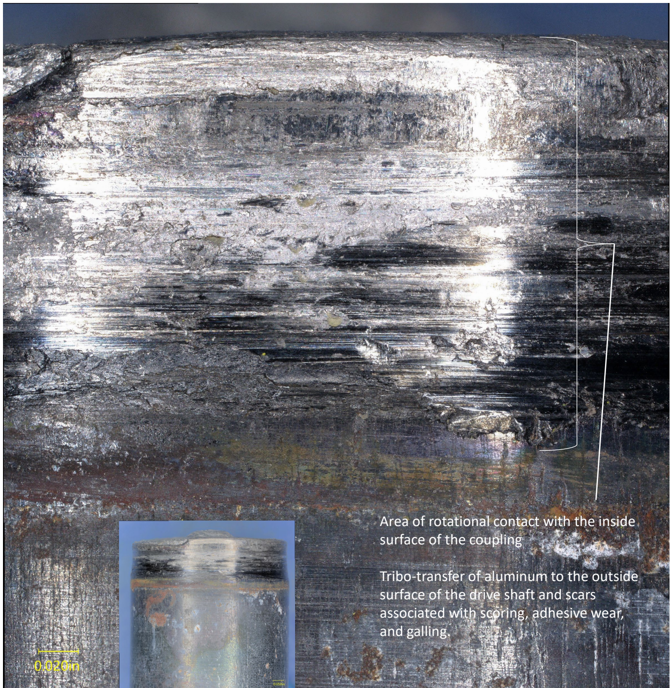
Figure 12 Closer side view of the fractured end of the as-received drive shaft tube showing rotational contact damage on the outside diameter of the drive shaft where it mates with the coupling.
