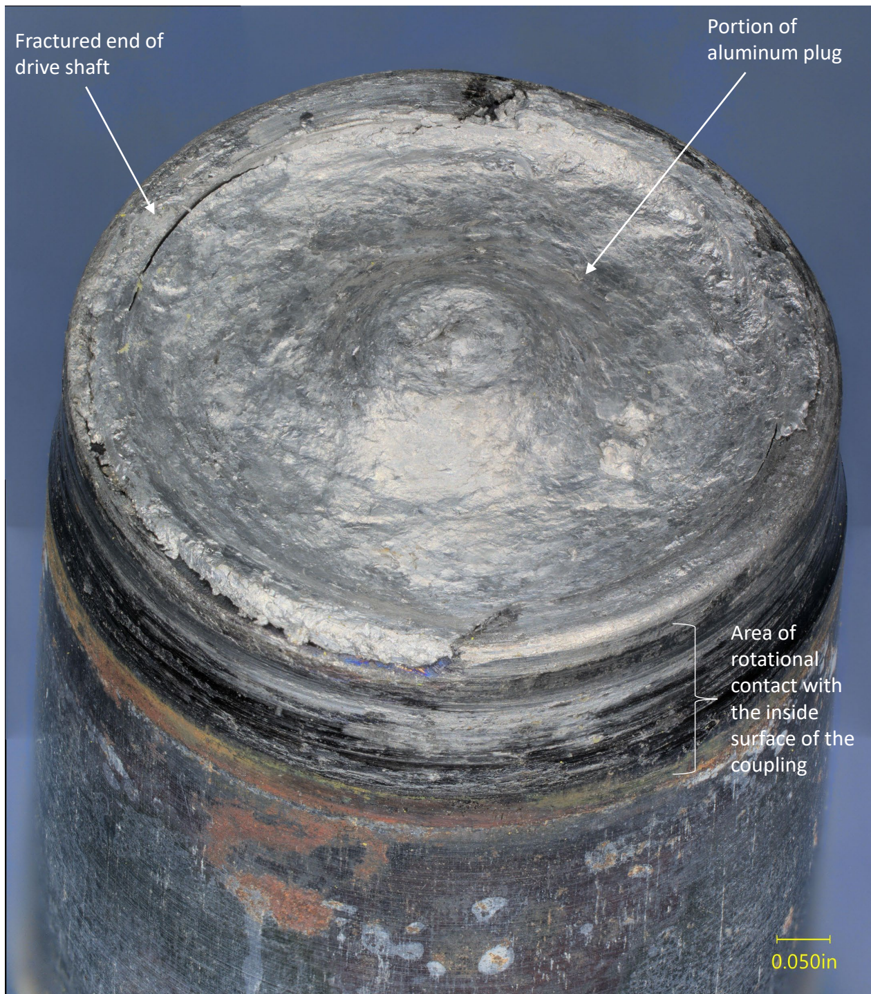
Figure 11 Oblique view of the fractured end of the as-received drive shaft tube showing rotational contact damage on the outside diameter of the drive shaft where it mates with the coupling.
