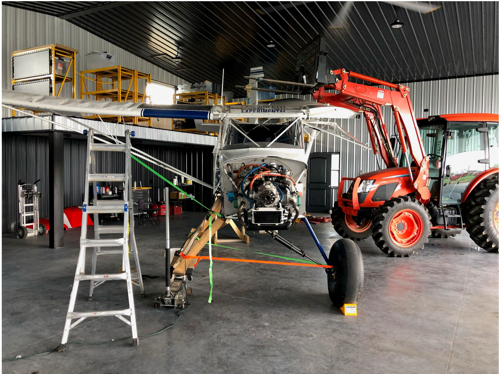
Photo 2 – View of Airplane Suspended from Sling During Testing (FAA)
