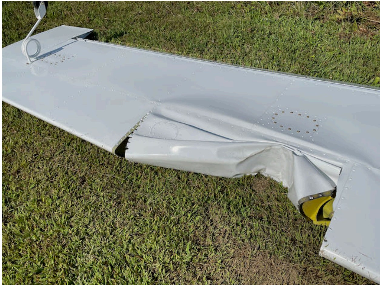
Photograph 1 – Accident glider – Left wing leading edge damage.
