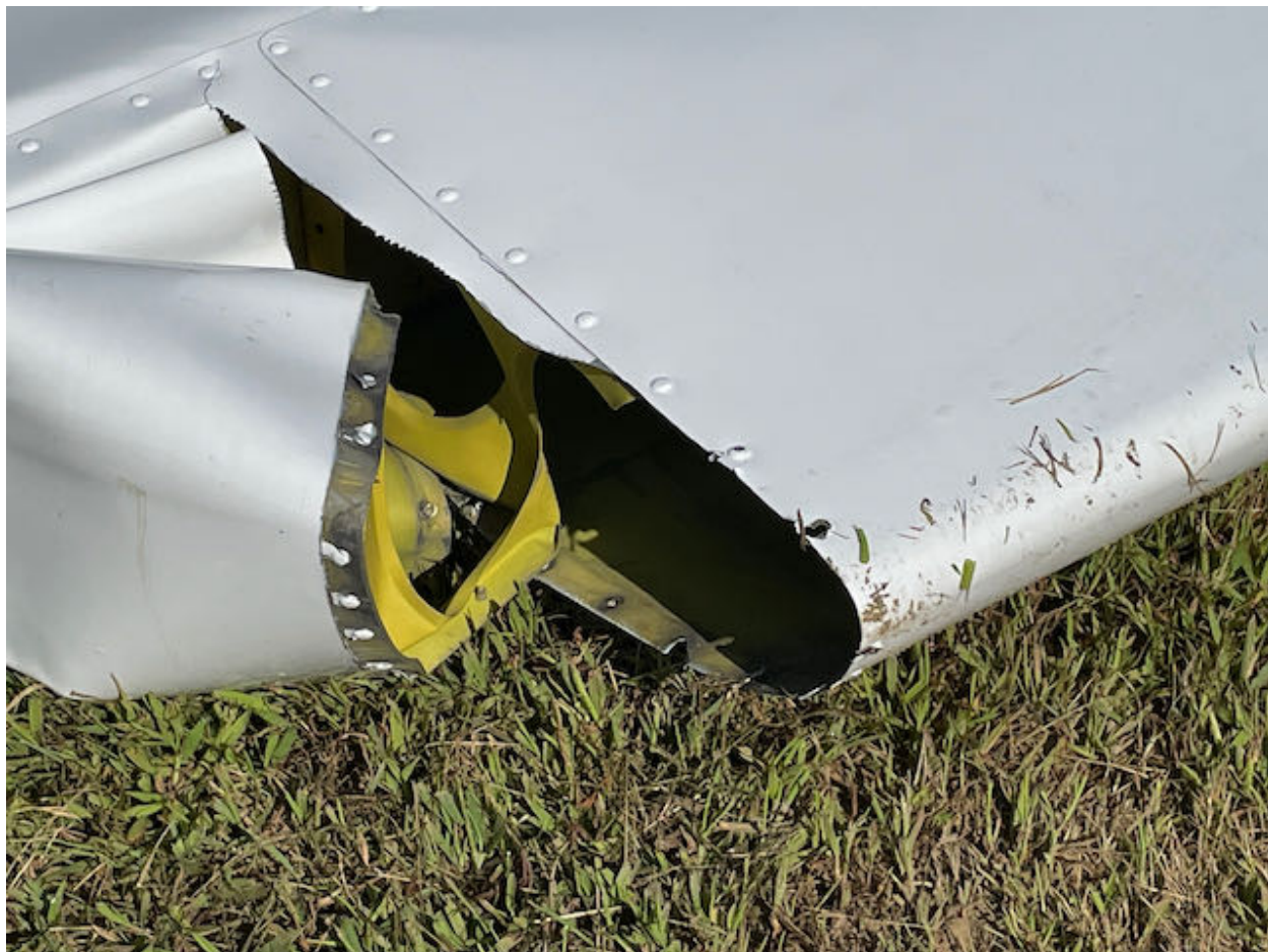
Photograph 3 – Accident glider – (Close-up) Left wing leading edge rib damage.
