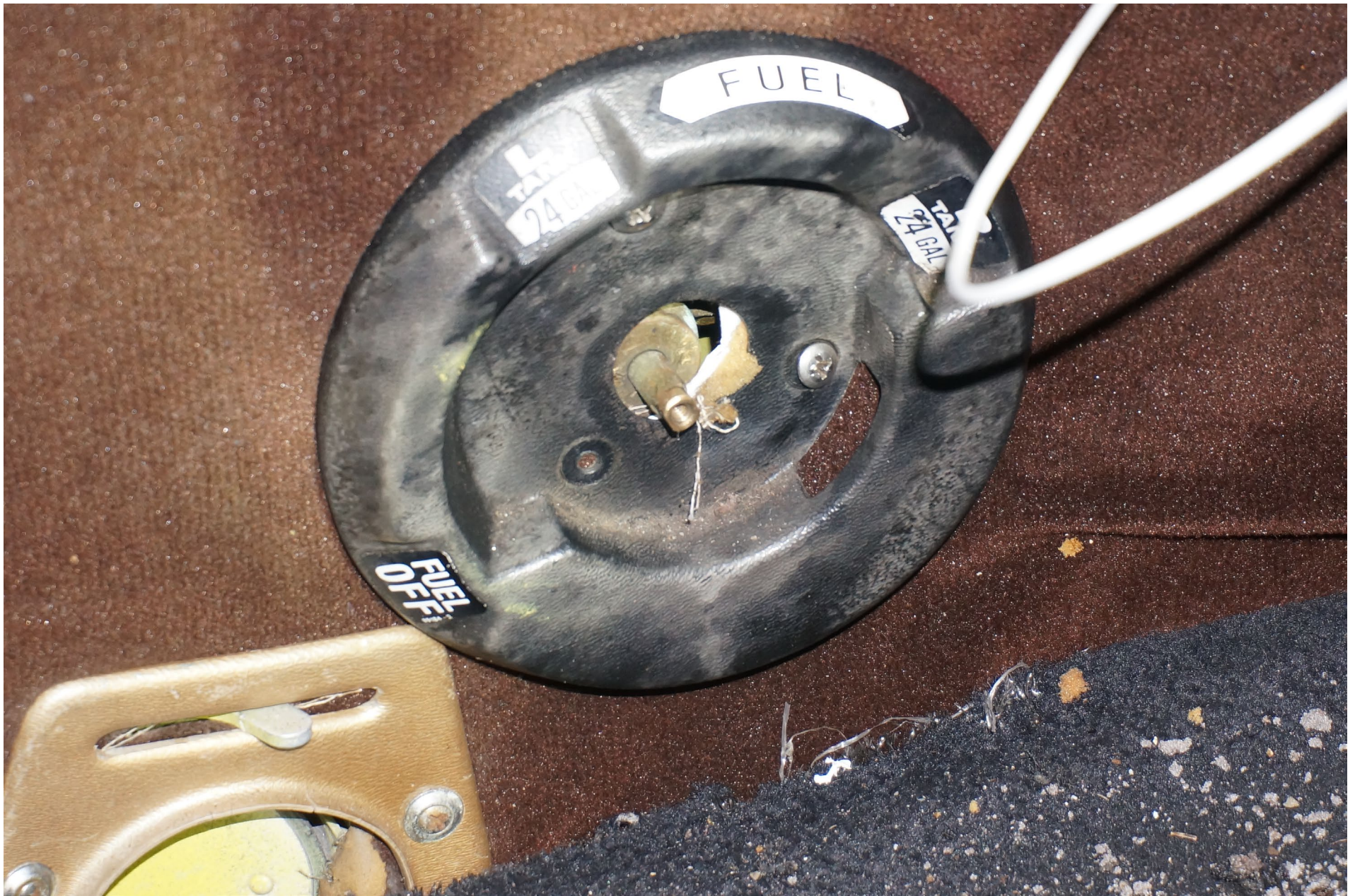
Photo 16 – Fuel Selector Valve Cover Mounted Off Center and not Clocked / Indexed
