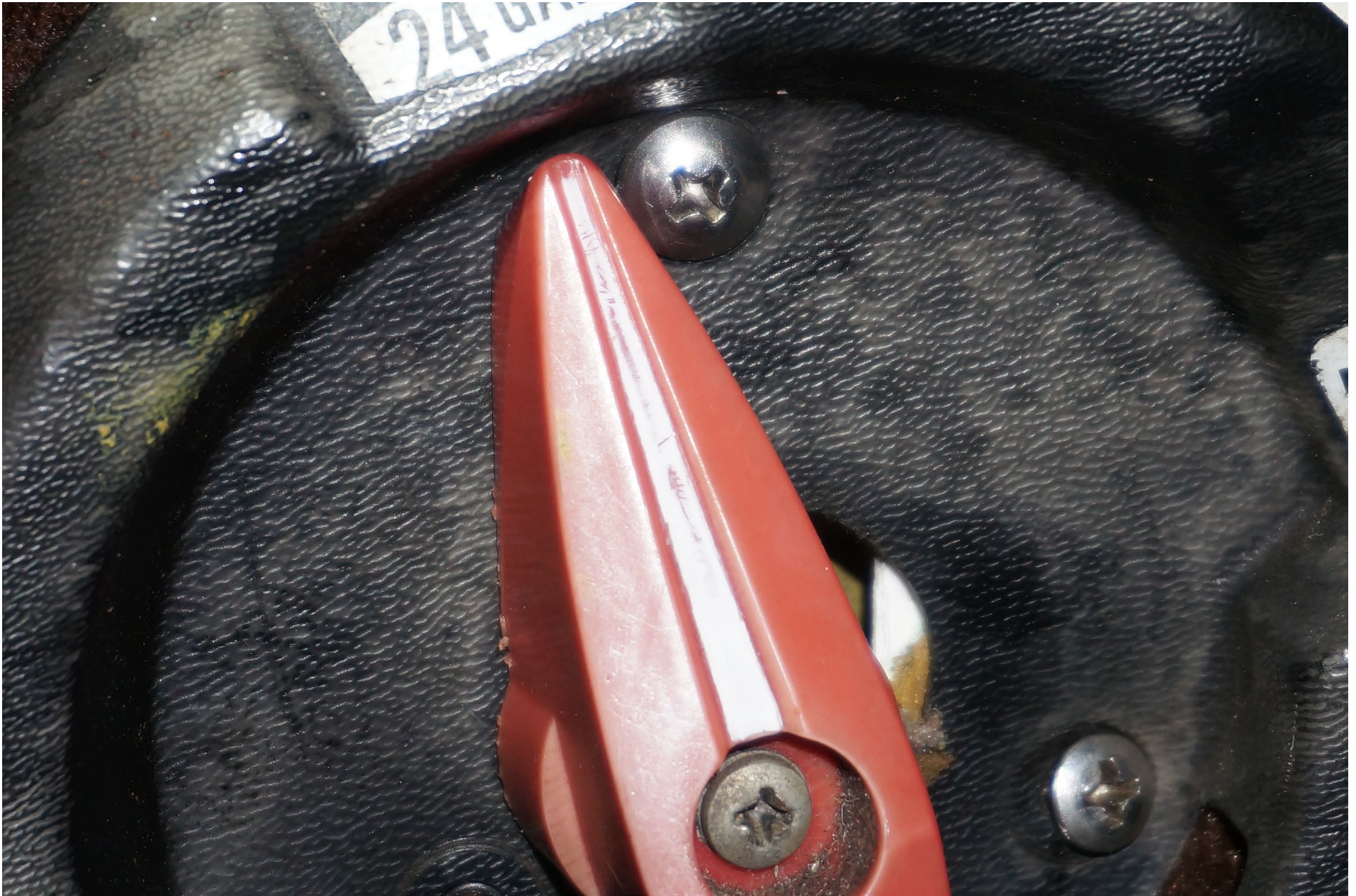
Photo 14 – Screw Interfering with Fuel Selector Handle
