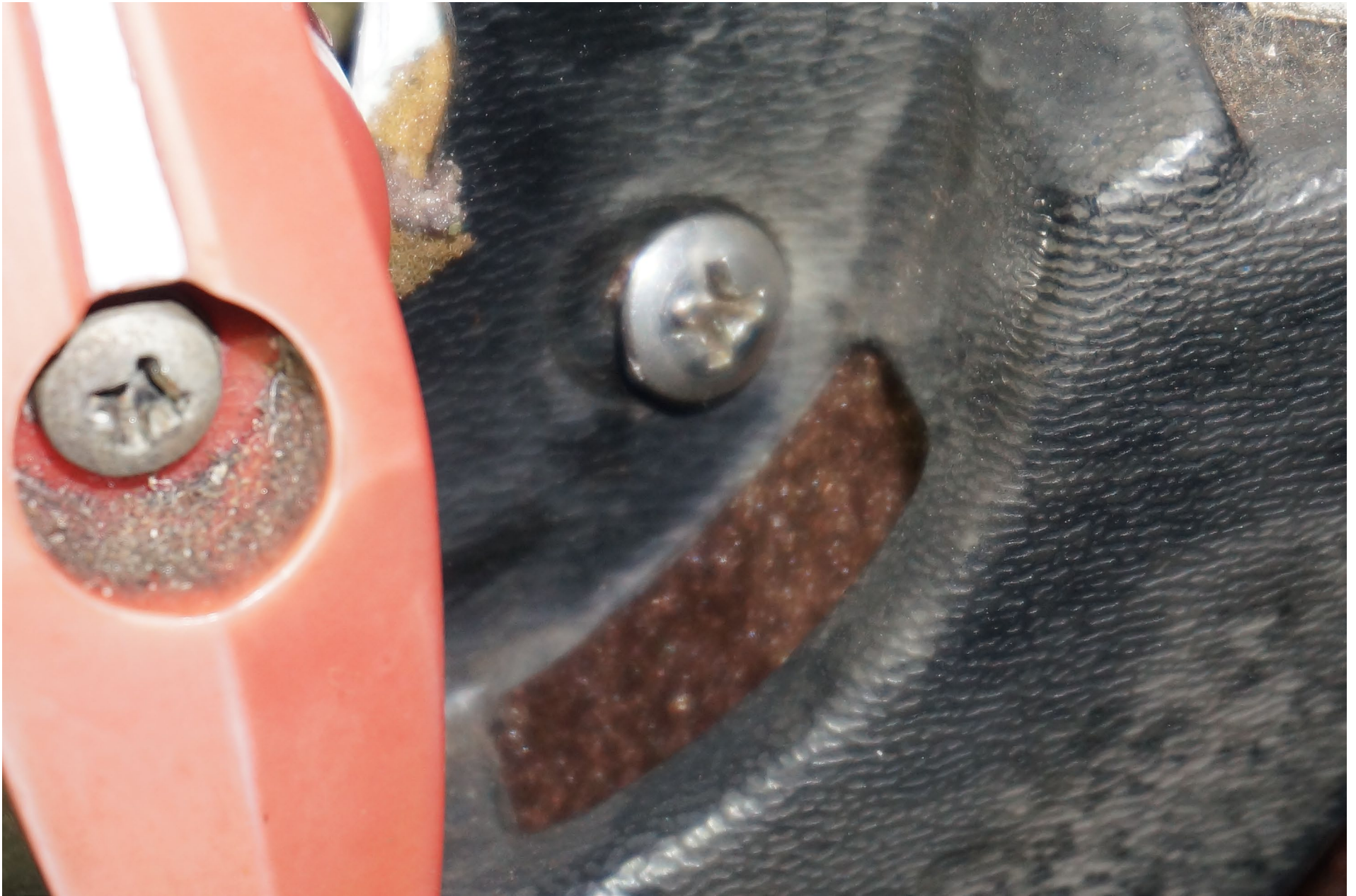
Photo 15 – Missing Spring Loaded Metal Stop
