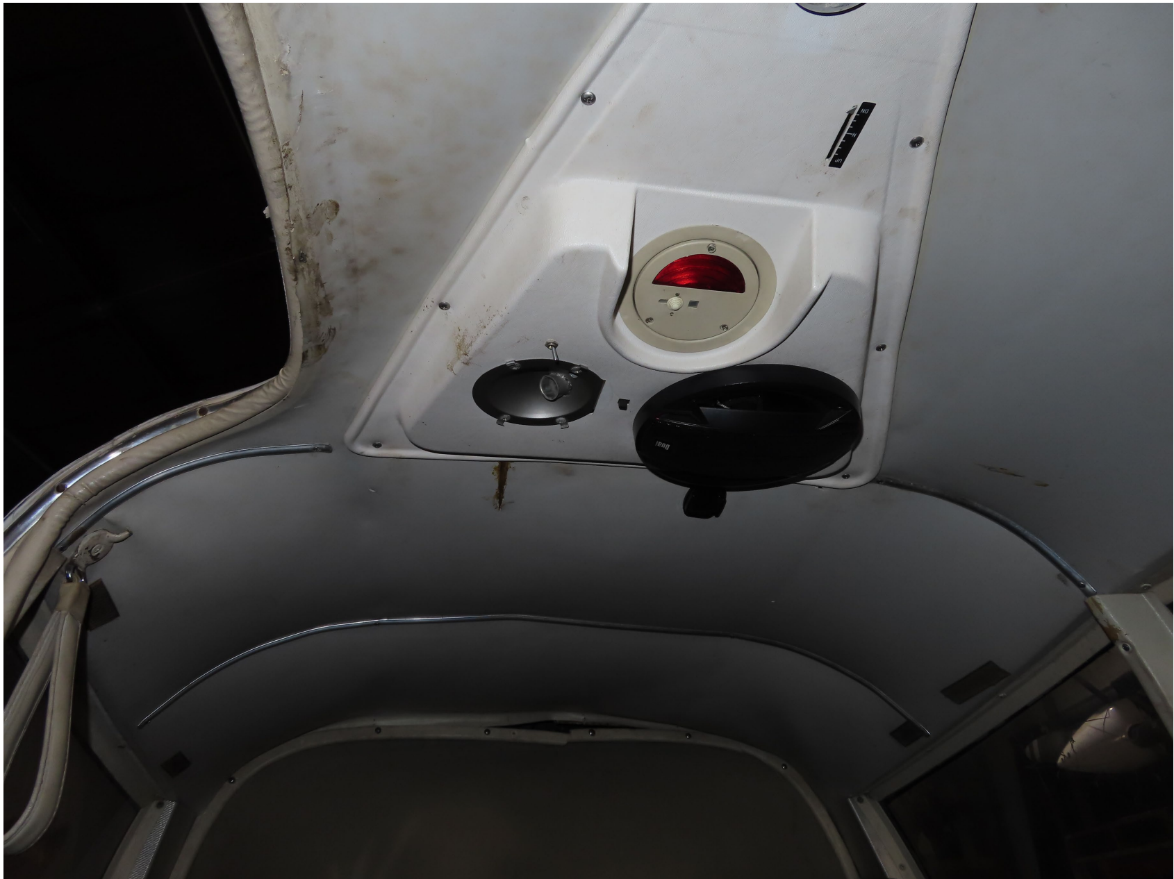
Photo 7 – Missing Light and Lense – Courtesy of Piper Aircraft
