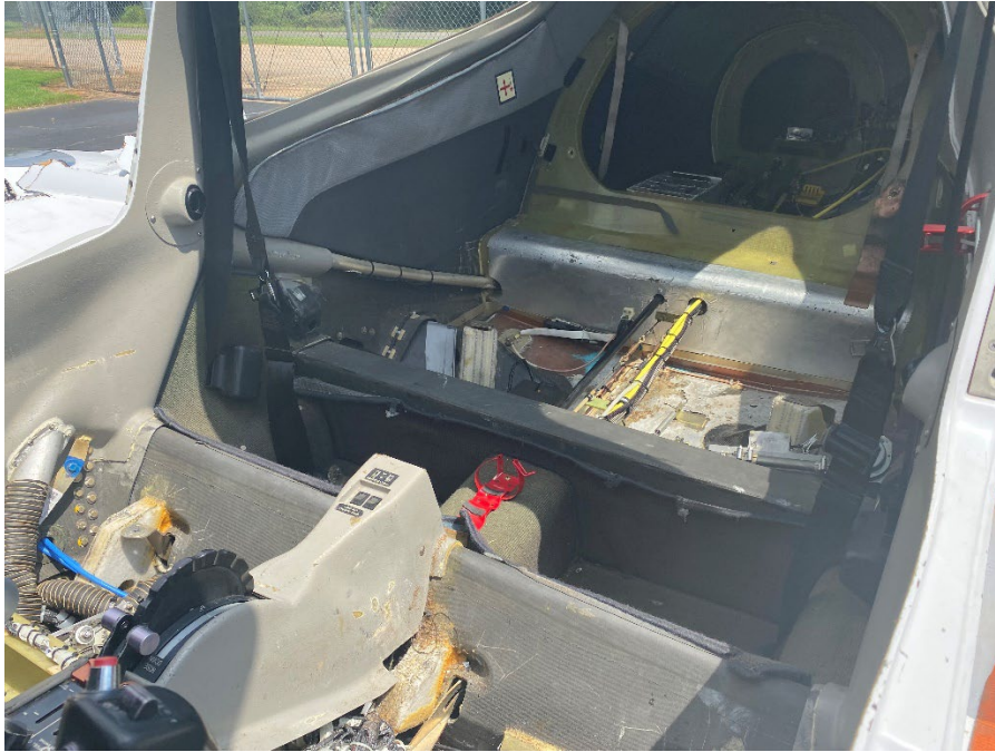
Figure 4: View of the elevator control linkages
