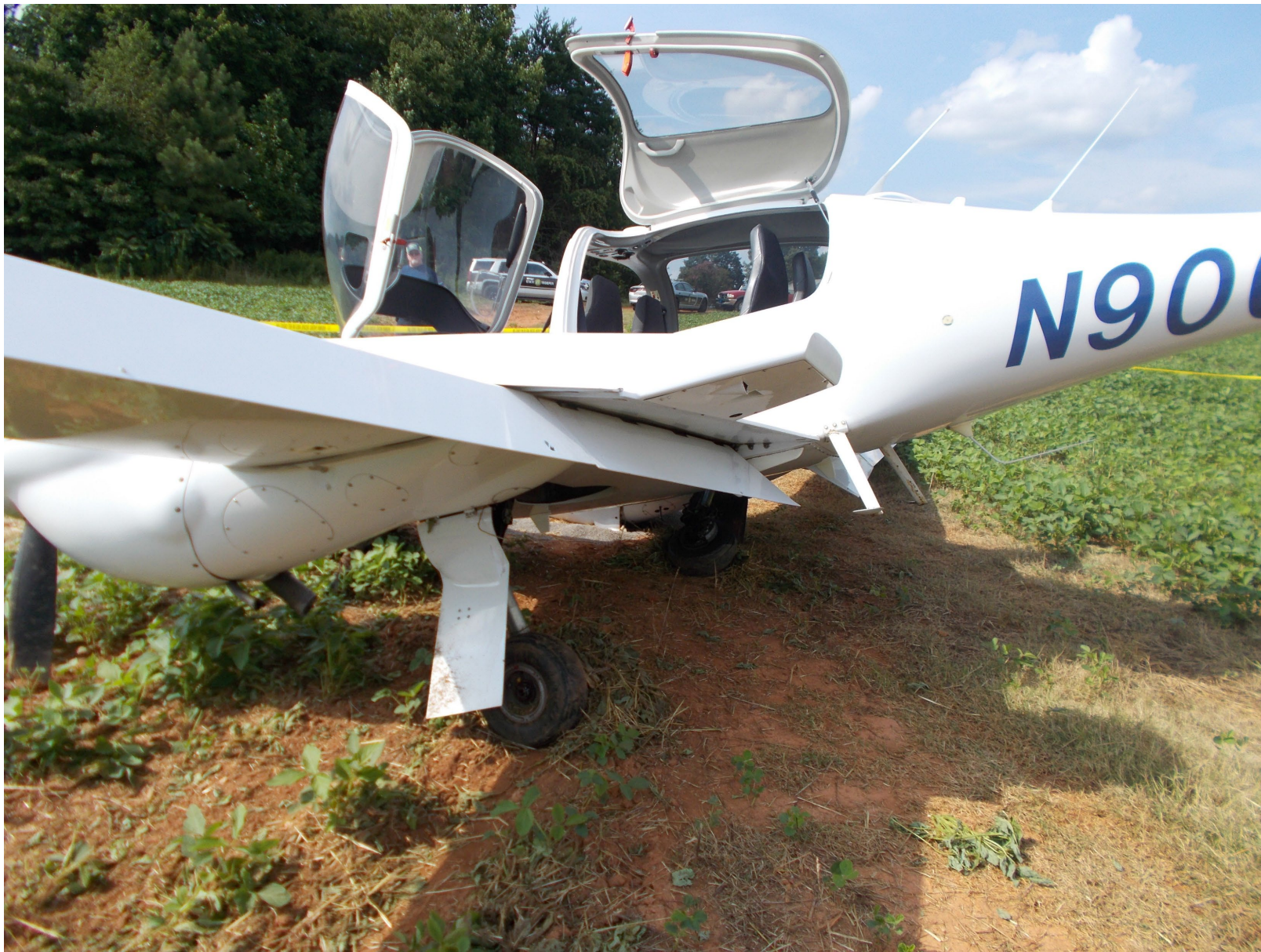
Photo 3 – View of the accident airplane’s left wing, flaps, and landing gear (Photo Courtesy of FAA)
