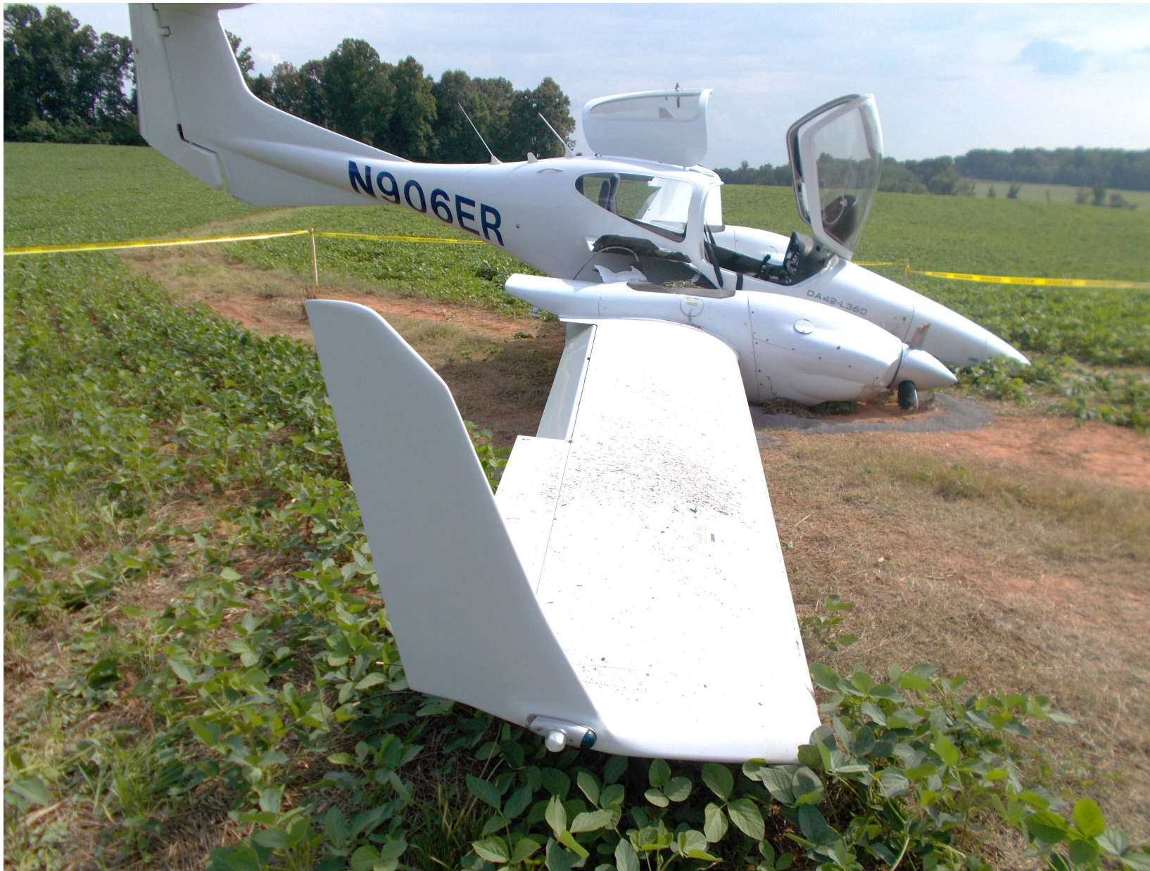
Photo 4 – View of the accident airplane's right wing (Photo Courtesy of FAA)
