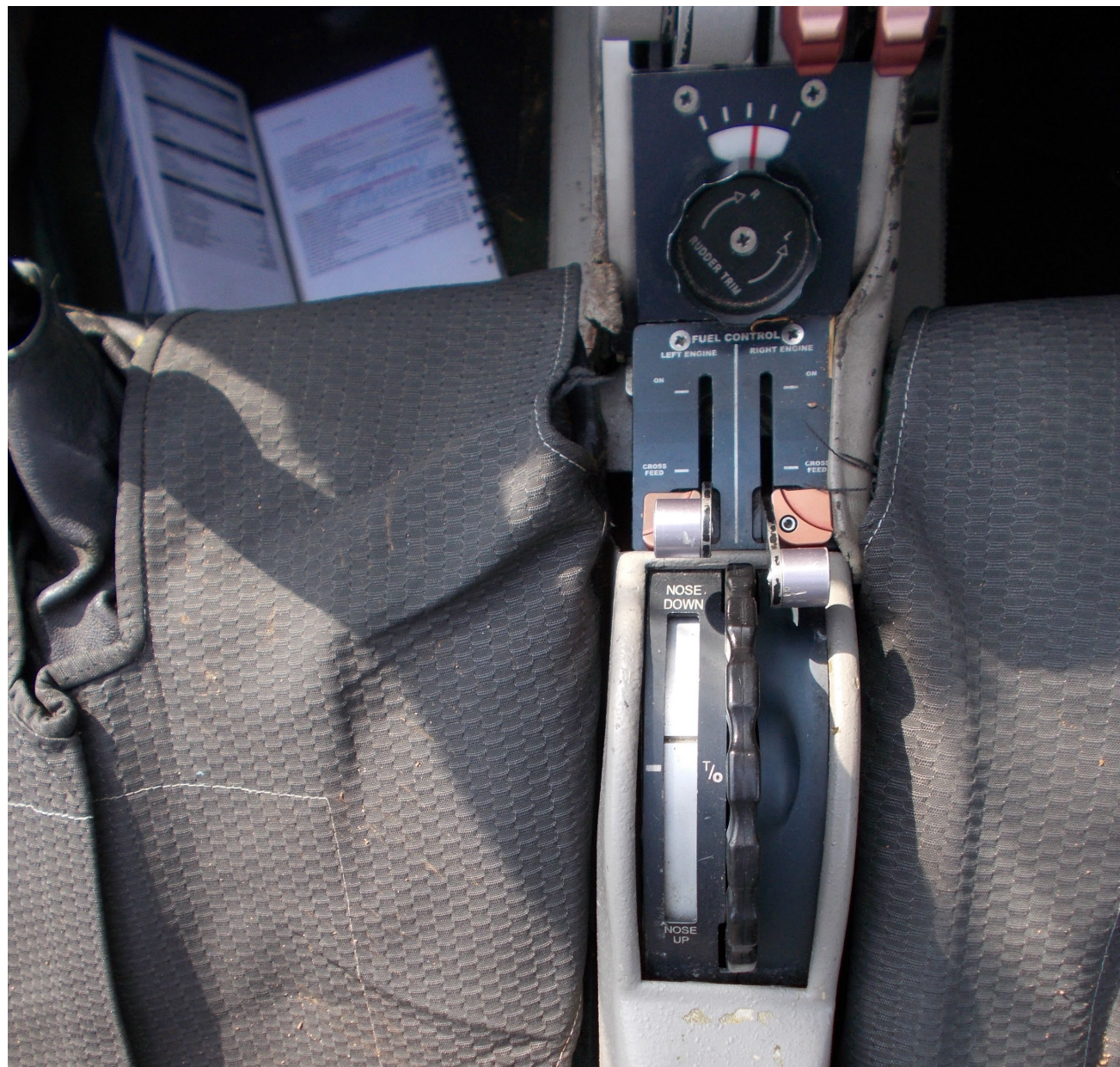
Photo 9 – View of the accident airplane's manual elevator trim and checklist located on floor (Photo Courtesy of FAA)
