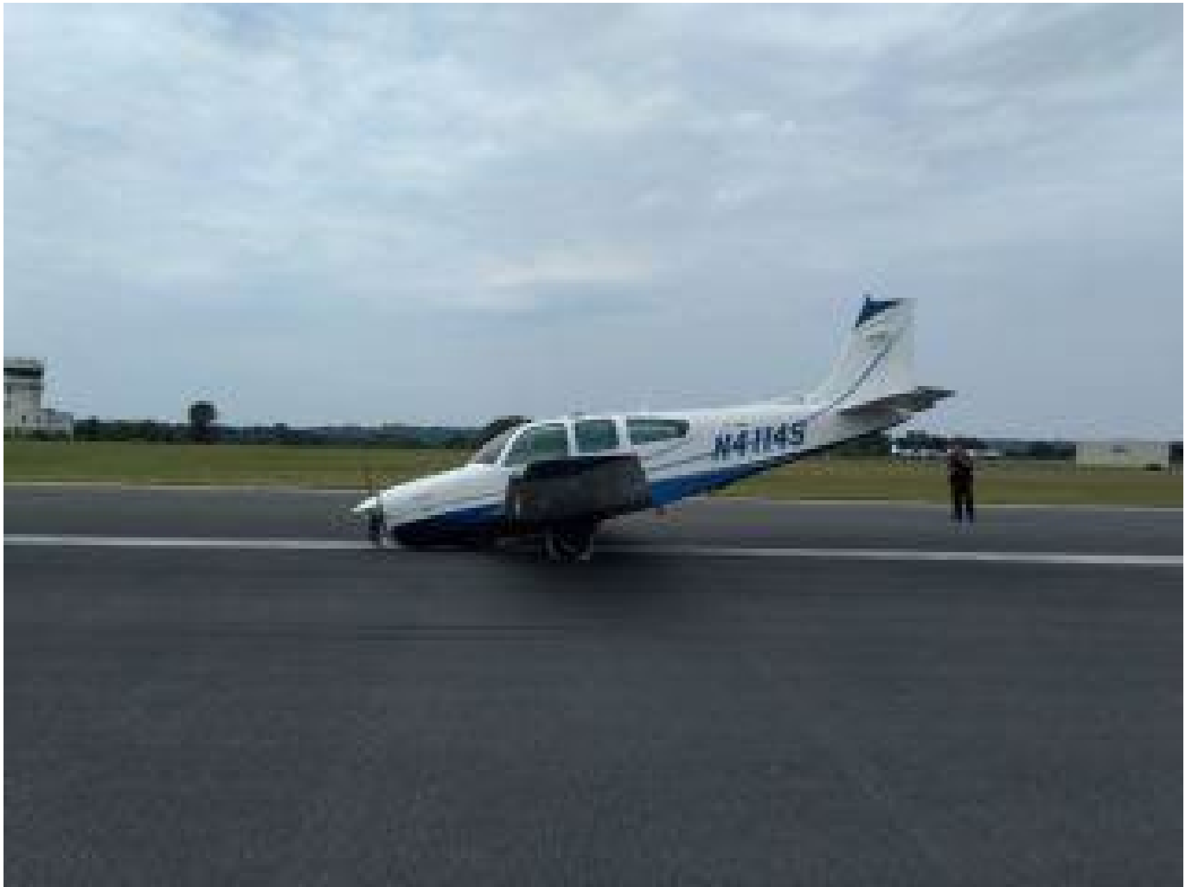
Photo 1 – View of airplane on runway with main gear partially collapsed and nose gear retracted. (FAA Photo)
