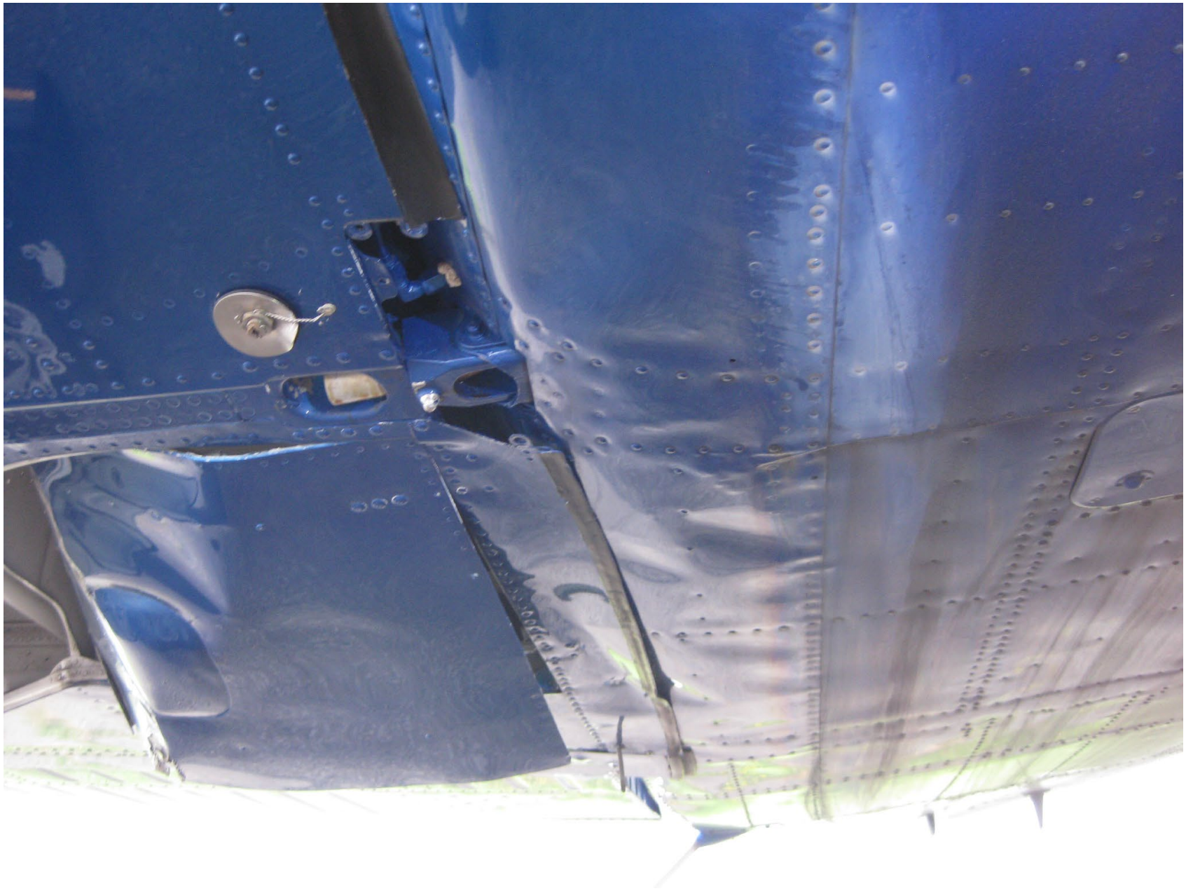
Photo 2 – View of underside of fuselage buckling. (FAA Photo)
