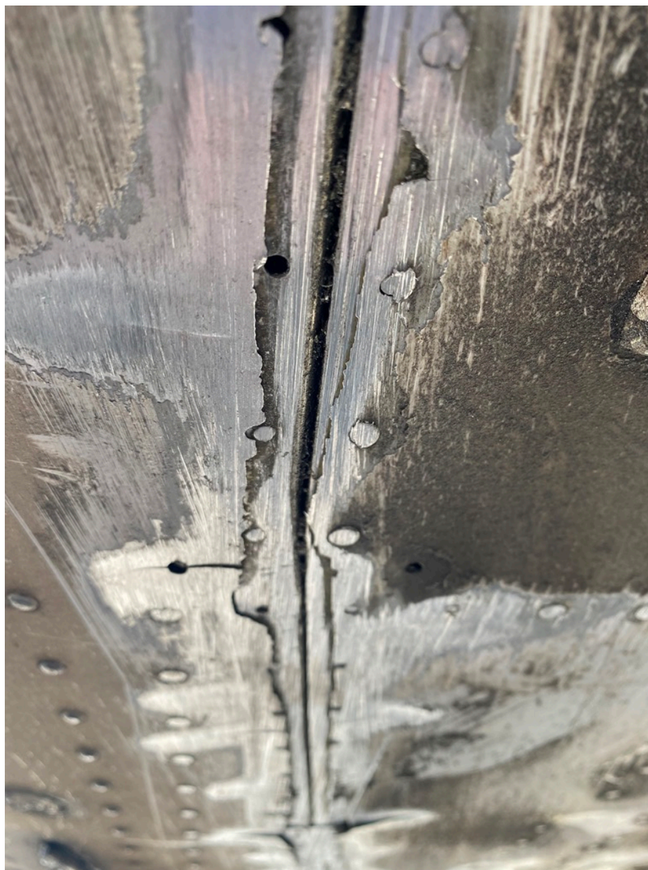
Photo 3 - Damage to lower fuselage (courtesy FAA)
