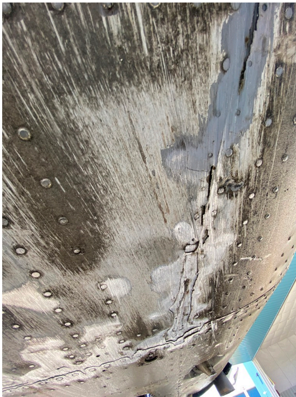
Photo 2 – Damage to lower fuselage (courtesy FAA)
