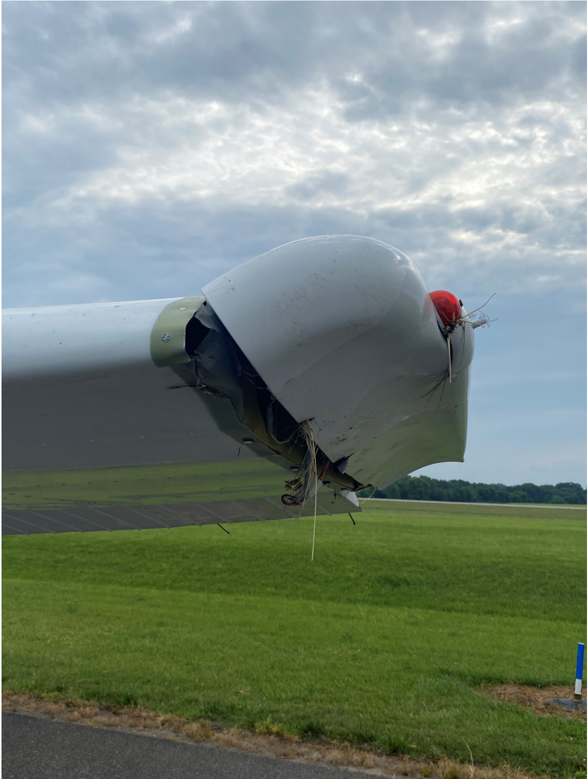
Photograph 5 – Accident airplane – Left wing damage.
