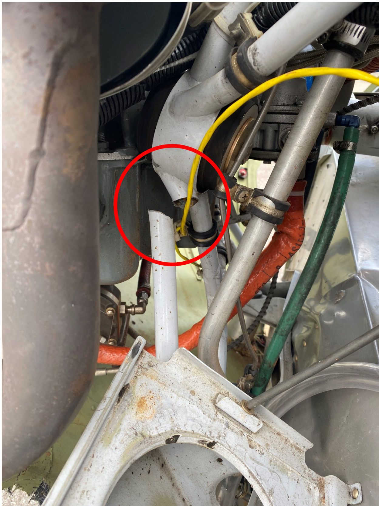
Photograph 6 – Accident airplane – Broken motor mount.
