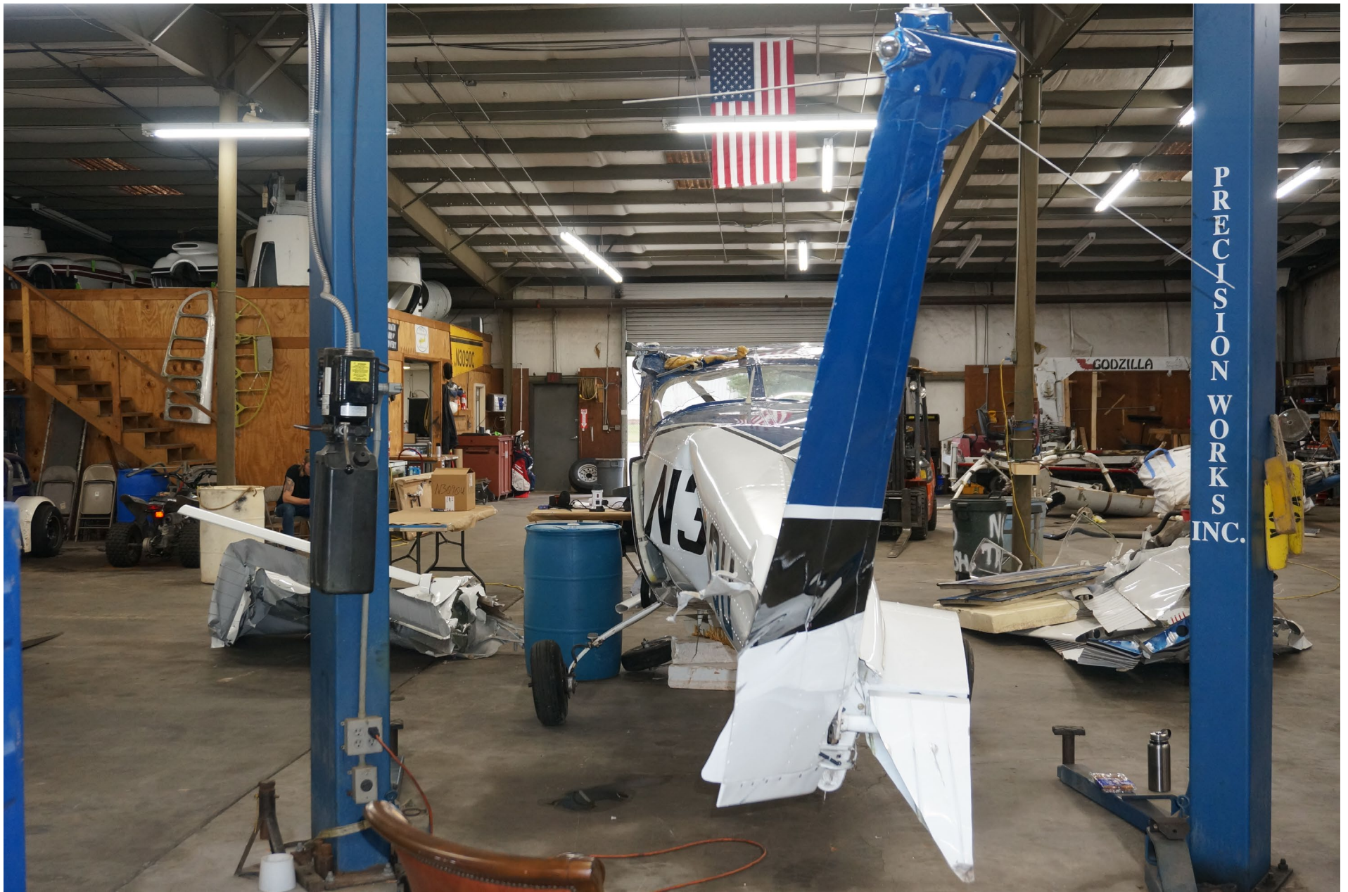
Photo 11 – Rear View of Main Wreckage
