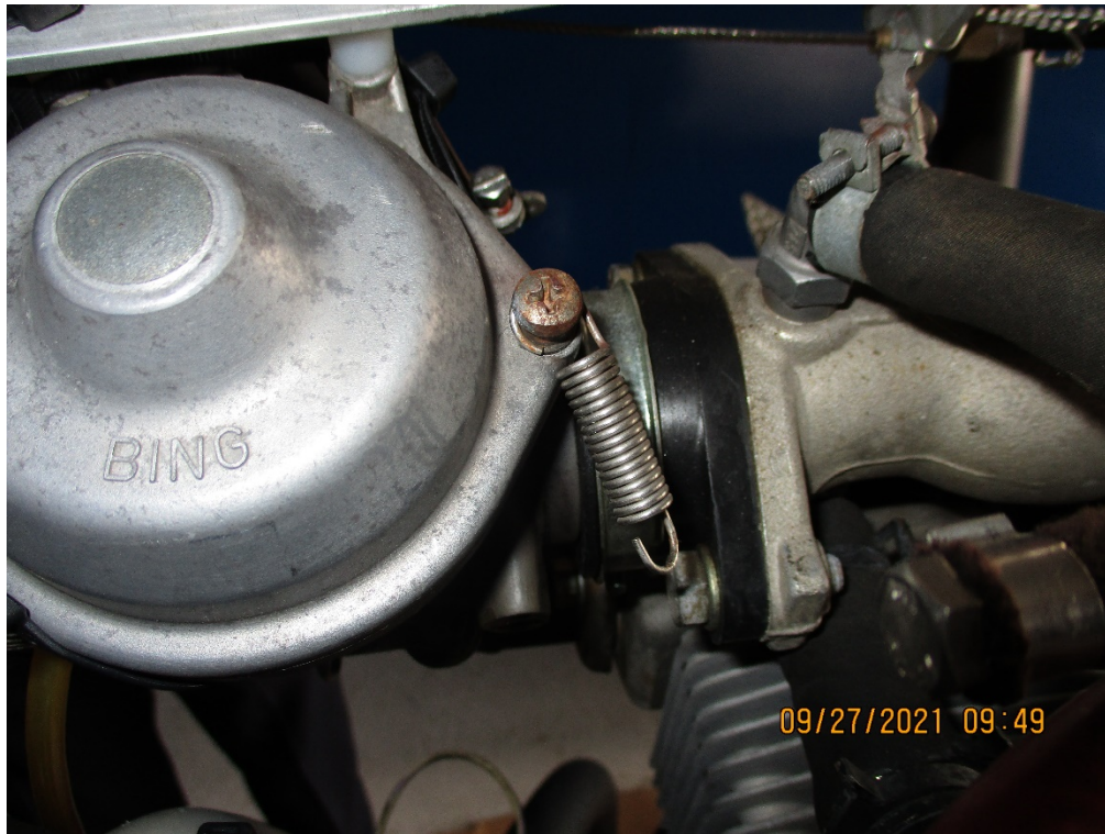
Right side carburetor in its mount with anti-vibration spring not connected.
