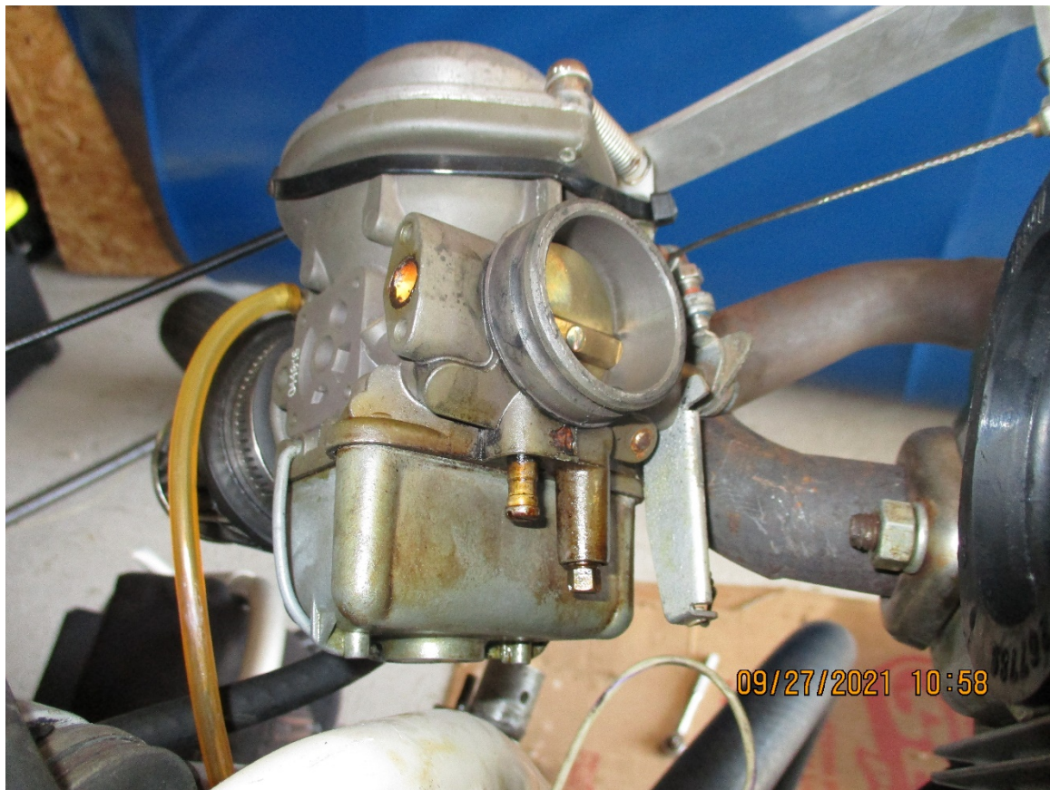
Right side carburetor out of mount, held up by throttle cable. Carburetor show no signs of any post-accident damage .
