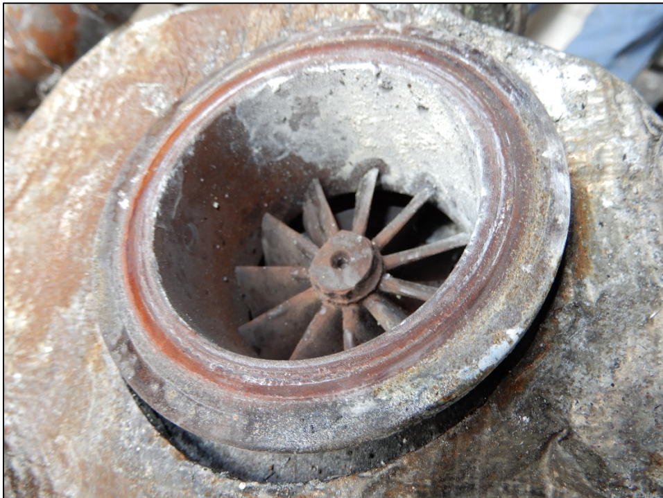
Photo 8: View of the turbo charger with fire debris removed from its outer area
