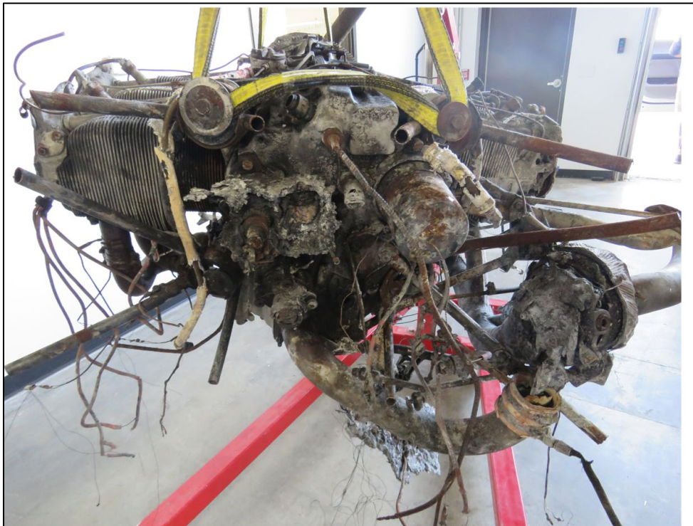
Photo 6: Accessory section of engine and view of damaged oil and fuel hose lines
