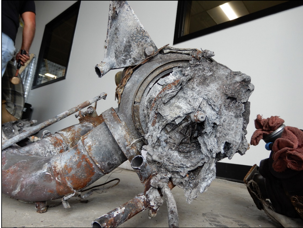
Photo 7: View of the turbo charger
