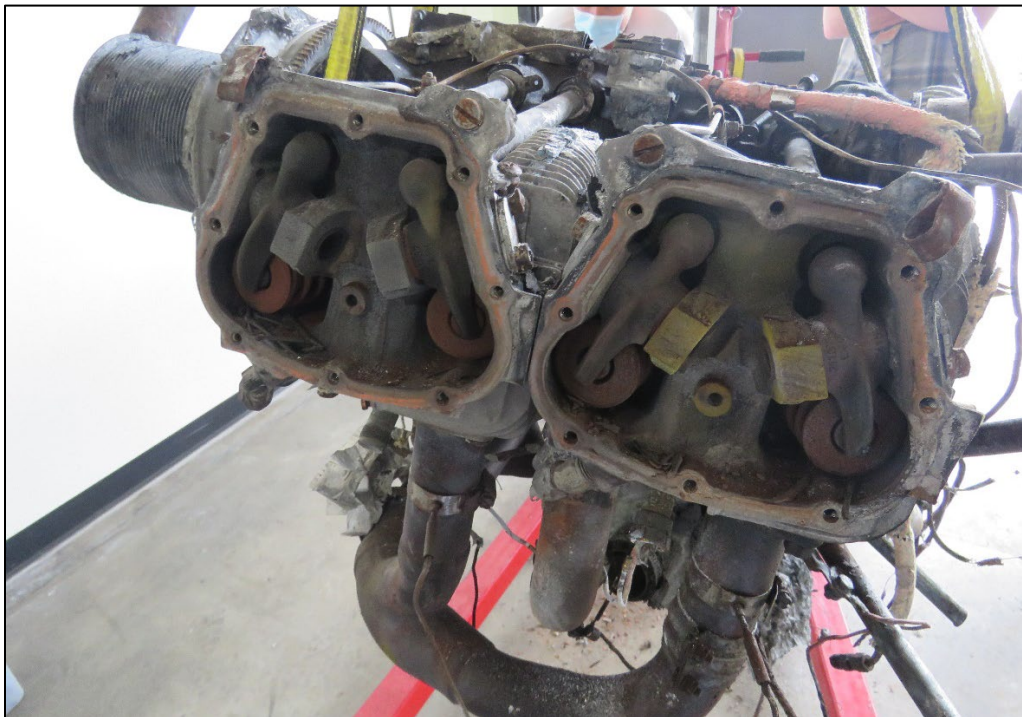
Photo 4: View of the cylinder valves
