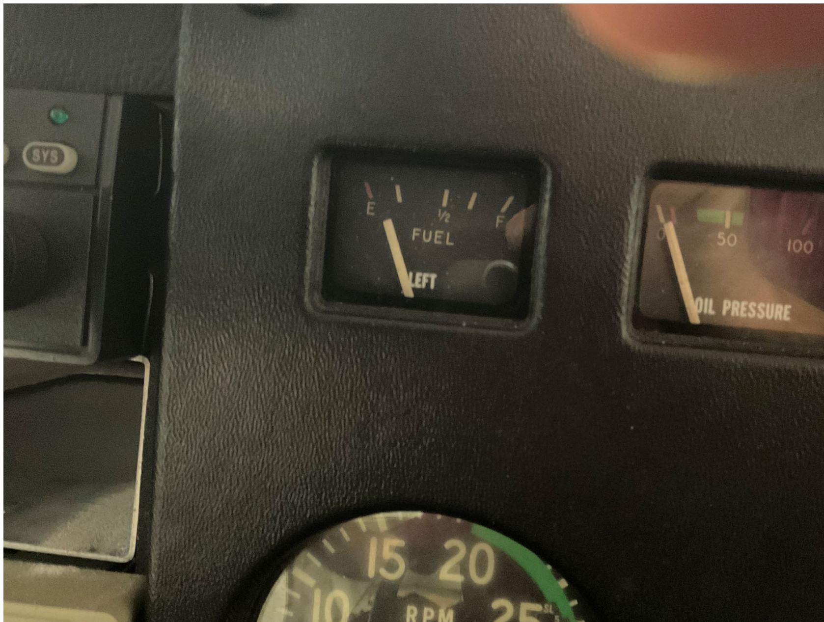
Photo 3 - FAA Digital Photograph. View of the Left Fuel Gauge with Electrical Power Applied and No Fuel in Left Fuel Tank. Note the Needle Slightly Above Empty.
