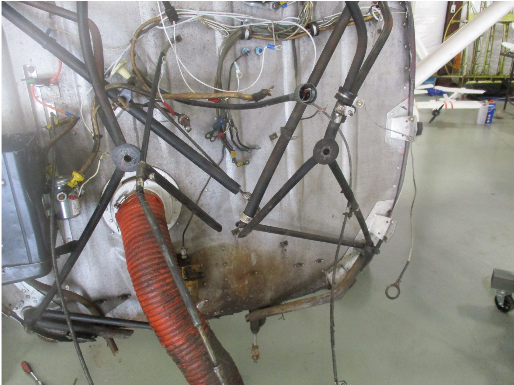
Photo 2 – FAA Digital Photograph. View of the Firewall and Damaged Engine Mount.
