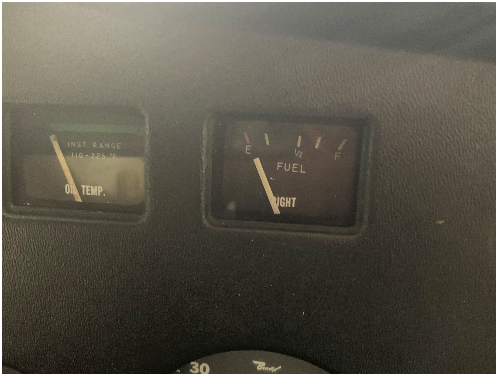
Photo 4 - FAA Digital Photograph. View of the Right Fuel Gauge with Electrical Power Applied and No Fuel in Right Fuel Tank. Note the Needle at Empty.
