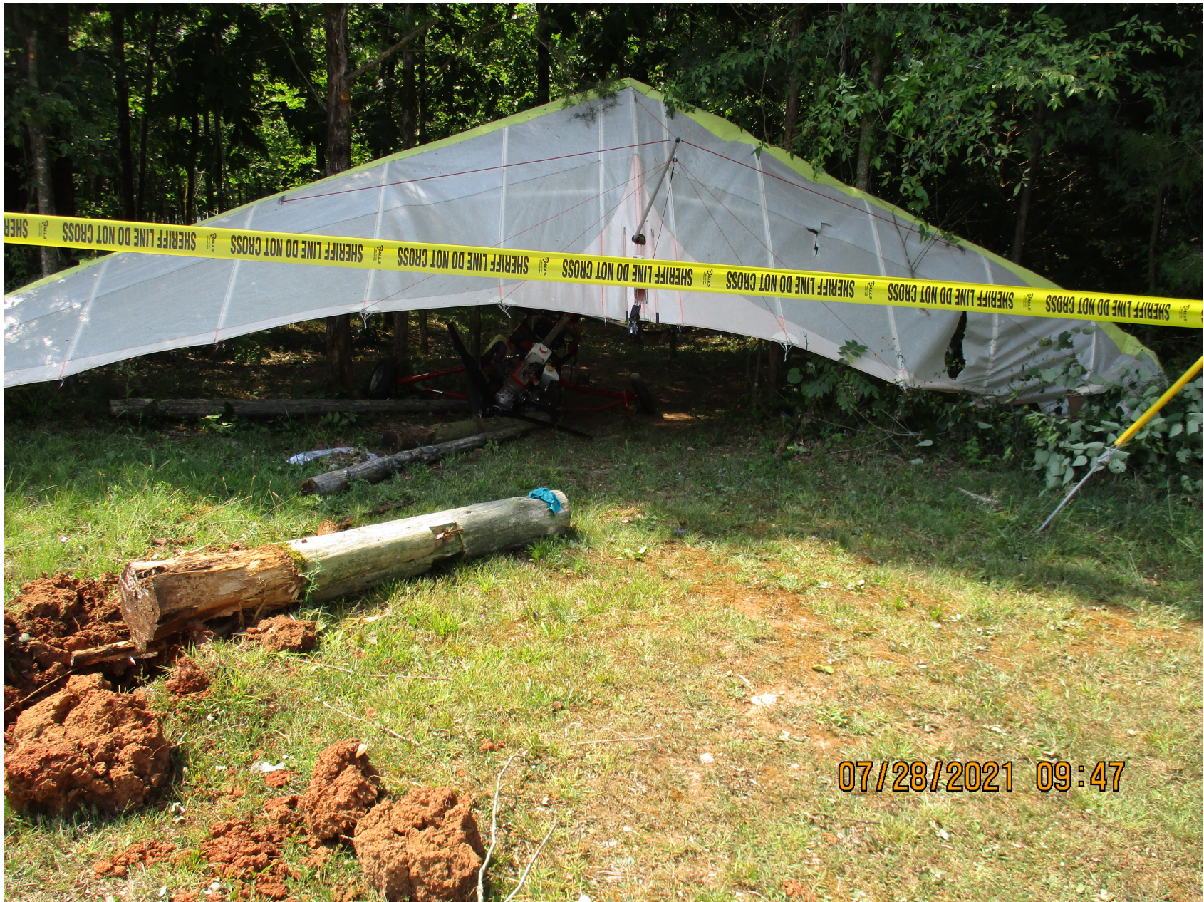
Photo 2 – View of weight-shift aircraft in tree line with fence post laying on the ground. Picture also shows structural damage to the right wing.
