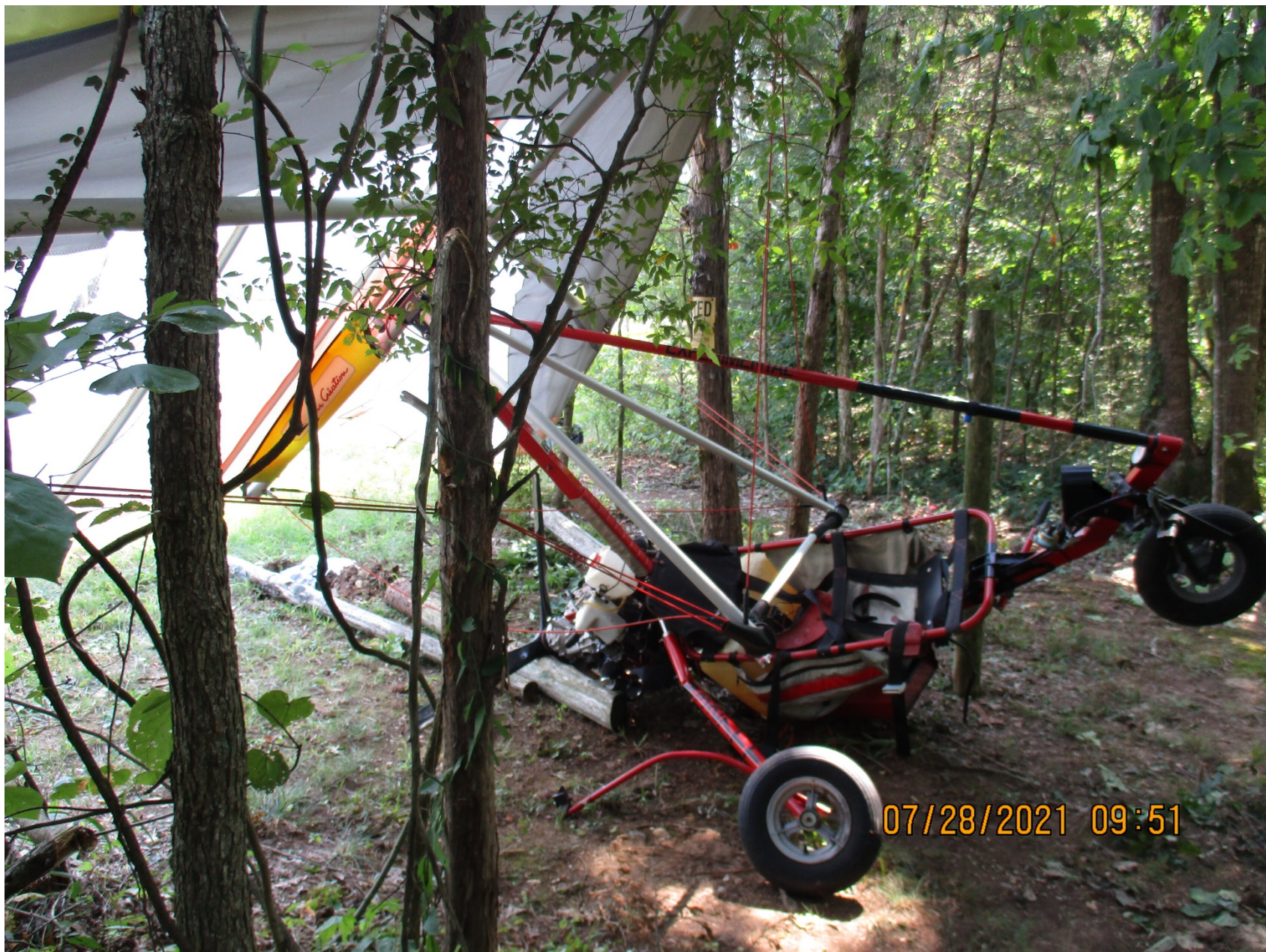
Photo 1 – View showing weight-shift aircraft in tree line. Also showing structural damage to the airframe.
