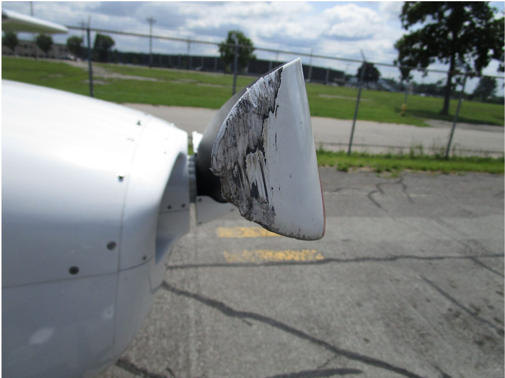
Photo 8 – Damage to 2nd Propeller Blade – Courtesy of FAA
