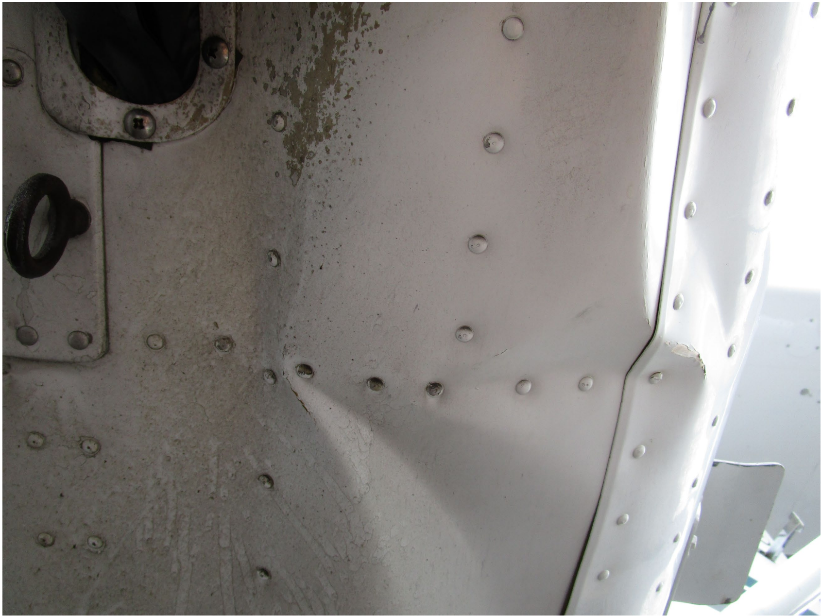
Photo 6 – Close Up Photograph of Buckling and Rivets (Bottom Forward Fuselage) – Courtesy of FAA
