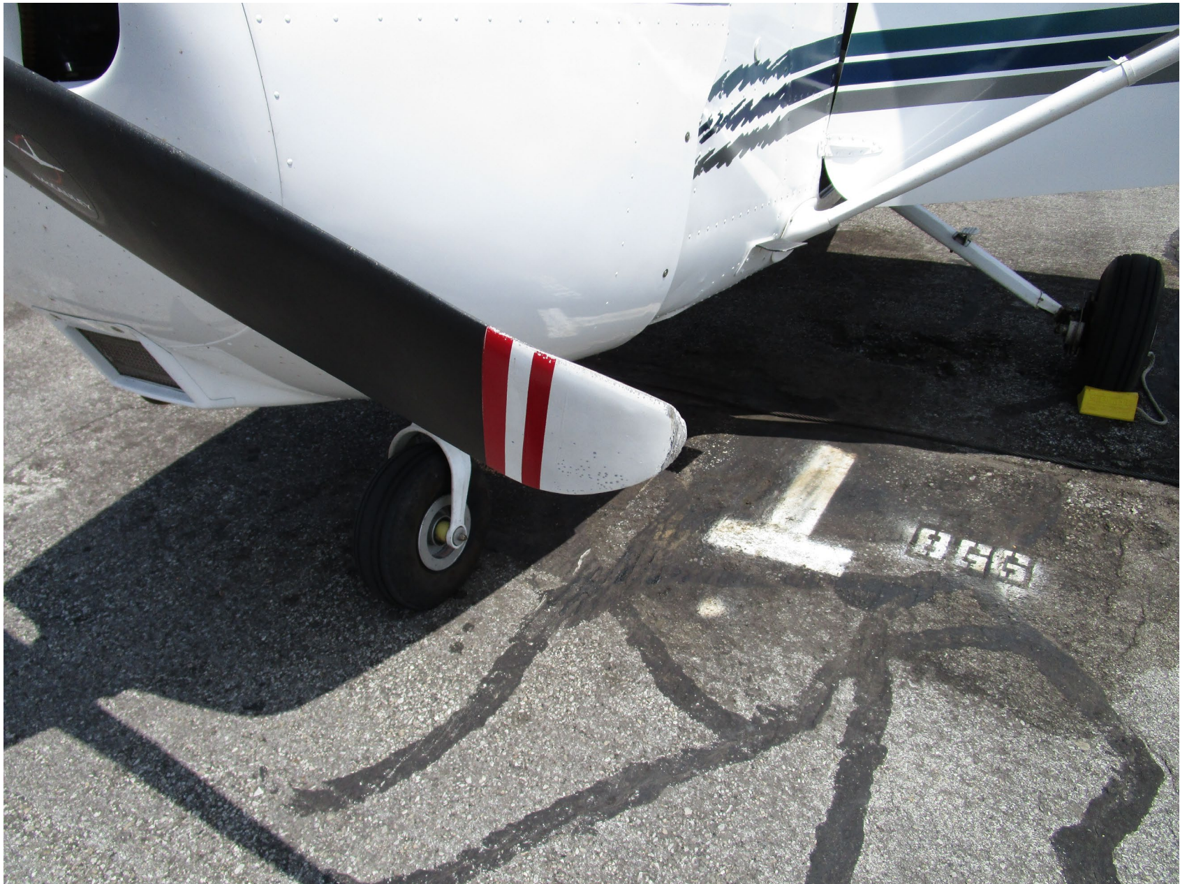
Photo 7 – Damage to 1st Propeller Blade – Courtesy of FAA
