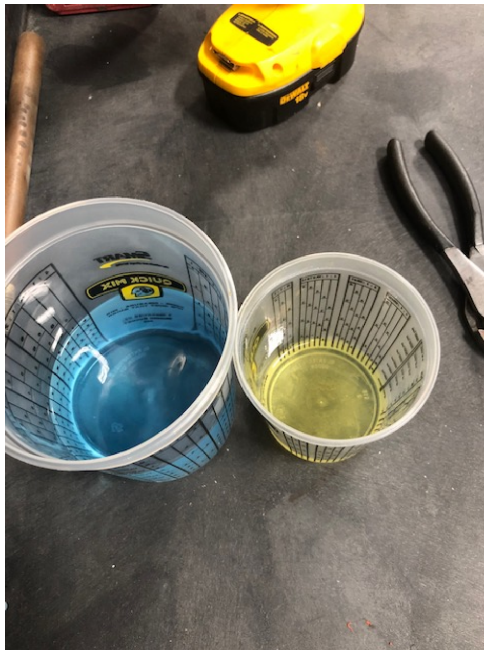
Photo 3 – View of Auto Fuel Drained from Gascolator (Right) and of Aviation Gasoline Used for Post-Accident Test Run (Precision Aviation)
