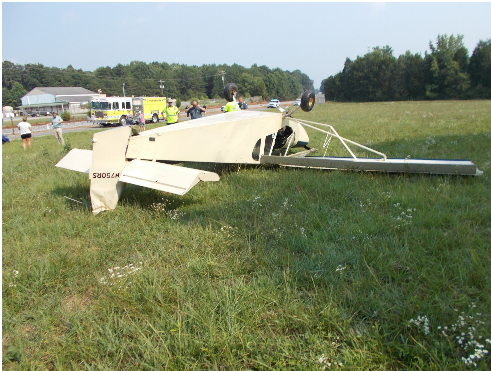
Photo 2 – View of Damage to Rudder/Vertical Stabilizer (FAA)
