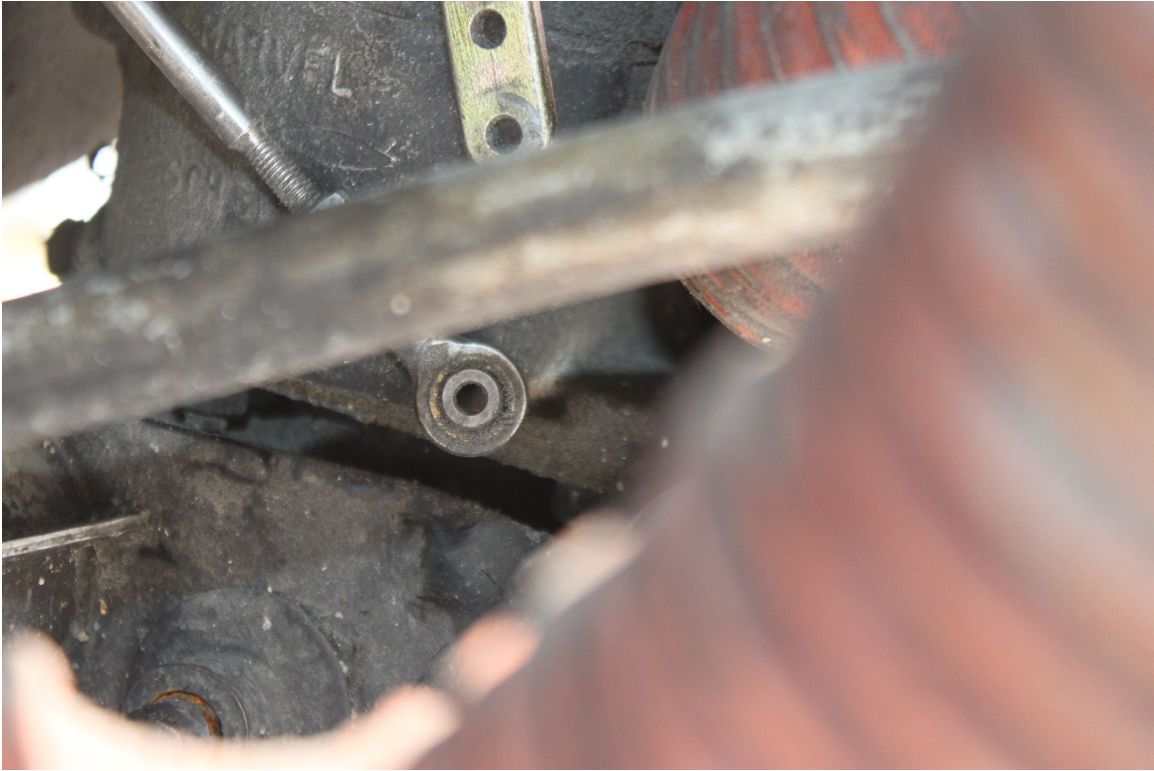
Figure 2: NTSB Digital Photograph. Close-Up View of the carburetor, intact throttle control lever, and separated but intact Throttle Control Cable.
