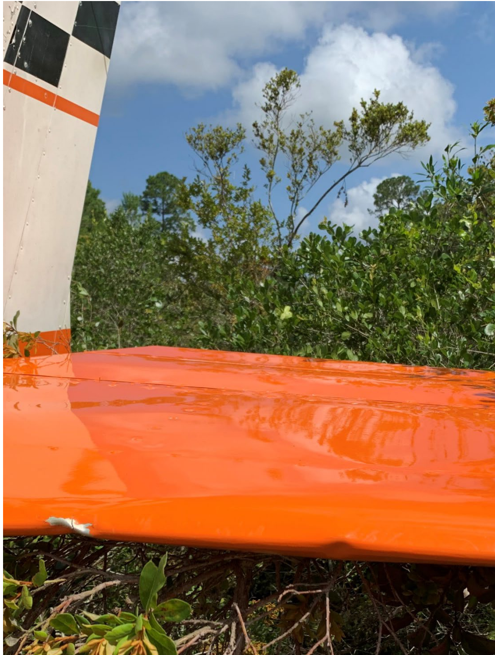
Photo 2 – View of the damage to the horizontal stabilizer. (Photo Courtesy of FAA)
