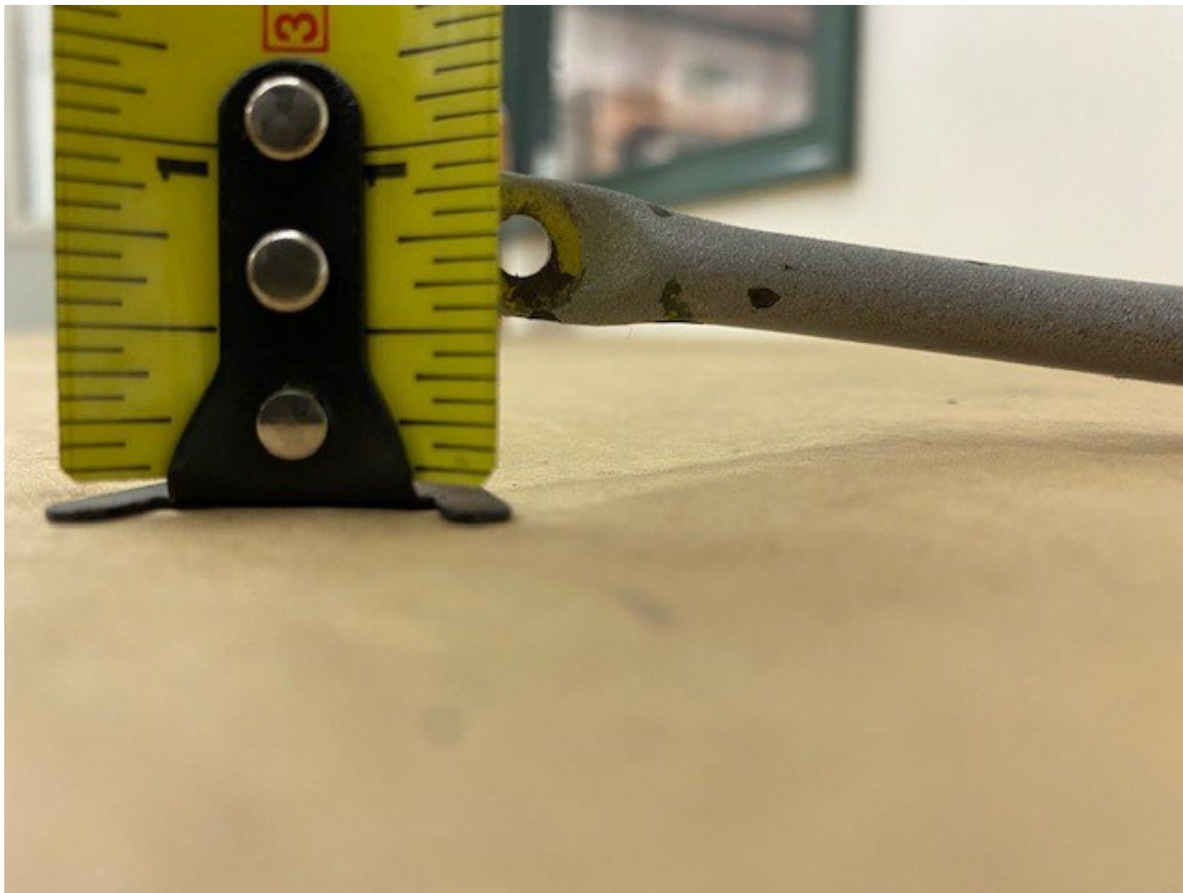
Photo 12 - FAA Digital Photograph. View of One End of the Right Front Seat Tube-Seat Catch Release. Note the Deformed Distance Above the Table About 0.5625 Inch.
