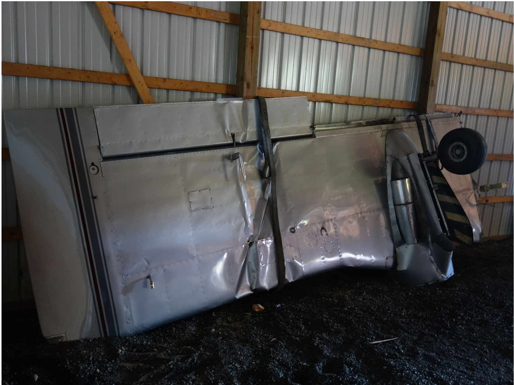
Photo 5 - Piper Digital Photograph. View of the Bottom Side of the Left Wing. Note the Structural Damage.
