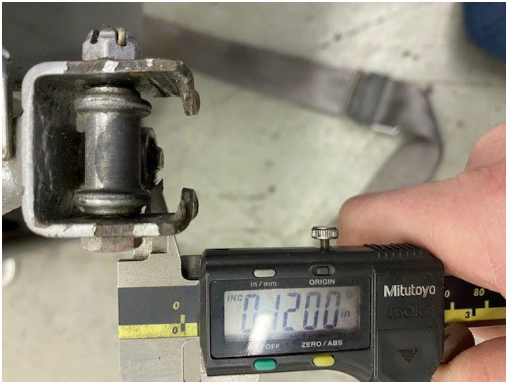
Photo 14 - FAA Digital Photograph. View of the Right Plunger-Seat Catch Extension of the Right Front Seat. Note the Extension of 0.1200 Inch From the Housing.
