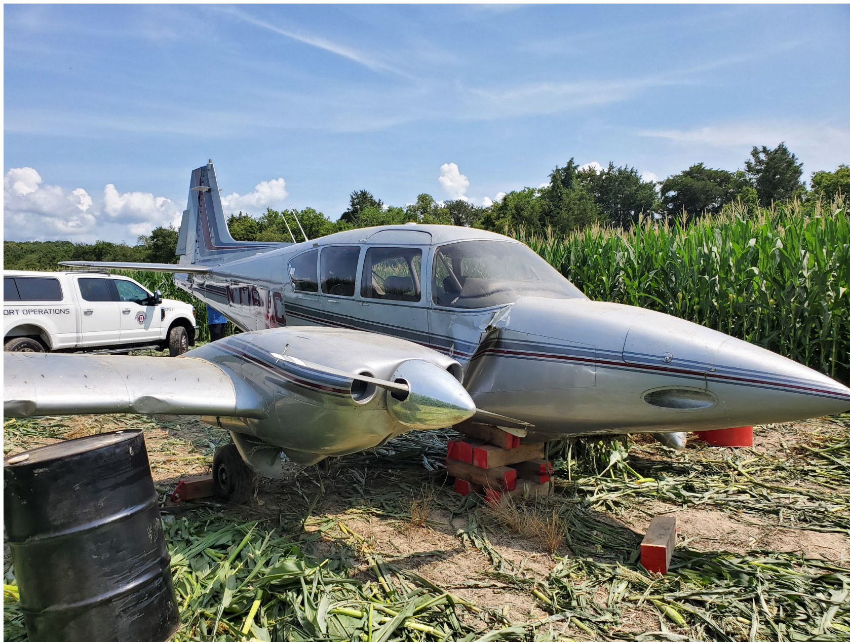
Photo 3 - FAA Digital Photograph. Right Front Quartering View of the Airplane at the Accident Site. Note the Right Fuselage Damage, and Feathered Right Propeller.
