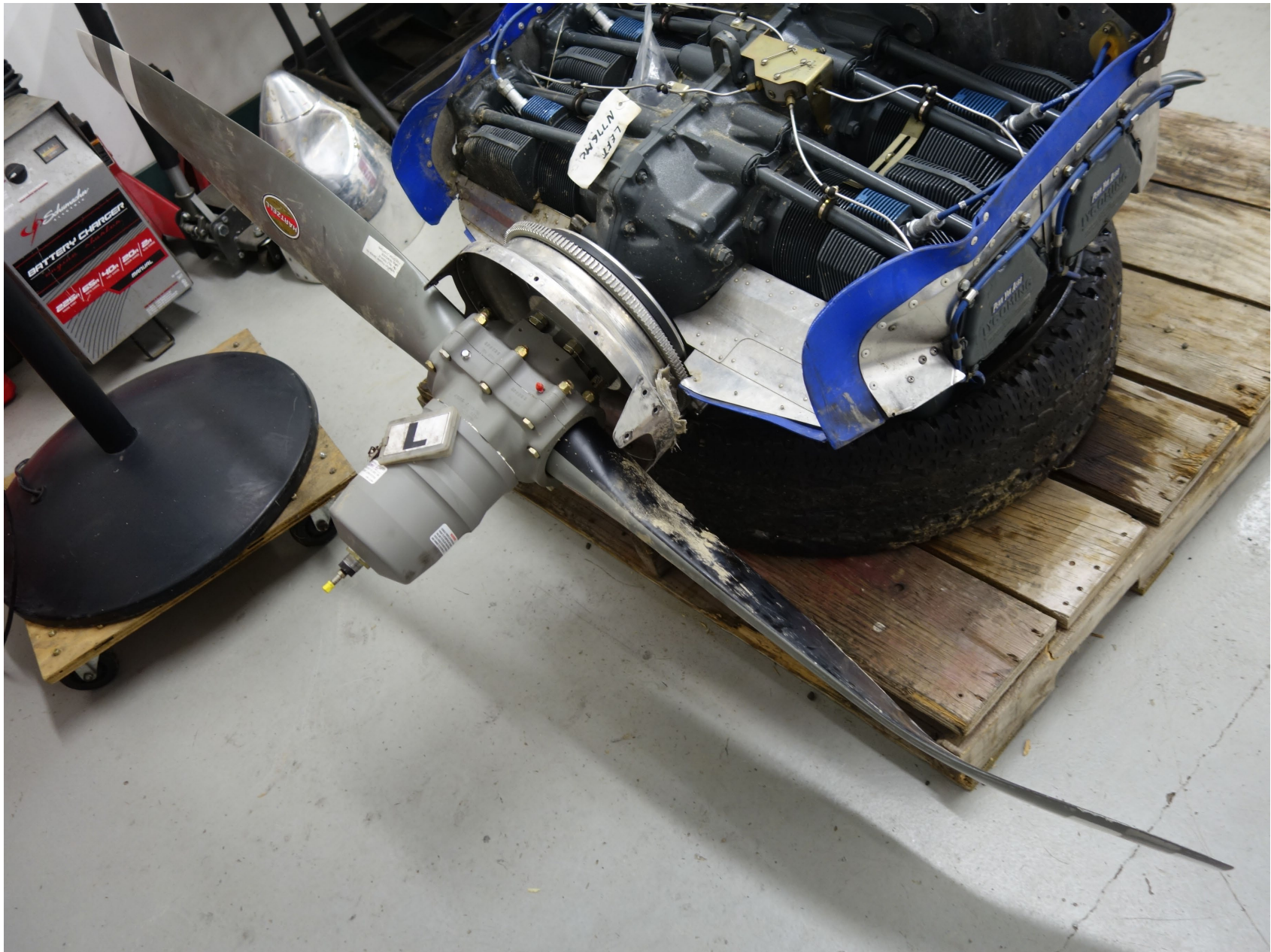
Photo 6 - Piper Digital Photograph. View of the Separated Left Engine And Propeller Assembly. Note the Slight Aft Bend of 1 Propeller Blade.
