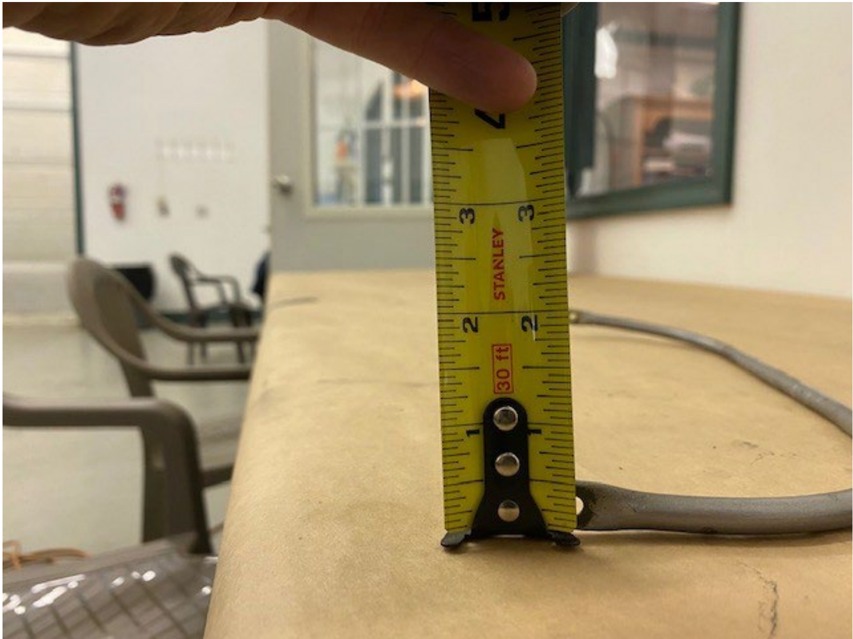
Photo 11 - FAA Digital Photograph. View of One End of the Right Front Seat Tube-Seat Catch Release. Note the Deformed Distance Above the Table About 0.125 Inch.
