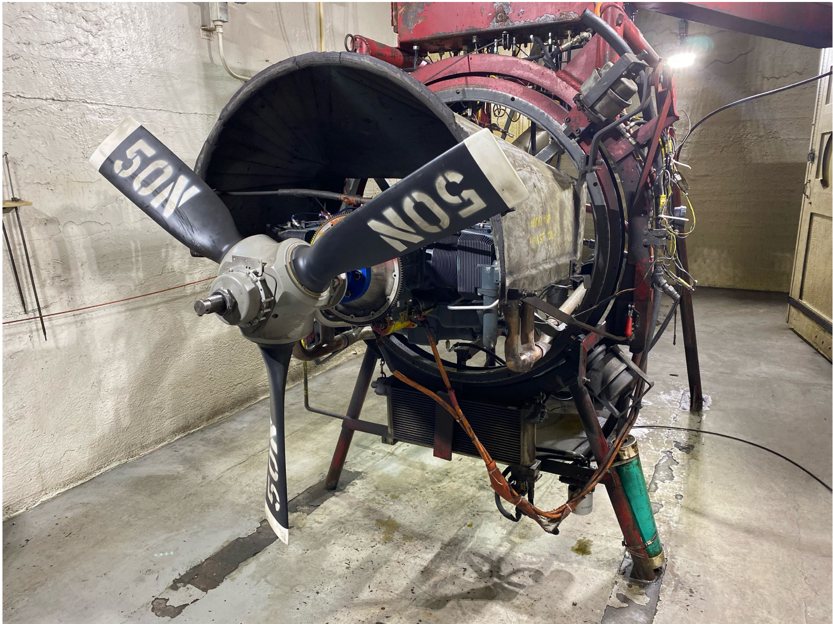
Photo 8 - Piper Digital Photograph. View of the Left Engine with Test Club Propeller Installed Prior to Engine Run.
