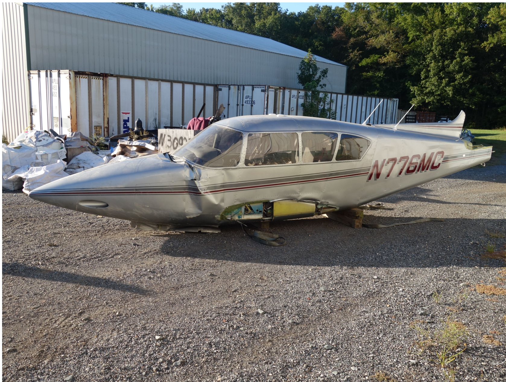
Photo 4 – Piper Digital Photograph. Left Side View of the Fuselage Following Recovery. Note the Structural Damage.
