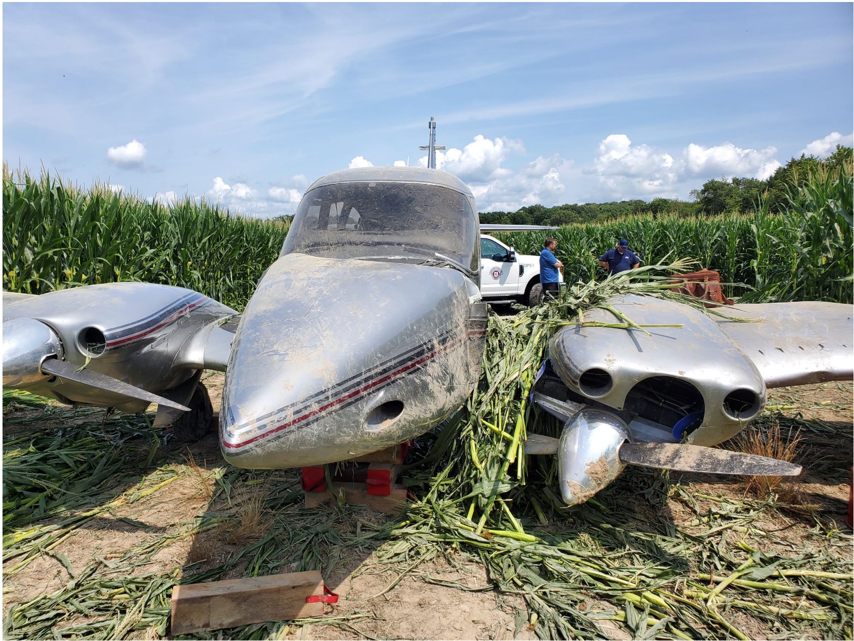
Photo 1 – FAA Digital Photograph. Frontal View of the Airplane at the Accident Site Depicting Inboard Portions of Both Wings. Note the Feathered Left and Right Propellers and Displaced Left Engine.
