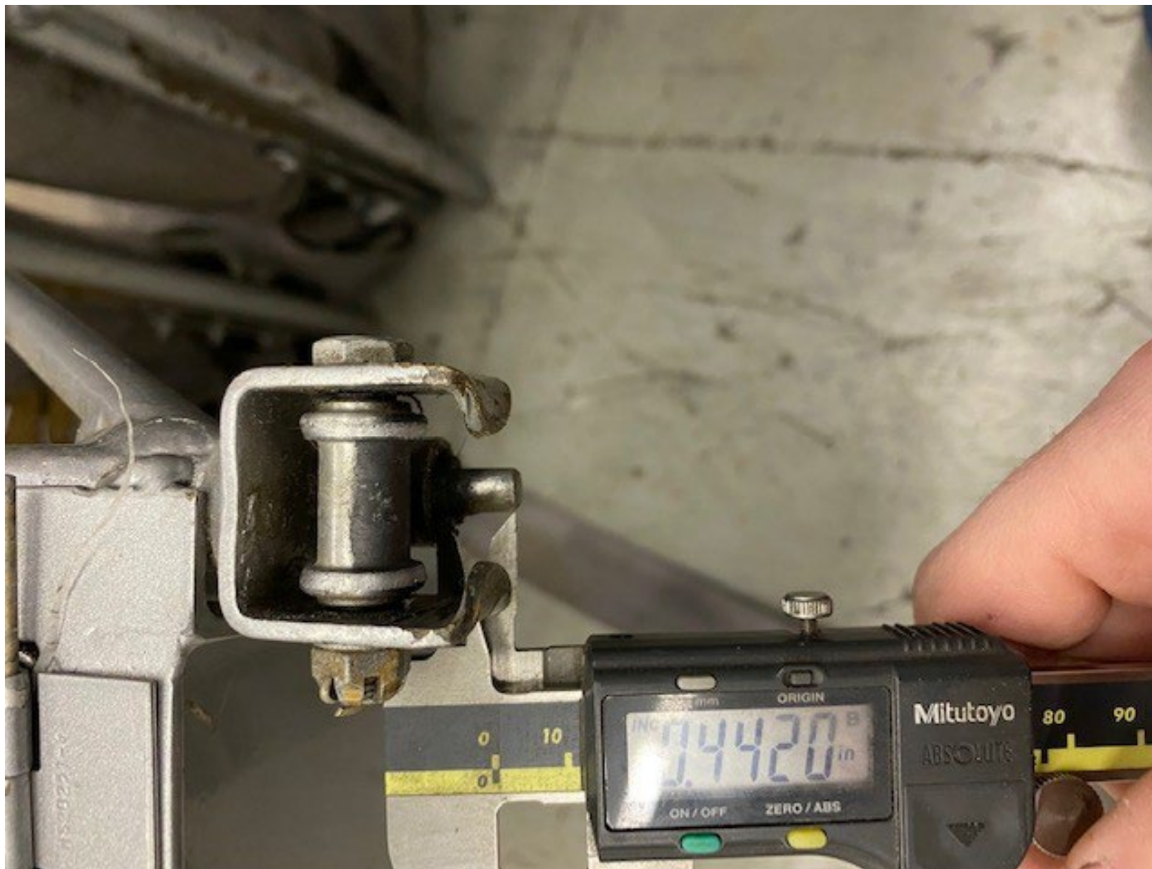
Photo 13 - FAA Digital Photograph. View of the Left Plunger-Seat Catch Extension of the Right Front Seat. Note the Extension of 0.4420 Inch From the Housing.
