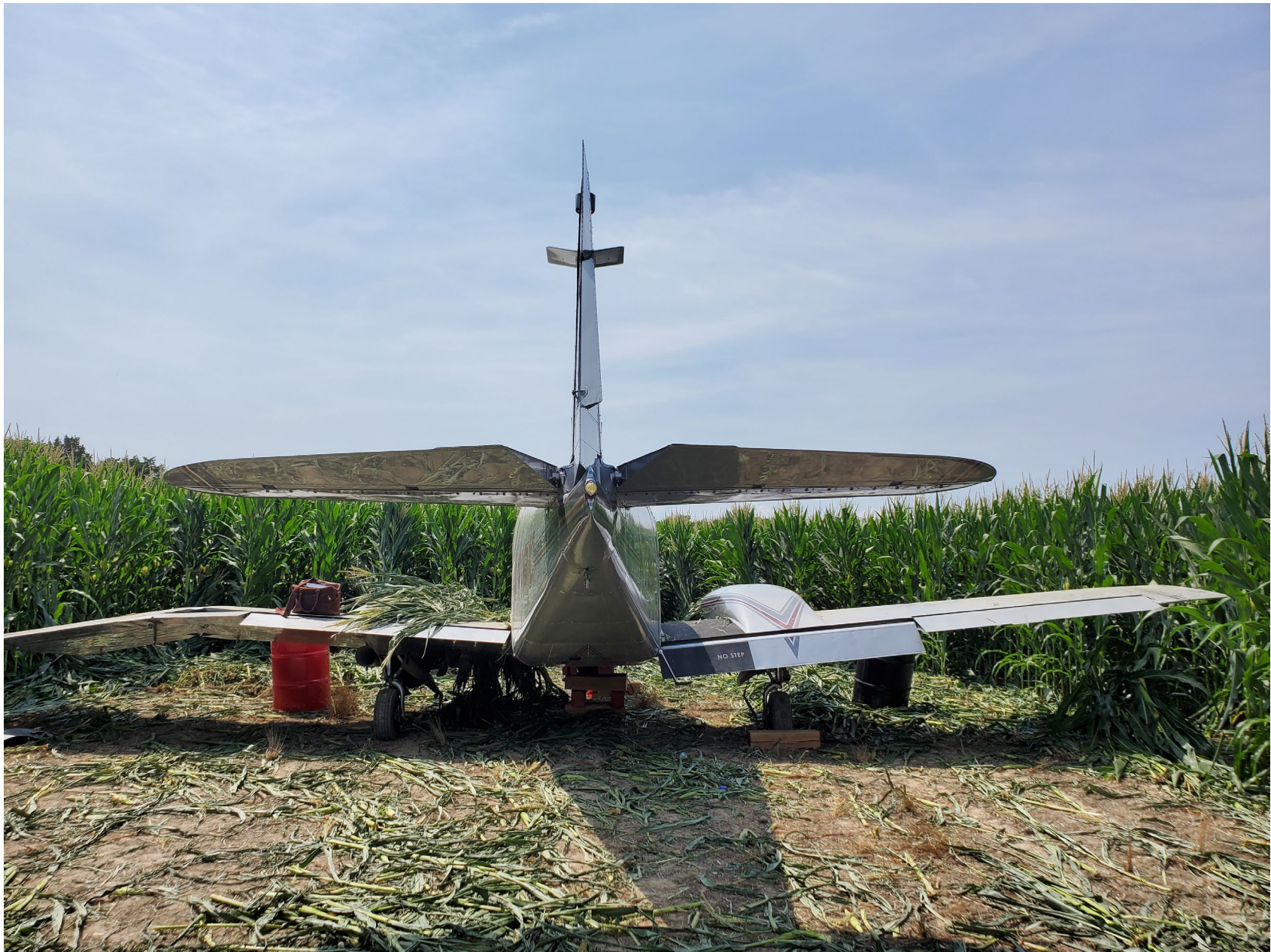
Photo 2 - FAA Digital Photograph. Rear View of the Airplane at the Accident Site. Note the Structural Damage to the Left Wing.
