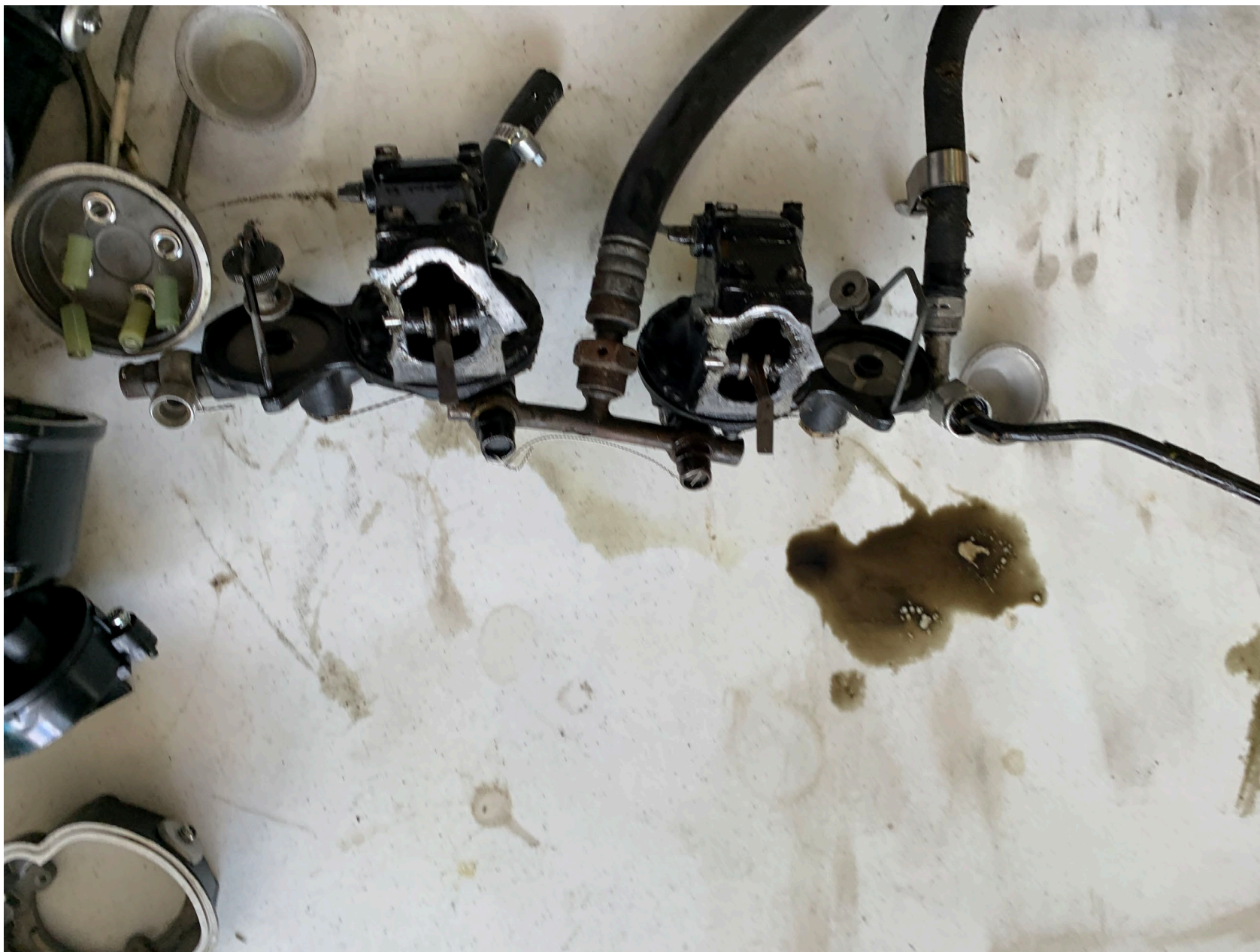
Photo 10 – Fuel Pumps (NTSB Photo)
