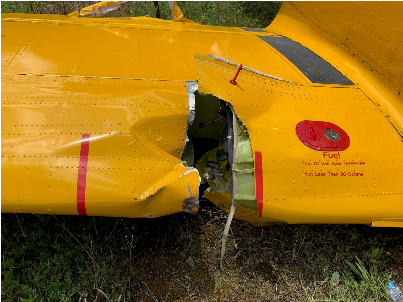
Photo 3 – Right Wing Damage (FAA Photo)
