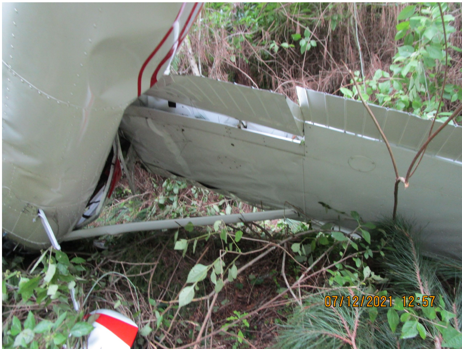
Photo 3 – View of right inboard wing damage. (Courtesy of FAA)
