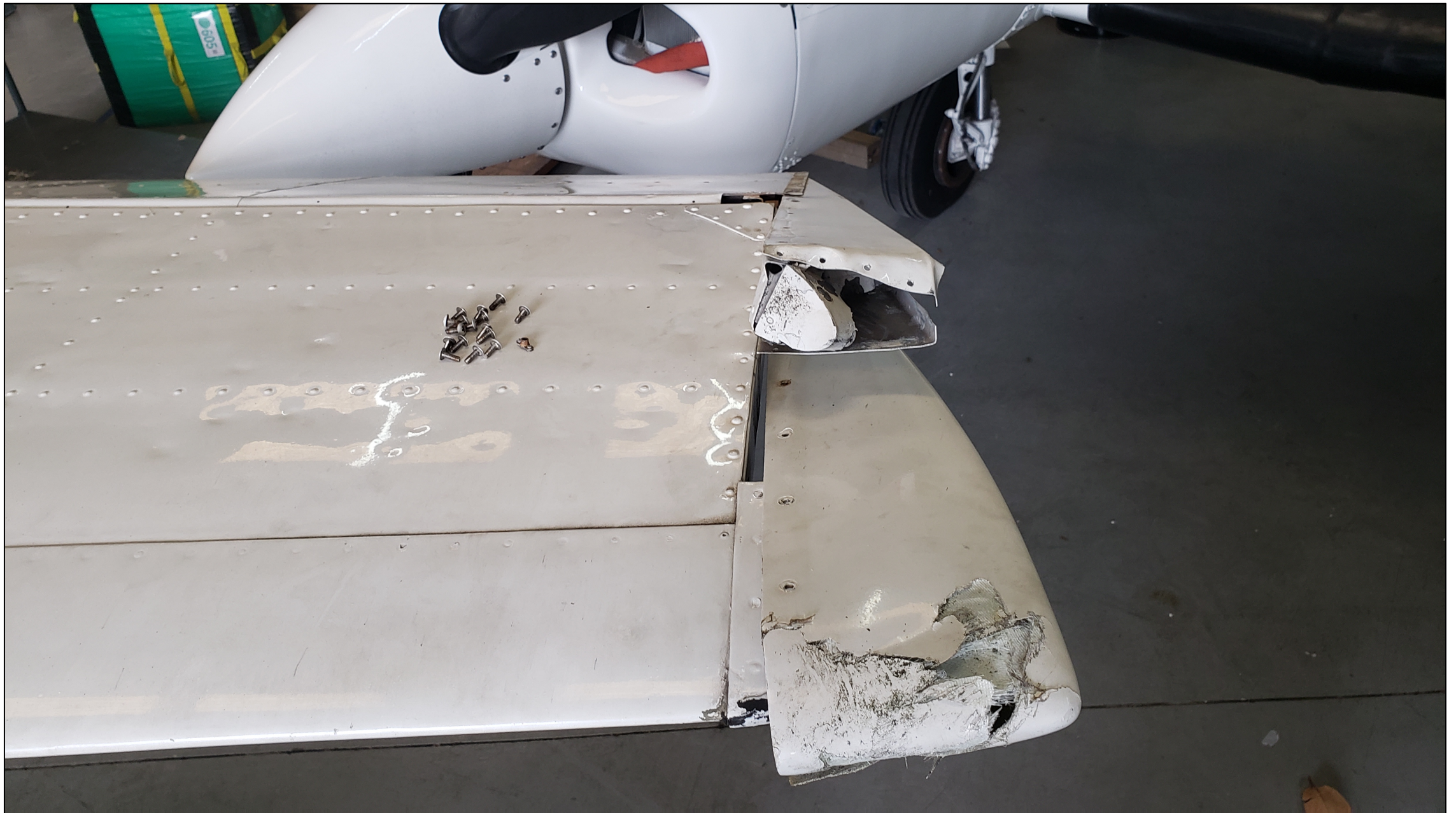
Photo 1 – View of the substantially damaged left elevator (Photo Courtesy of FAA)
