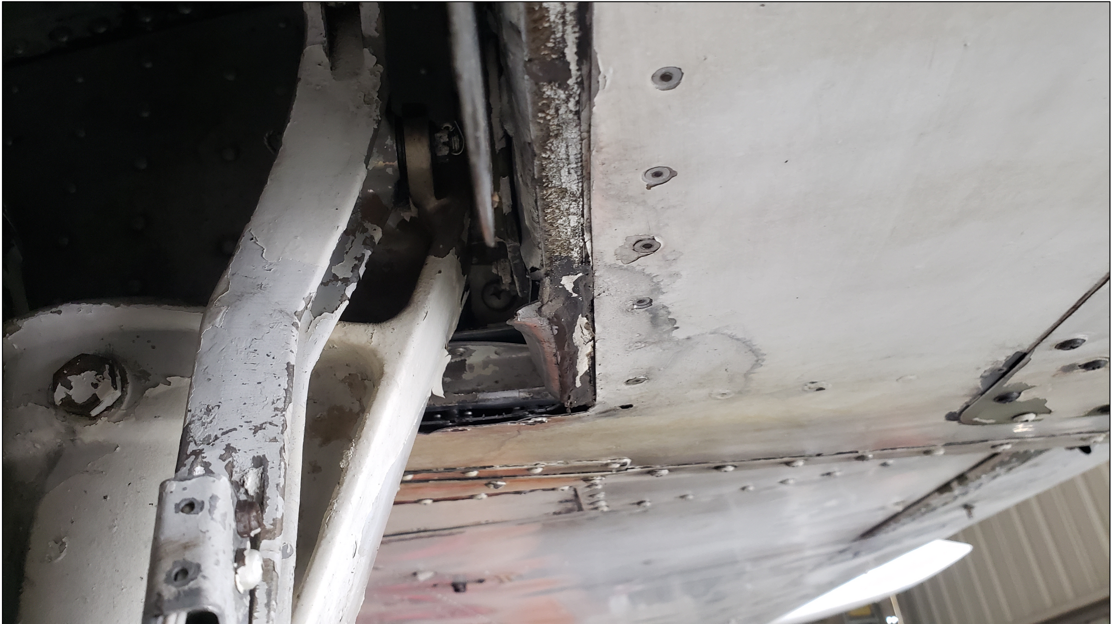
Photo 2 – View of the damaged left main landing gear assembly (Photo Courtesy of FAA)
