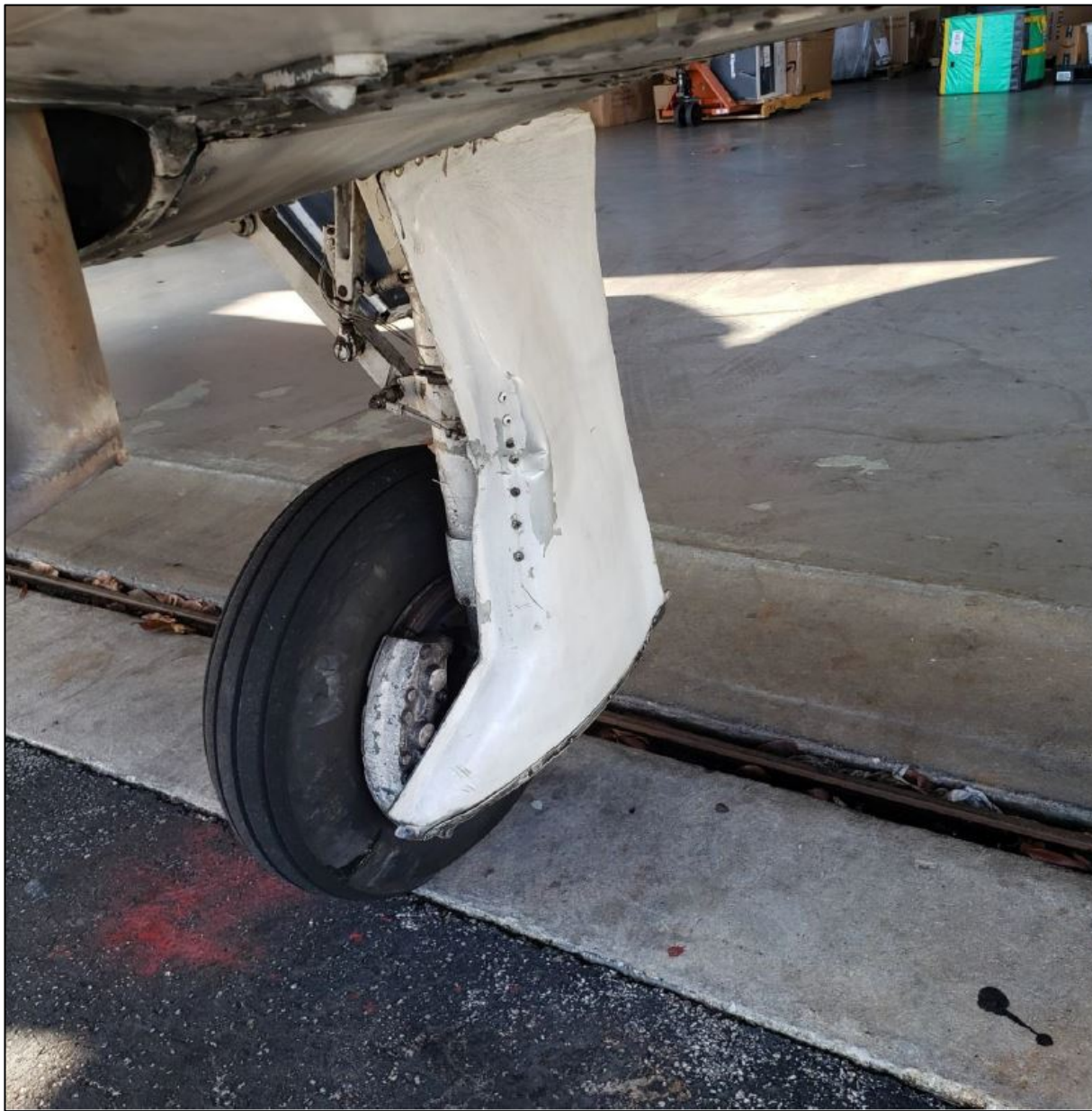
Photo 3 – Additional view of the left main landing gear damage (Photo Courtesy of FAA)
