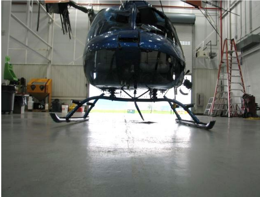
Figure 14 - Skids slightly spread (courtesy Bell)
