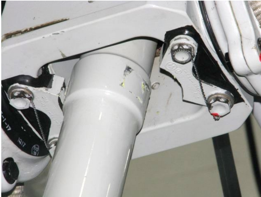
Figure 10 - Main rotor hub static stop contact from excessive hub flapping (courtesy Bell)
