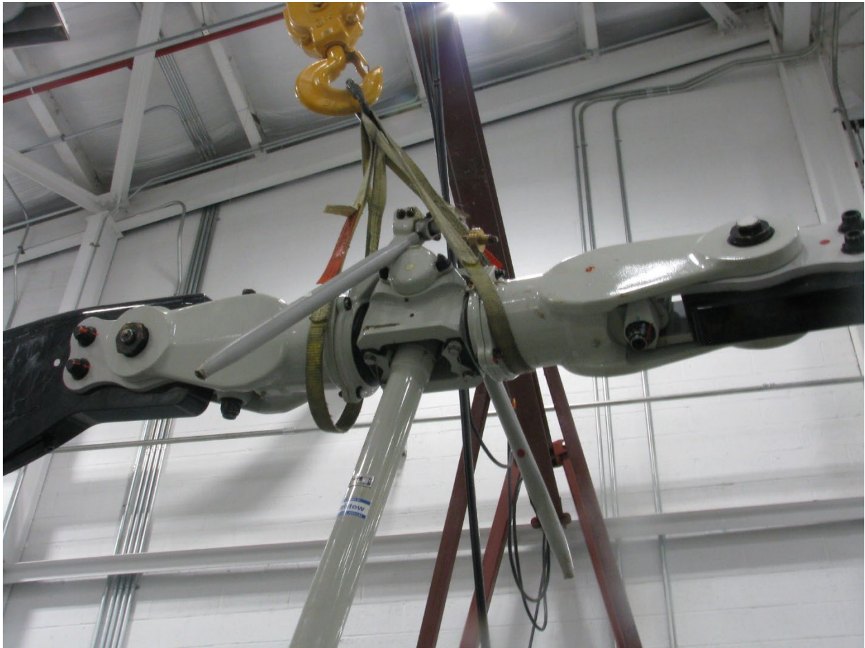
Figure 9 - Intact main rotor hub. Both pitch change links fractured at bottom swaged surfaces consistent with overload (courtesy Bell)
