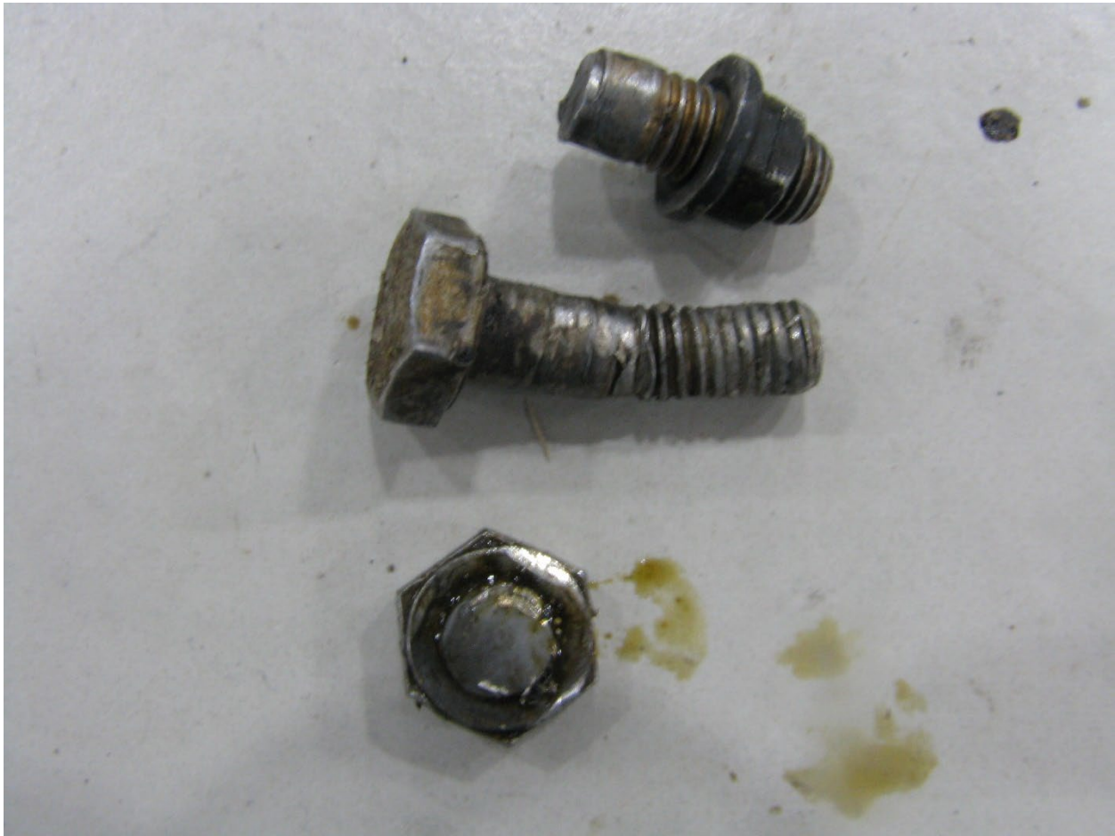
Figure 4 - Bolt remnants for main driveshaft outer coupling attachment to transmission input flange (courtesy Bell)
