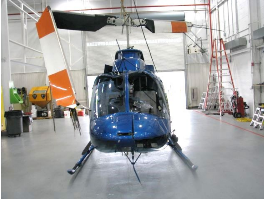
Figure 7 - Damage to main rotor blades (courtesy Bell)
