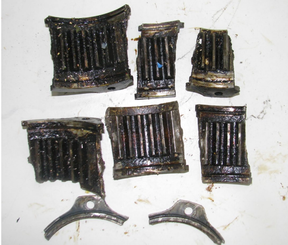
Figure 3 - Transmission side main driveshaft outer coupling (courtesy Bell)
