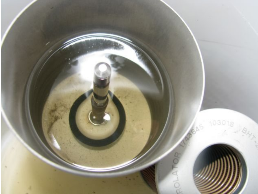
Figure 12 - Airframe fuel filter canister with clear/slight yellow fuel and small amount of particulate (courtesy Bell)
