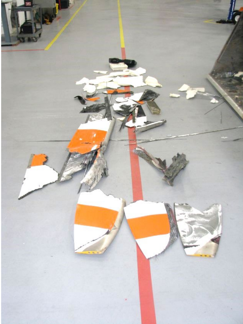
Figure 8 - Recovered blade fragments including tips, blade sections, trim tabs, and foam core (courtesy Bell)
