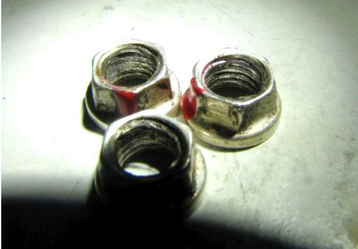
Figure 6 - Stripped silver plated nuts to secure engine end main driveshaft inner coupling to driveshaft tube (courtesy Bell)
