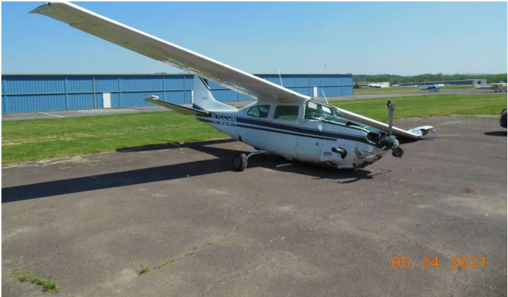
Photo 3 – View of the airplane, note substantial damage to the fuselage and left wing (Photo Courtesy of Airport Authority)
