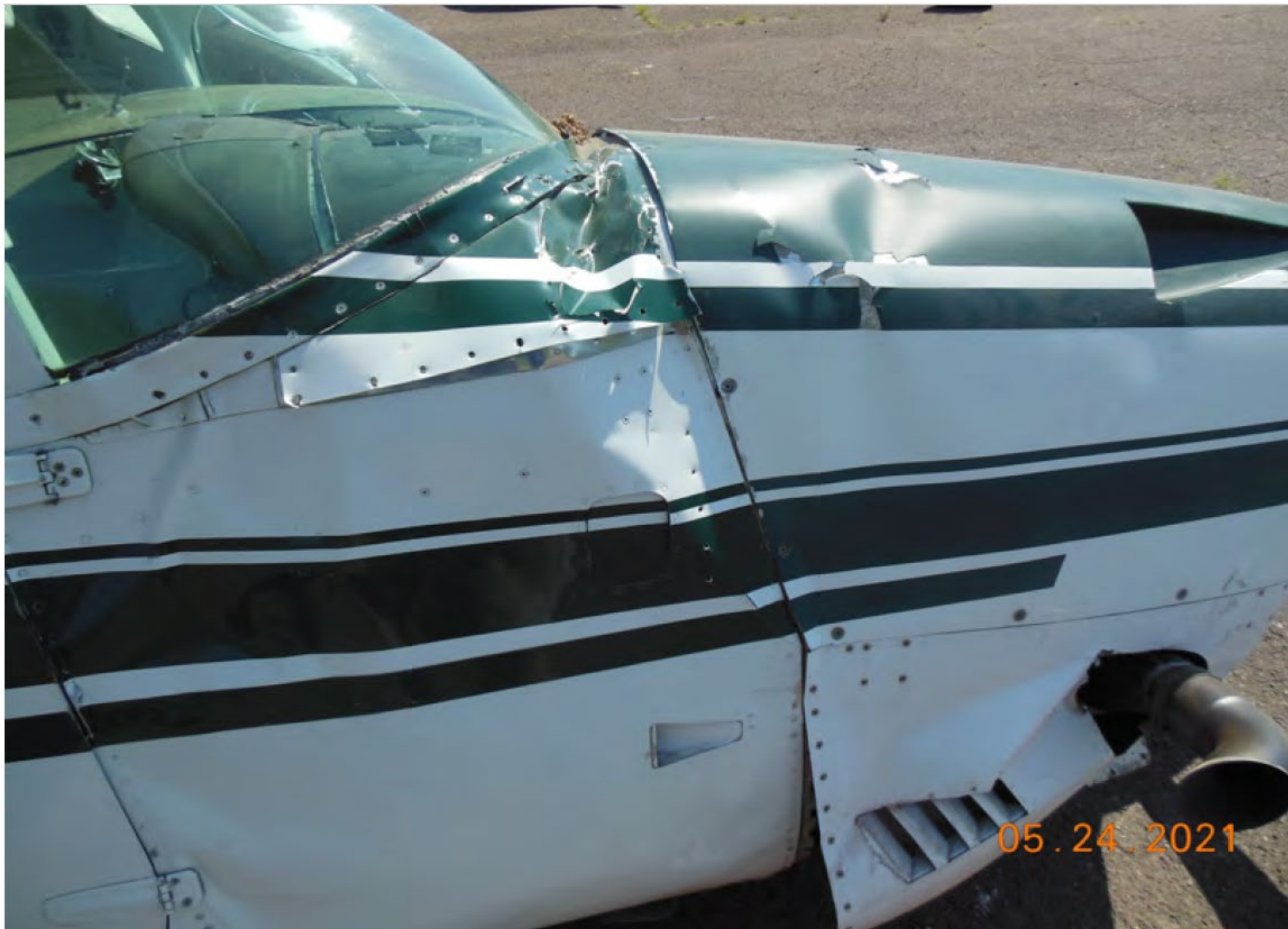
Photo 4 – Closer view of the fuselage damage (Photo Courtesy of Airport Authority)
