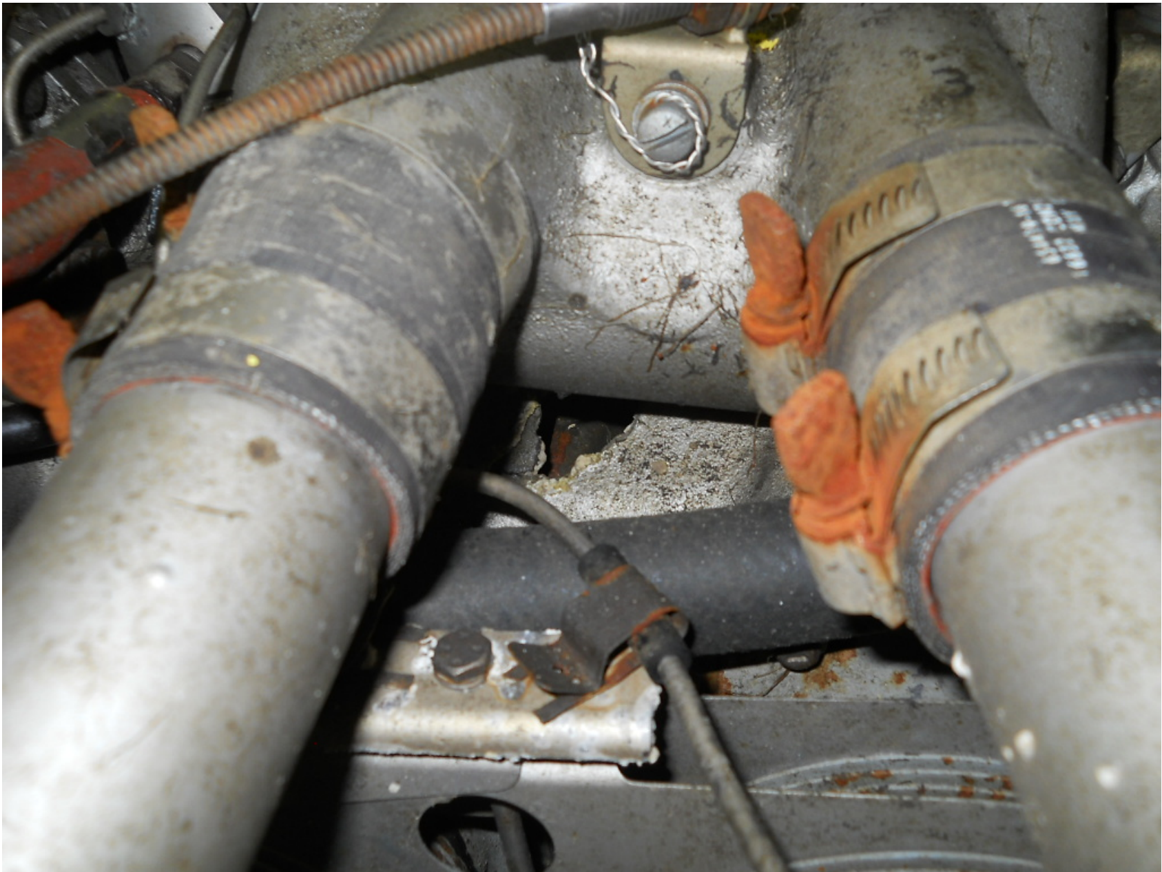
Photo 3 – Hole in Engine Crankcase
