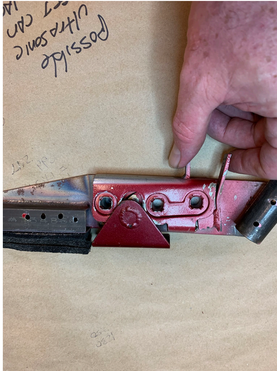
Photo 6 – Closeup view of canopy latch with striker pin in the latch mechanism. Note fingers on the trigger for scale.
