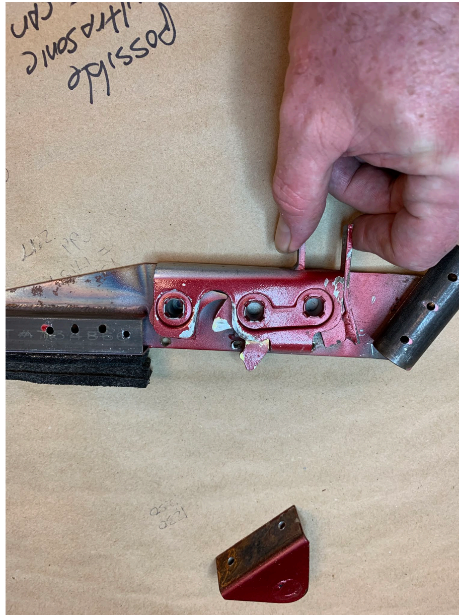
Photo 7 – Closeup view of canopy latch with striker pin ejected after applying pressure to trigger.
