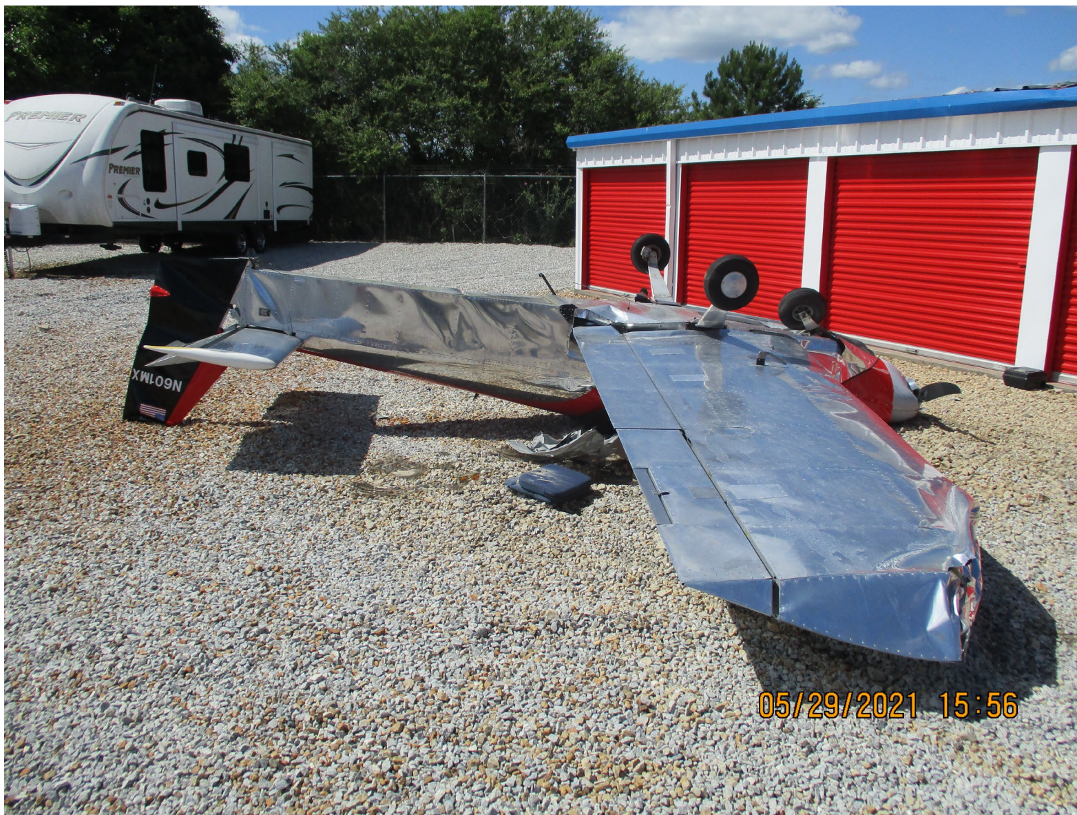
Photo 1 – View of inverted airplane adjacent to the structure it impacted. Note damage to wings and fuselage. (Courtesy of FAA)
