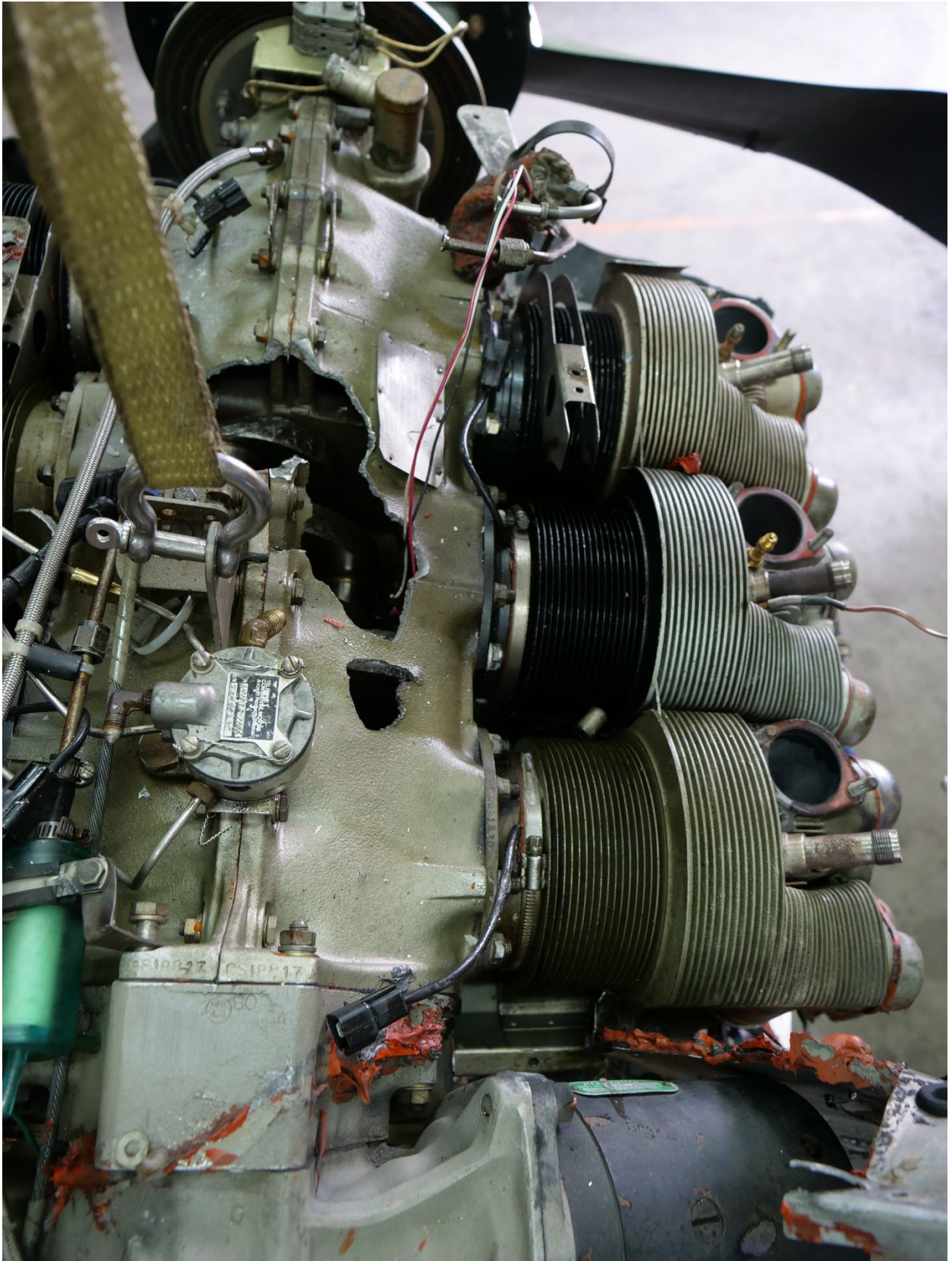
Photo 2: Two holes in the crankcase from the aft looking forward.
