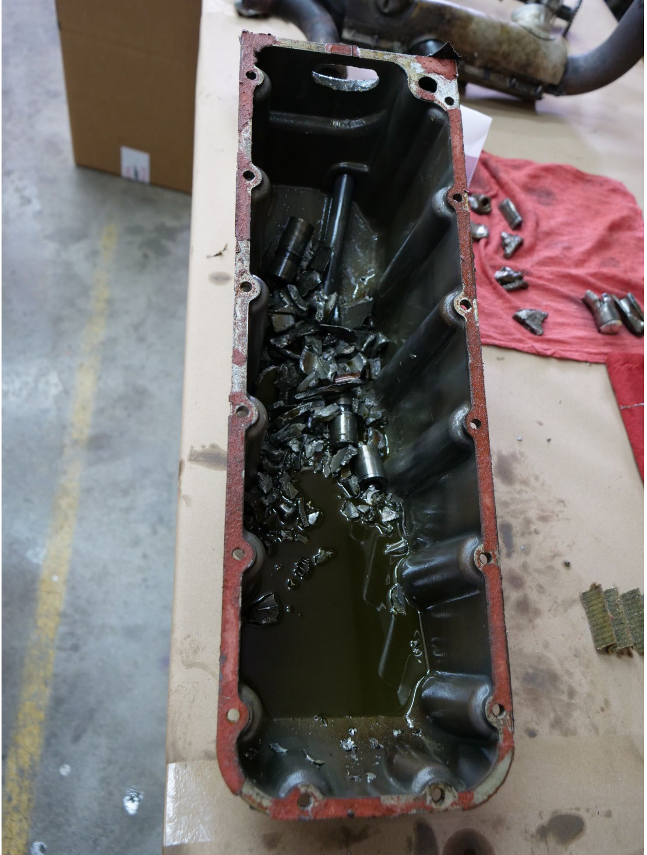
Photo 8: Oil pan containing a large amount of metallic debris.
