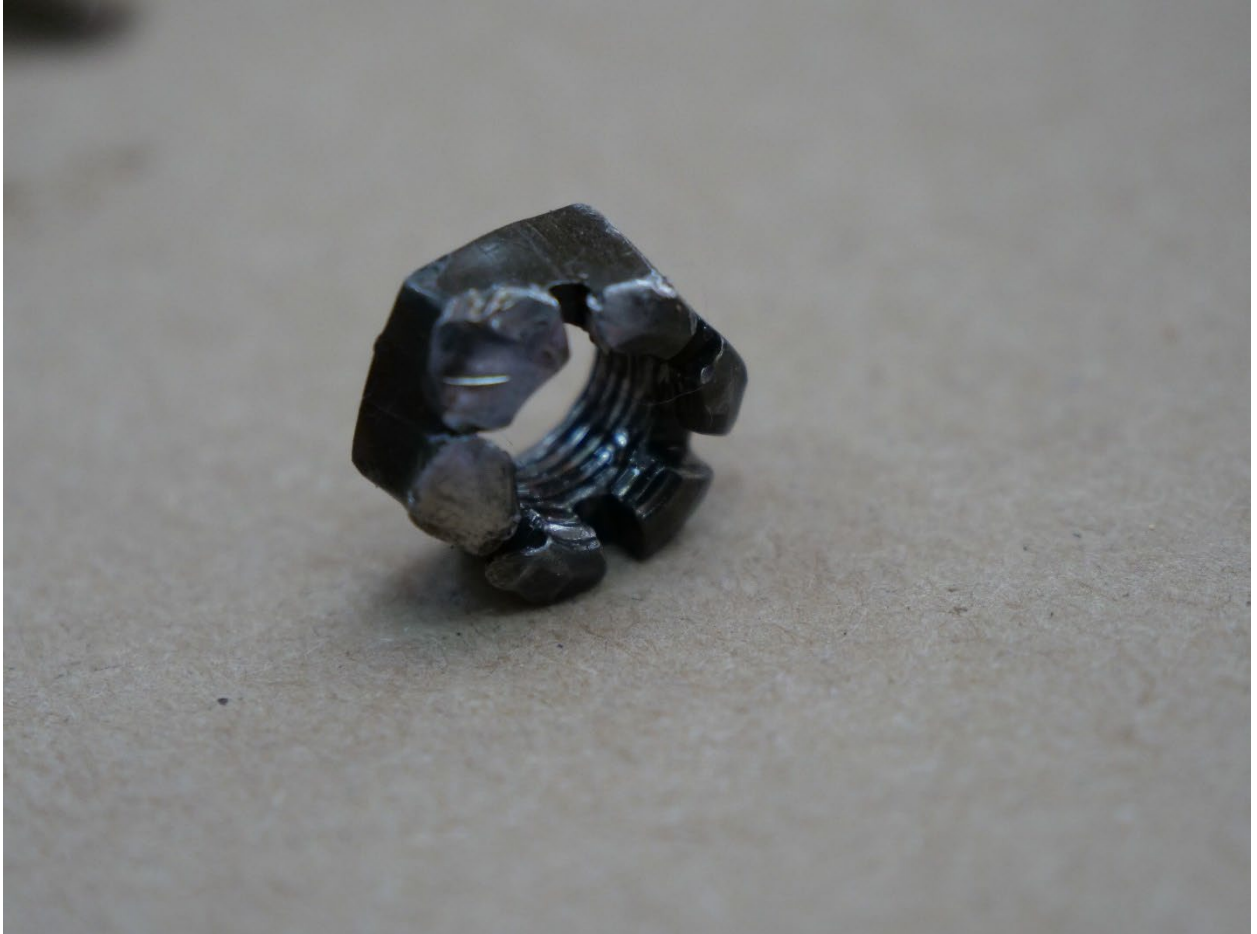
Photo 6: No. 4 Connecting Rod Cap Nut (no bolt or cotter pin)
