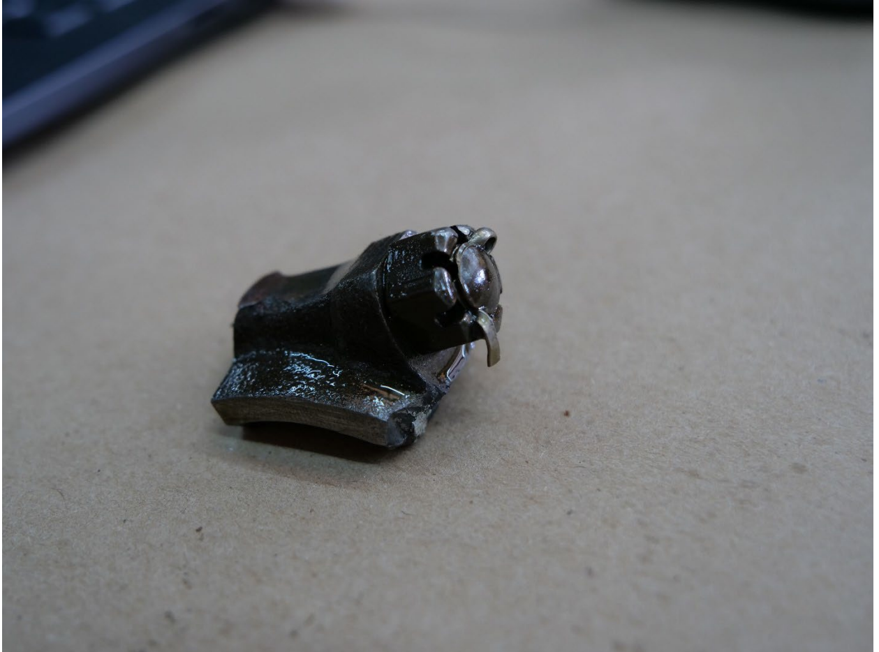
Photo 5: No. 4 Connecting Rod Cap Bolt, Nut, And Cotter Pin
