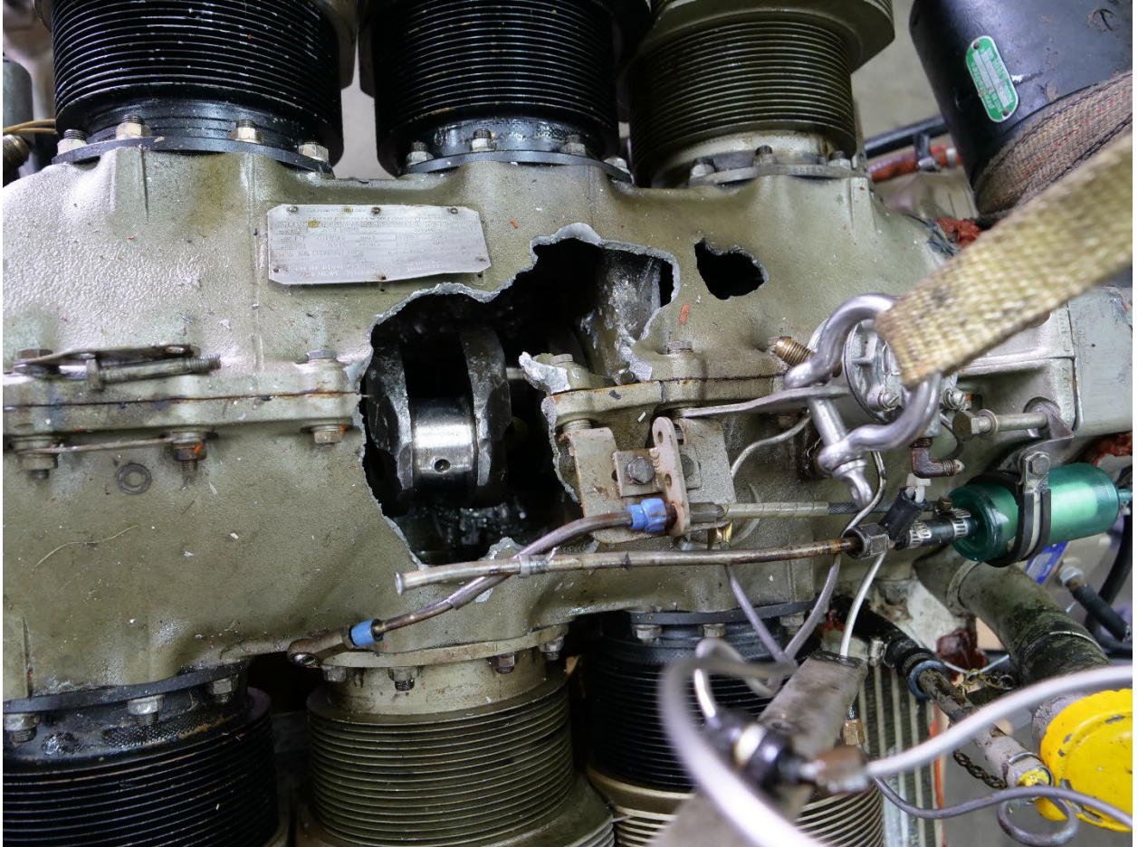
Photo 3: Top view of the holes in the crankcase.
