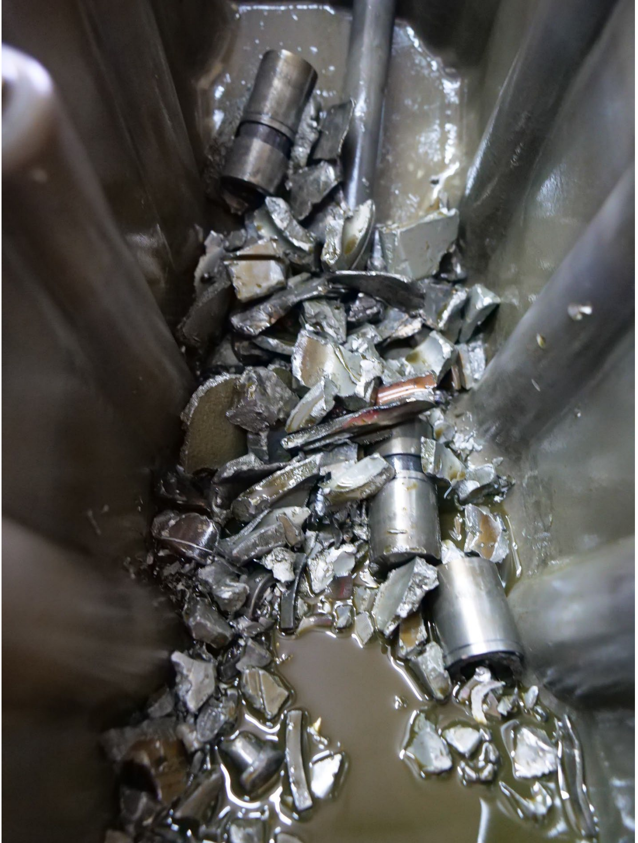
Photo 9: Metallic debris located in the oil pan.
