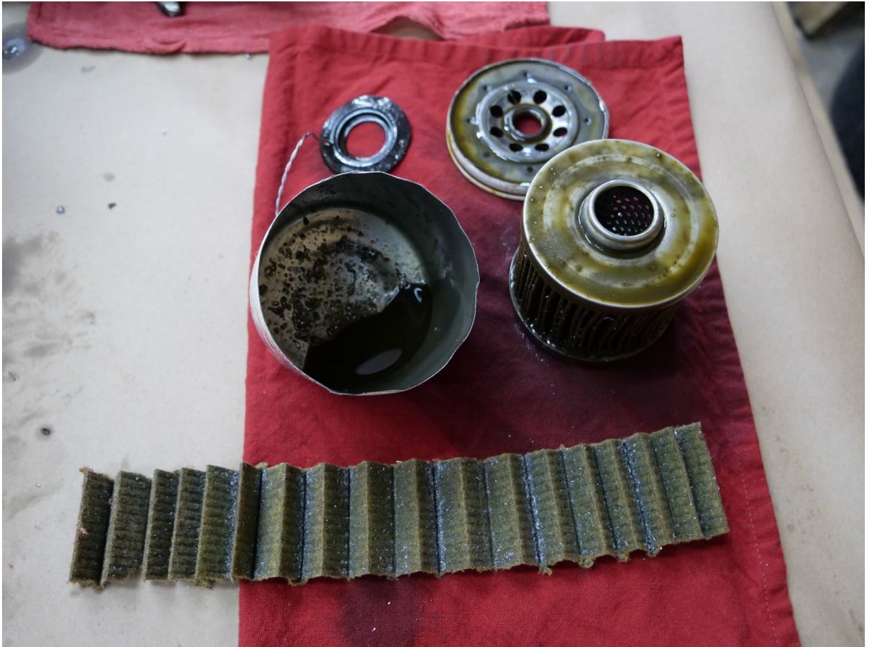
Photo 7: Oil filter pleats containing a large amount of metallic debris.
