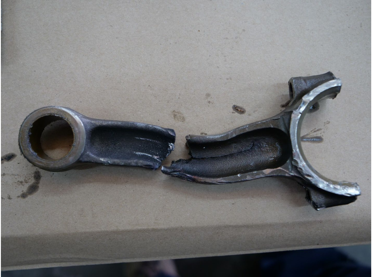
Photo 4: No. 4 connecting rod
