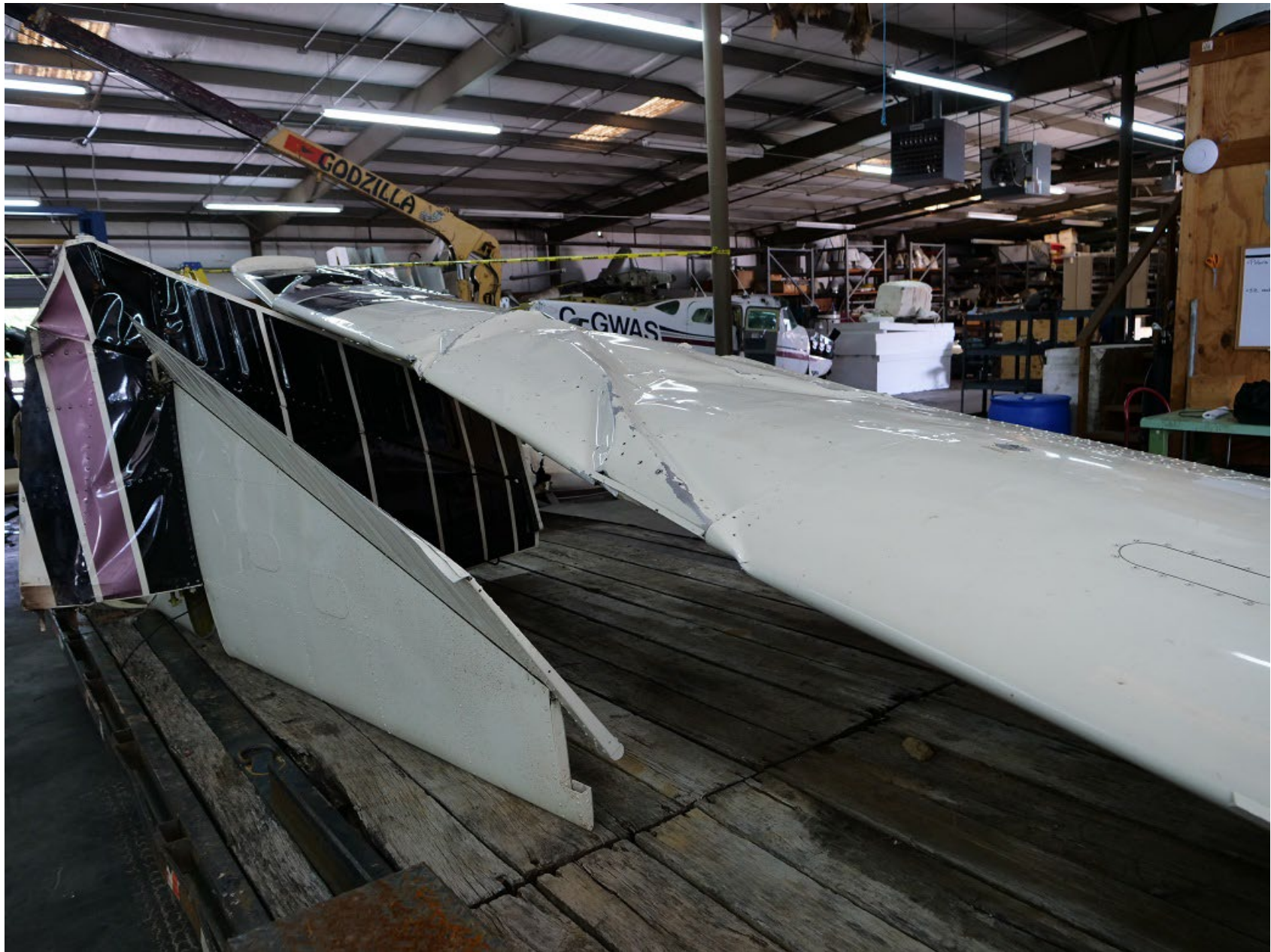
Photo 2 – Right Wing Damage
