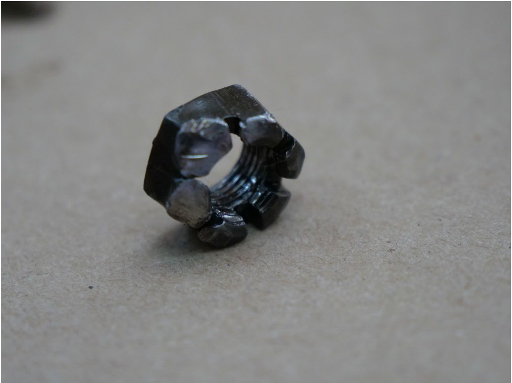
Photo 7 – No. 4 Connecting Rod Cap Nut (no bolt or cotter pin)
