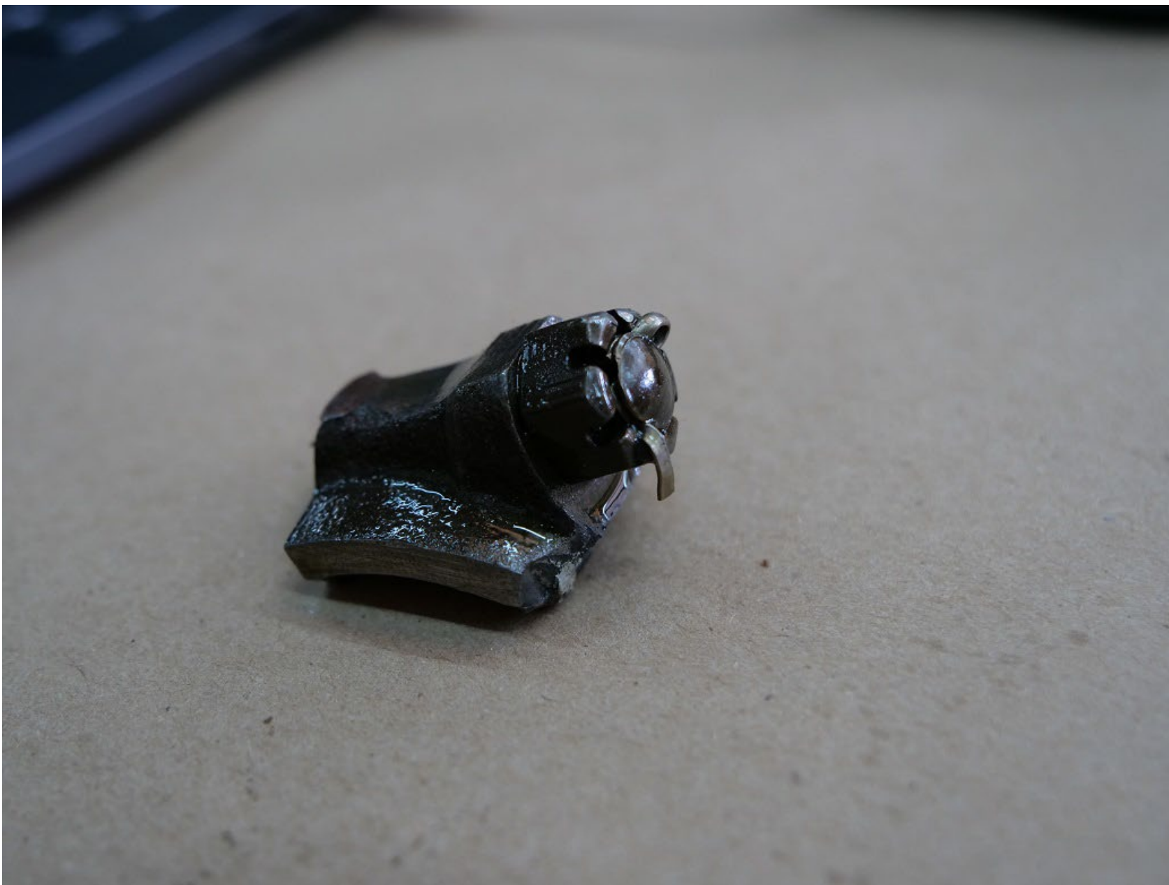
Photo 6 – No. 4 Connecting Rod Cap Bolt, Nut, And Cotter Pin
