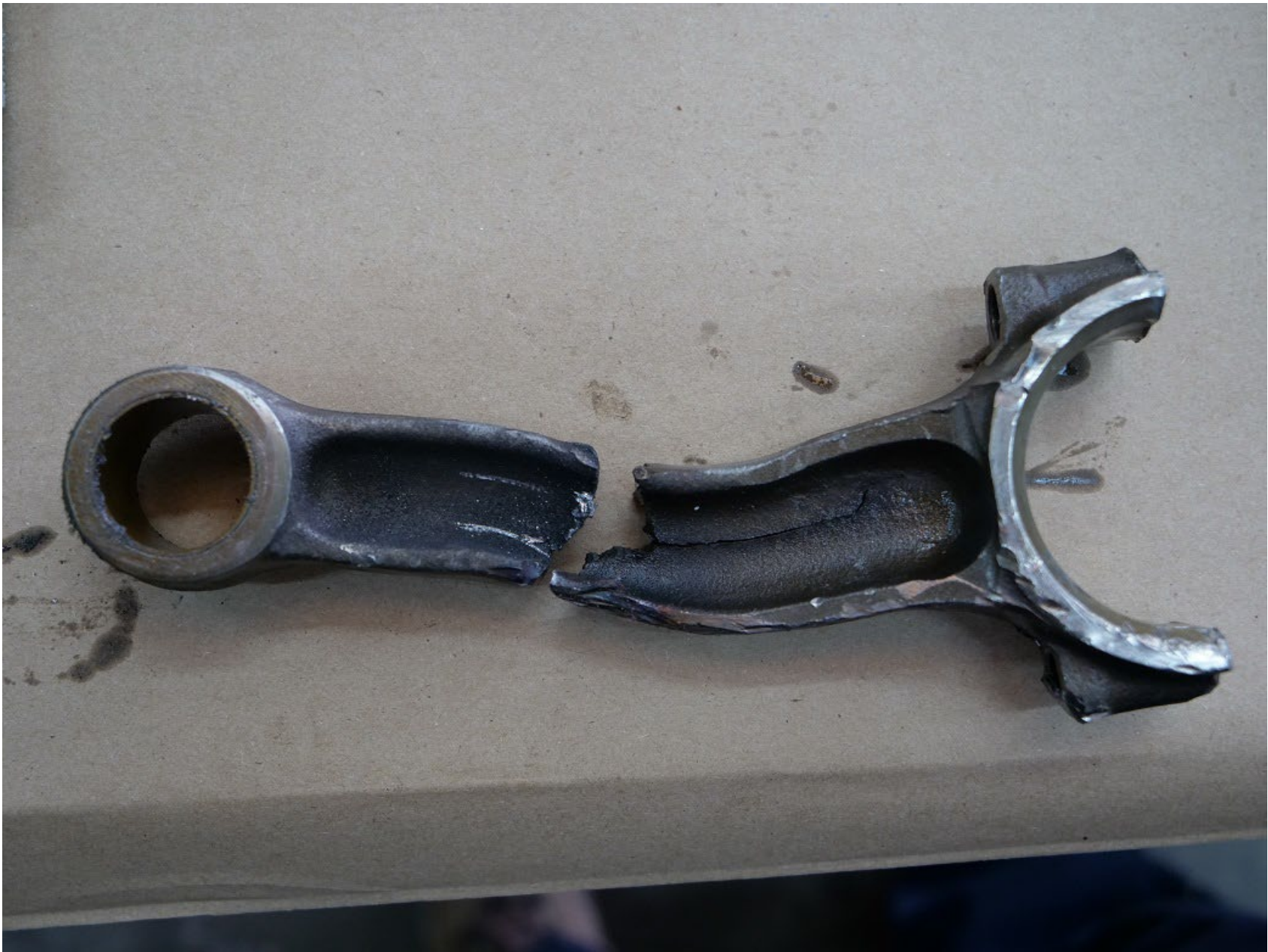
Photo 5 – No. 4 Connecting Rod
