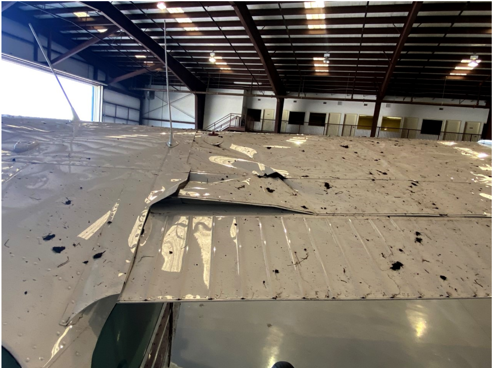
Photo 4 - Digital Photograph From FAA. View Looking Forward of the Inboard Portion of the Right Wing. Note the Skin Buckling and Wrinkling at the Aft Spar Area.
