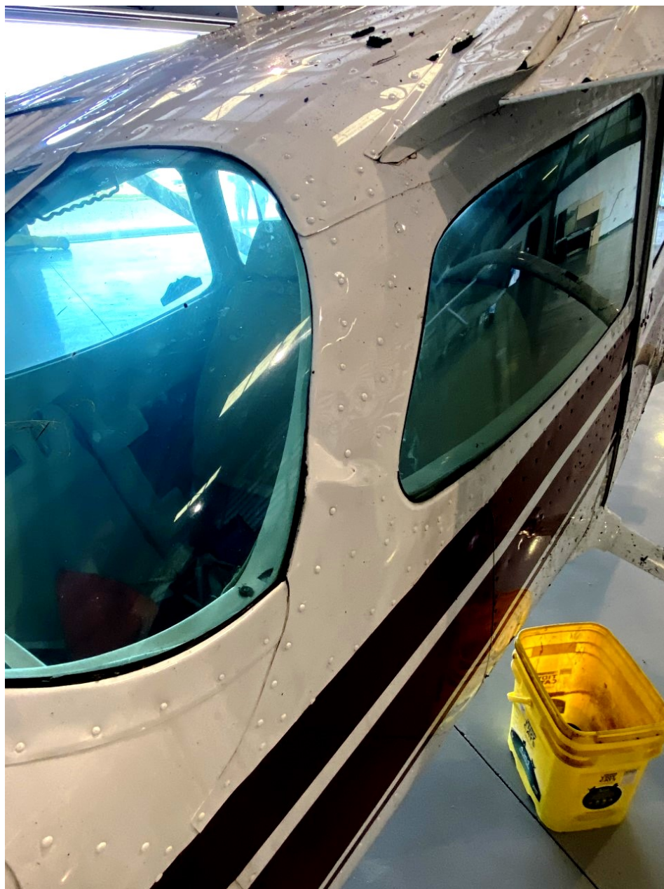
Photo 5 - Digital Photograph From FAA. View of the Right Side of the Fuselage near the Right Aft Window and the Aft Window. Note the Skin Buckling and Wrinkling.
