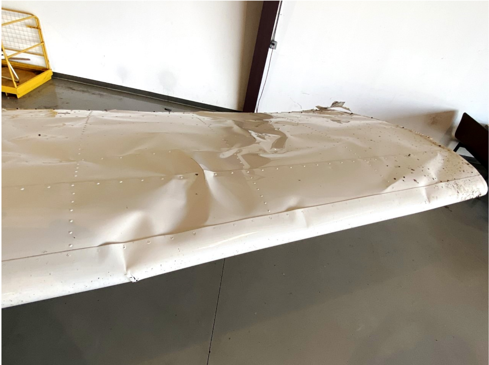
Photo 3 – Digital Photograph From FAA. View Looking Aft of the Outer Portion of the Left Wing. Note the Damage to the Skin Across the Main Spar, and the Skin Buckling and Wrinkling.
