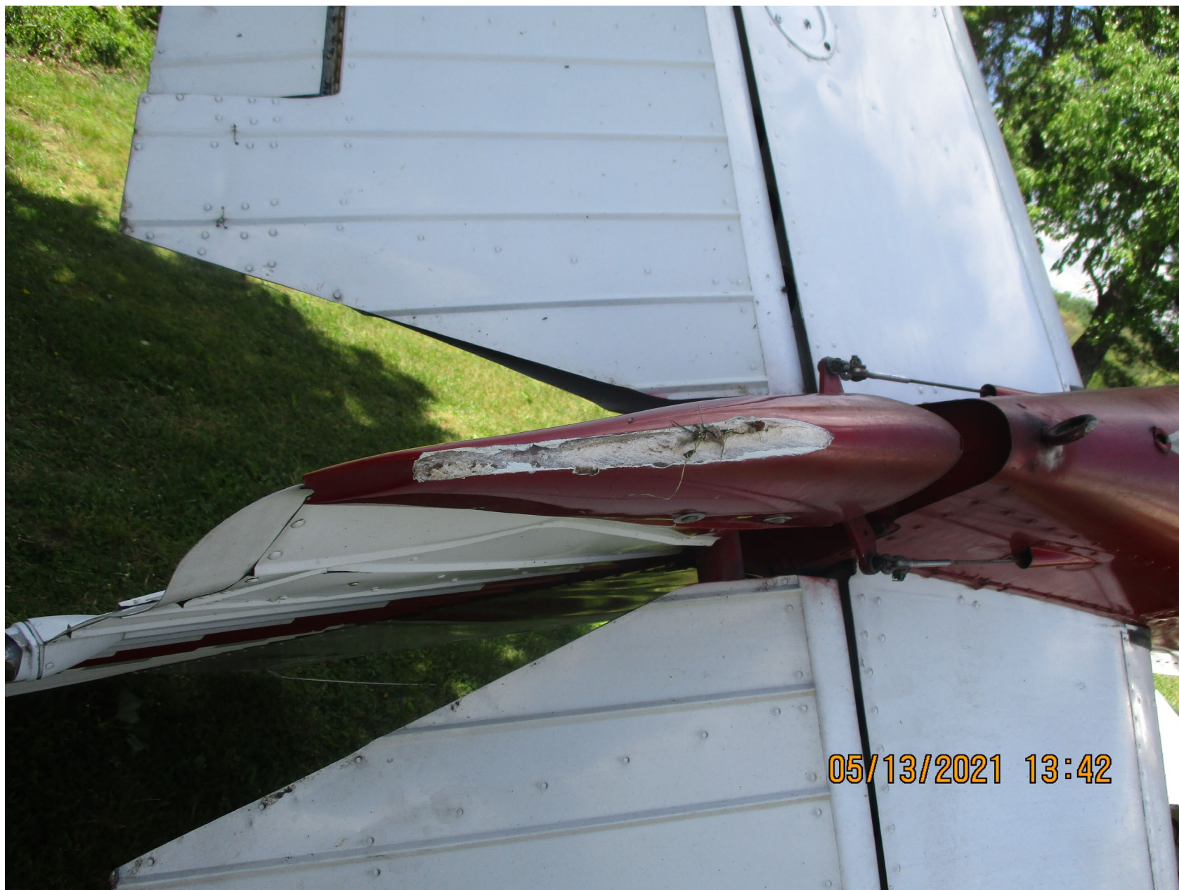
Photo 12 – Scrape on Bottom of Rudder – Courtesy of FAA
