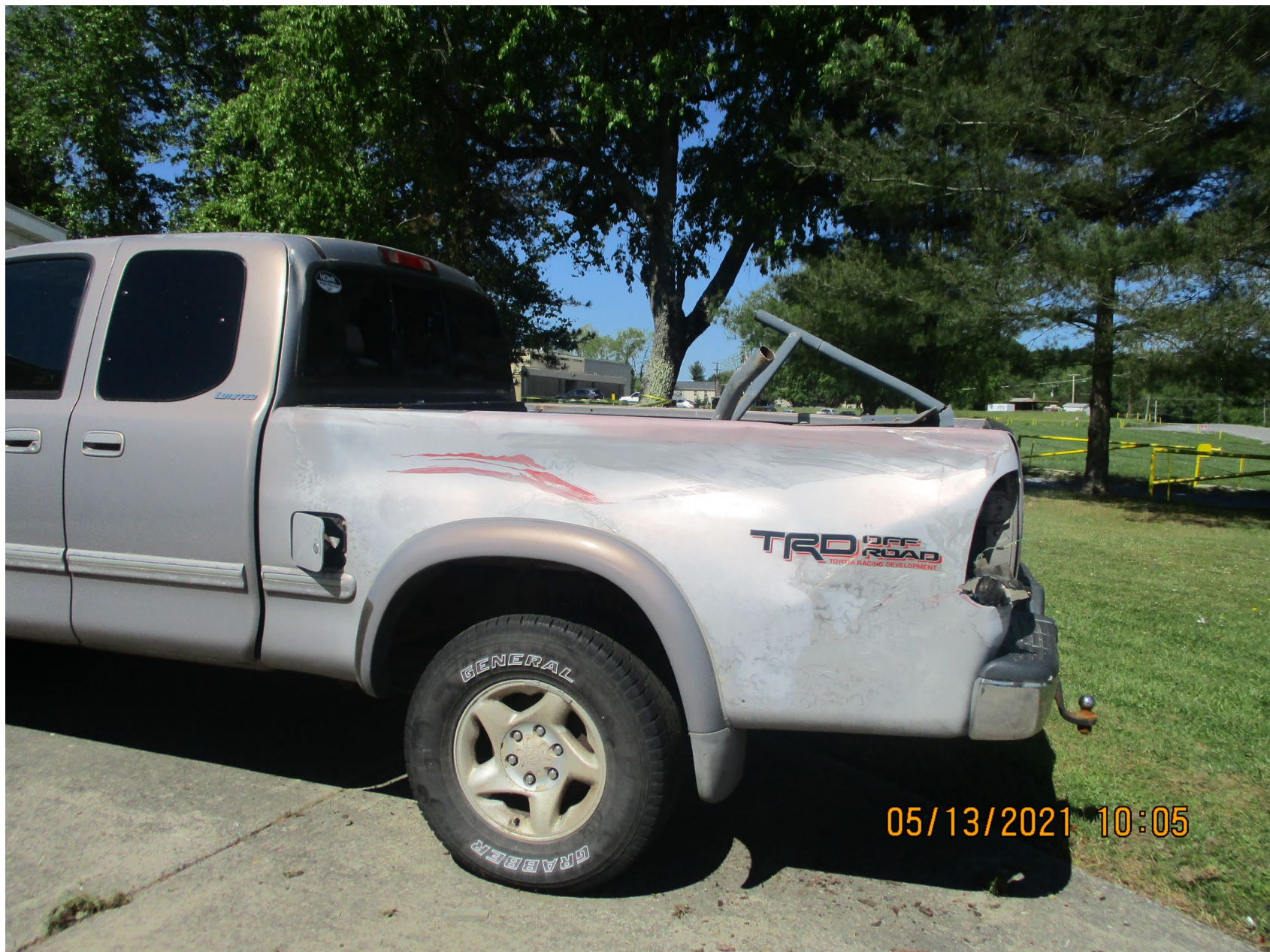
Photo 5 – Paint Transfer on Damaged Truck – Courtesy of FAA
