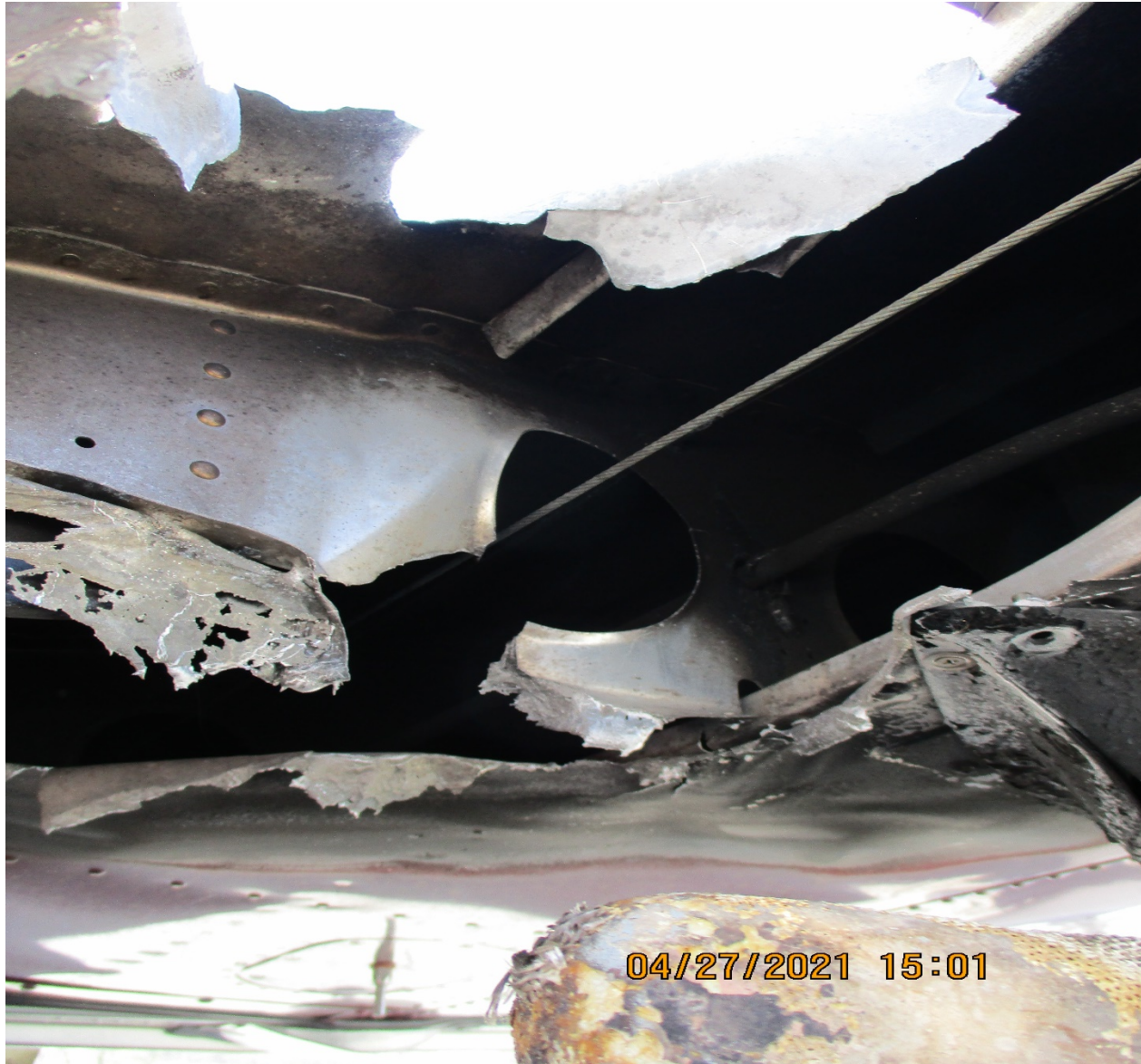
Photo 2 – View of right wing assembly showing fire damage
