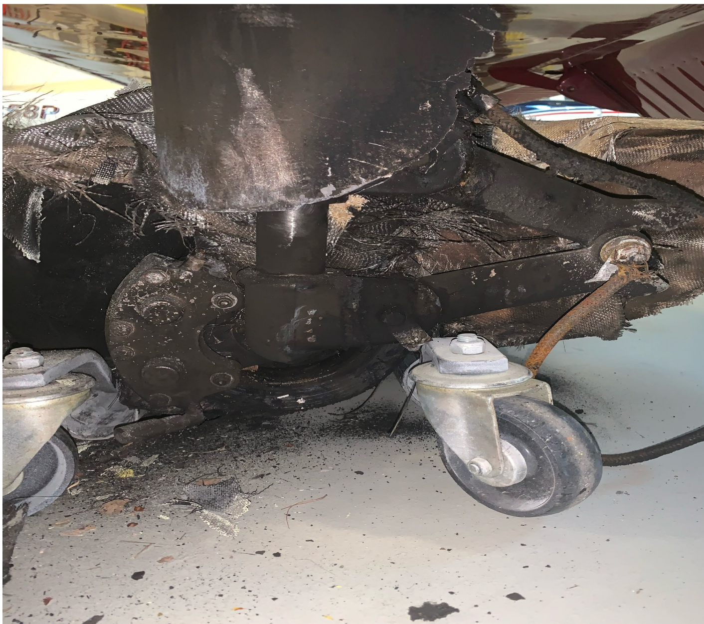
Photo 1 – View of right main landing gear brake assembly showing fire damage
