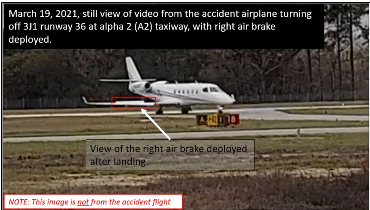
Figure 13: March 19, 2021, still view of video from the accident airplane turning off 3J1 runway 36 at alpha 2 (A2) taxiway after landing, with air brakes deployed.
