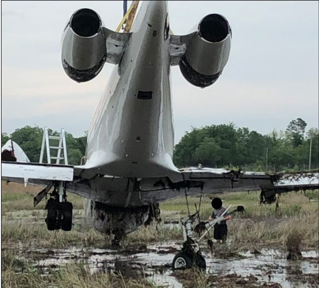
Figure 14: View of the left and right MLG as viewed during the recovery operation.
