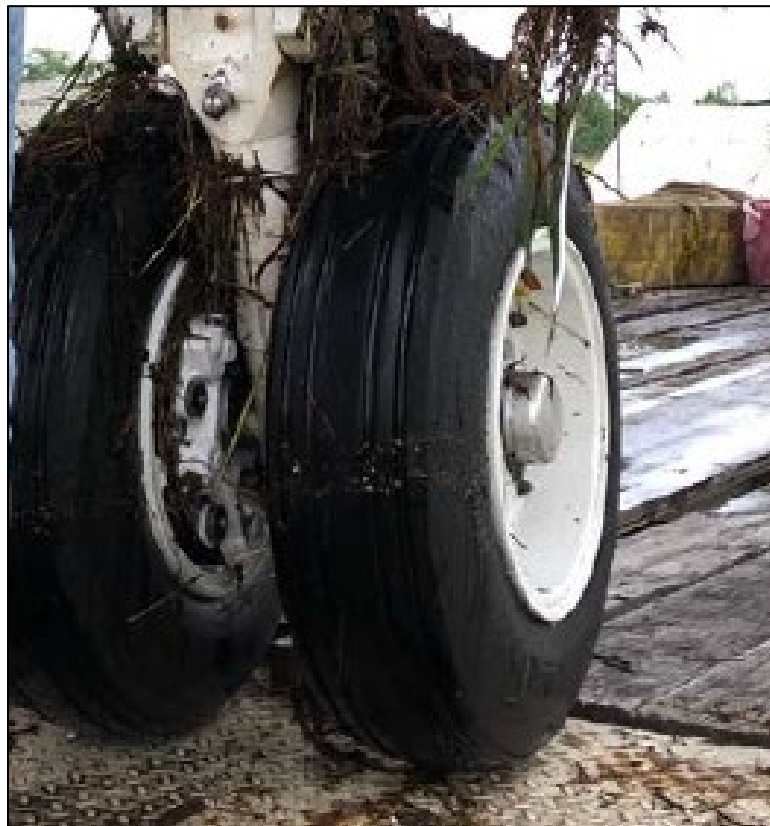
Figure 16: View of the right MLG post-recovery.
