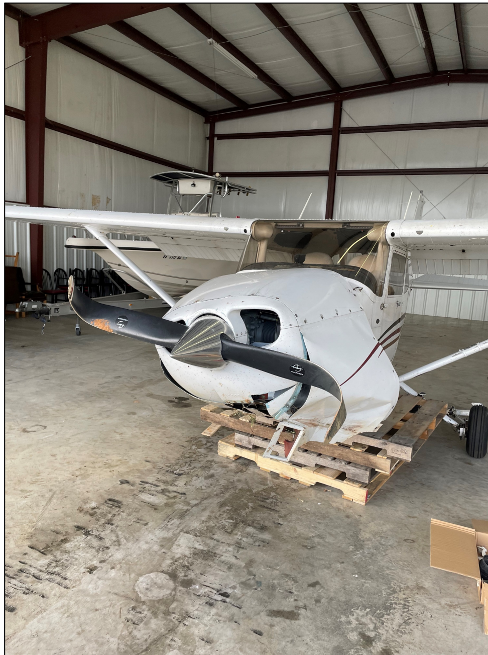
Photo 1 – View of the airplane damage sustained to the forward fuselage and engine area (Photo Courtesy of FAA)
