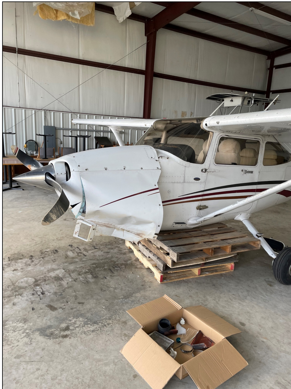
Photo 3 – Overview of the damaged cowling and fuselage area (Photo Courtesy of FAA)
