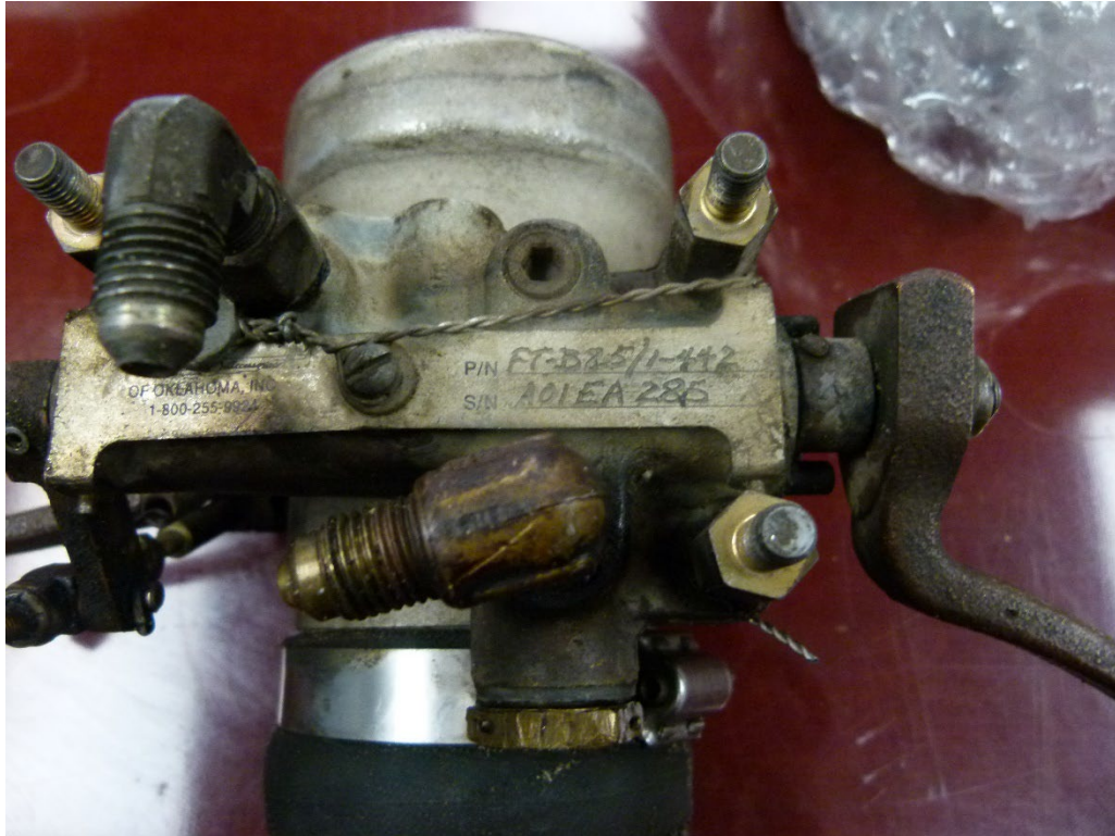
Figure 3: Digital Photograph from CAT. View of the Throttle Body and Metering Valve.
