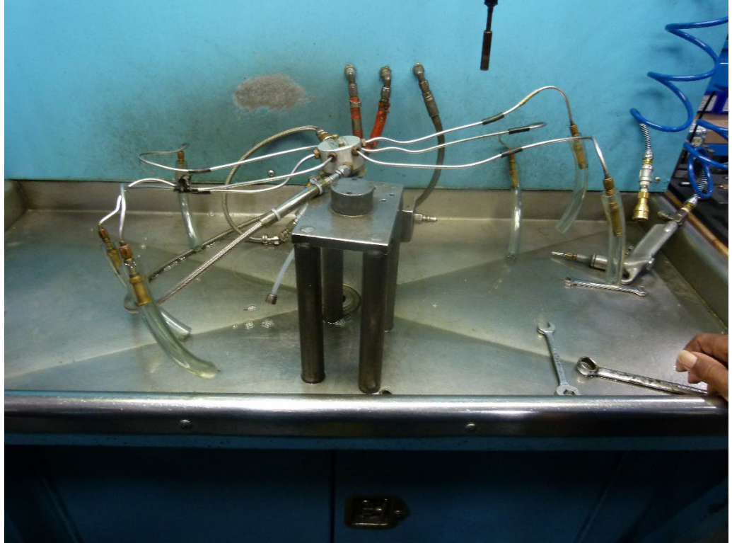
Figure 8: Digital Photograph from CAT. View of the Testing of the Manifold Valve Injector Lines and Injector Nozzles.
