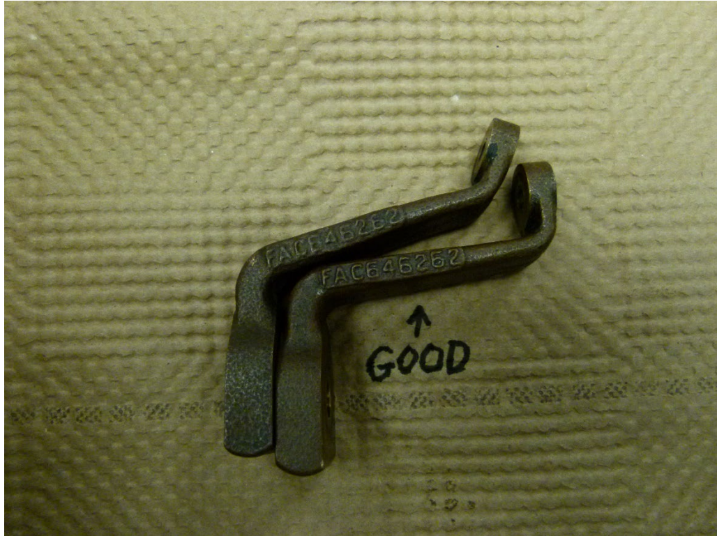
Figure 6: Digital Photograph from CAT. View of the Accident Throttle Control Lever on Top and Exemplar Lever on the Bottom. Note the Impact Damage to The Accident Lever Near Both Ends.
