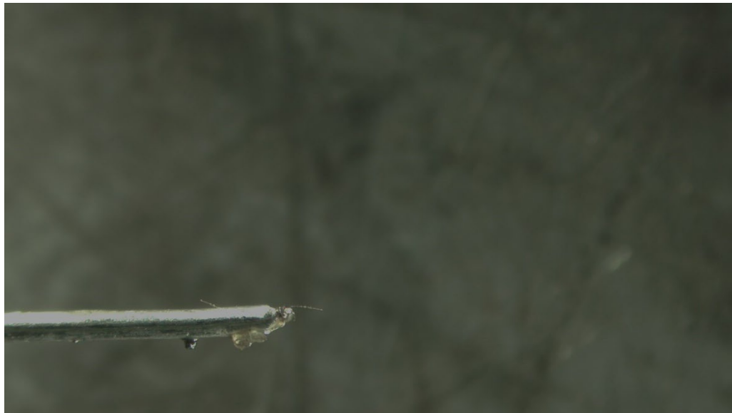
Figure 7: Microscope Image From CAT. View of the Debris removed from the No. 1 Fuel Injector Nozzle. The horizontal component holding the object is a piece of safety wire no more than 0.032 inch in diameter.
