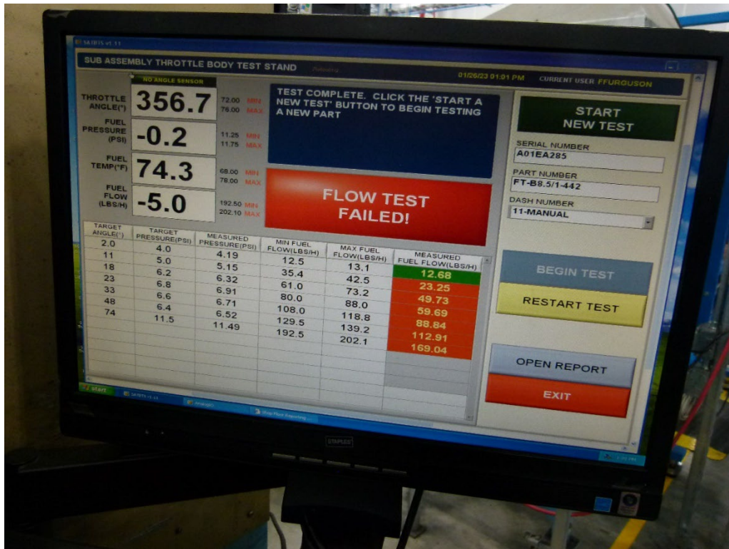
Figure 5: Digital Photograph from CAT. View of the Throttle Body and Metering Valve Subsequent Test Result to a -11 Cam.
