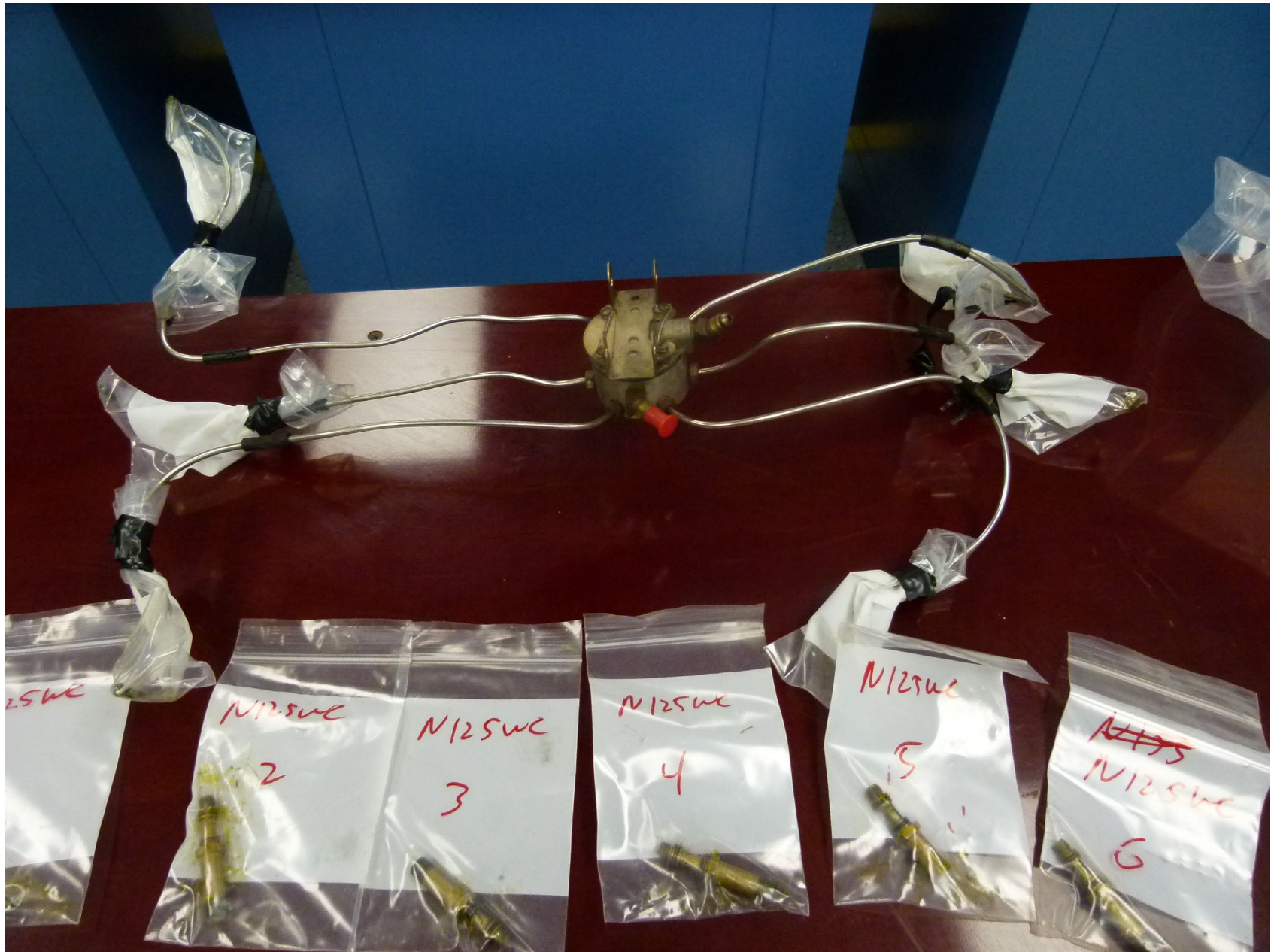
Photo 10 – Continental Aerospace Technologies Digital Photograph. View of the Manifold Valve or Flow Divider with Attached Fuel Injector Lines and Separated Fuel Injector Nozzles Prior to Testing.
