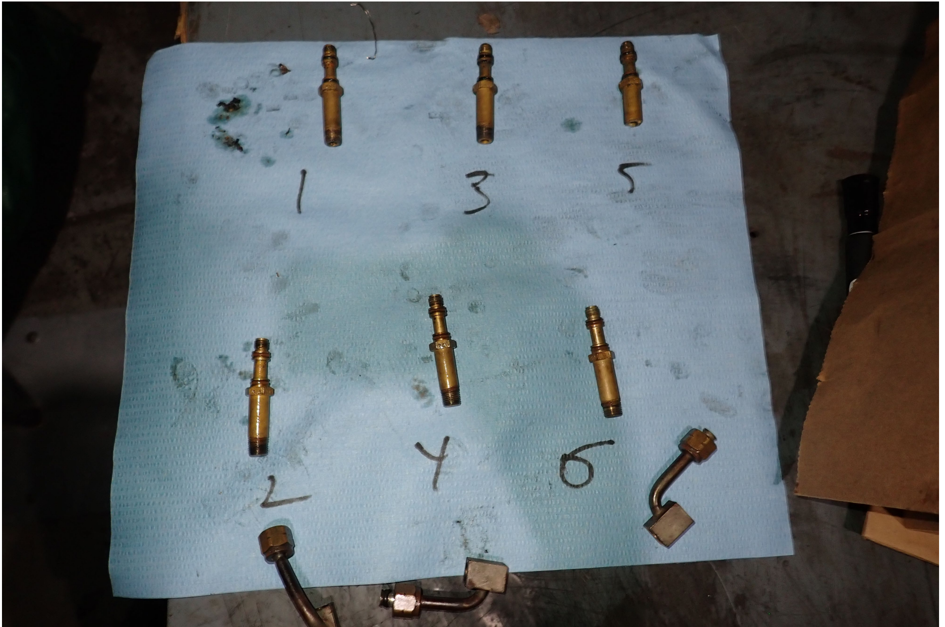
Photo 8 - Textron Aviation Digital Photograph. View of the Fuel Injector Nozzles.
