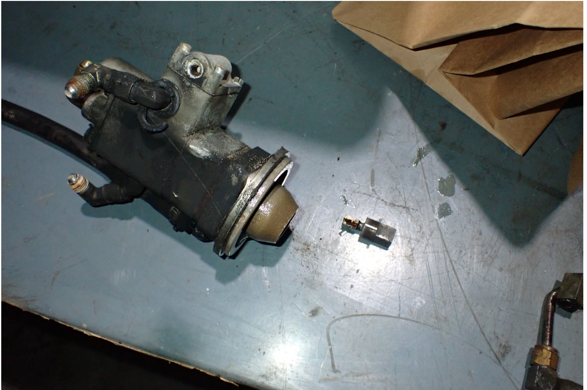
Photo 6 - Textron Aviation Digital Photograph. View of the Engine-Driven Fuel Pump and Intact Drive Coupling.
