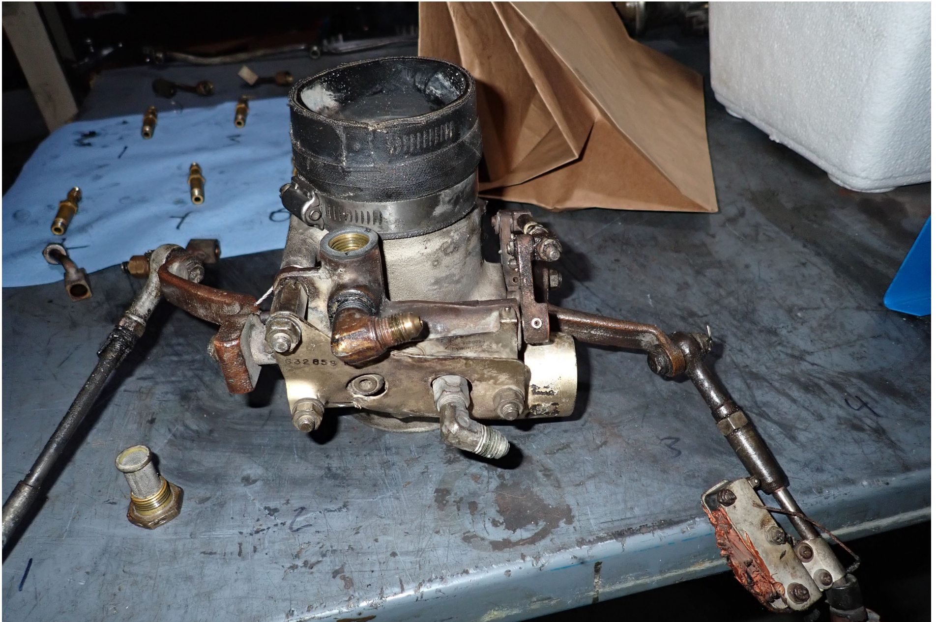
Photo 5 - Textron Aviation Digital Photograph. View of the Throttle Body and Metering Valve.
