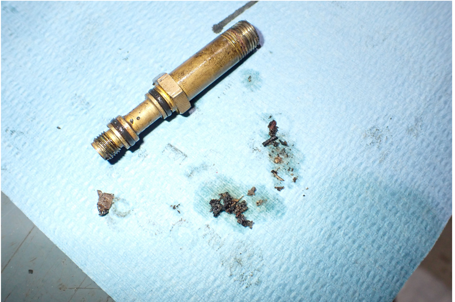
Photo 9 - Textron Aviation Digital Photograph. View of the Organic Material Removed from the No. 1 Cylinder Fuel Injector Nozzle.
