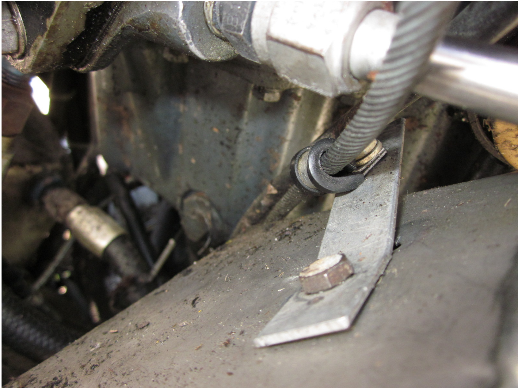
Photo 7 – Throttle Cable and Standoff Clamp Under Load – Courtesy of FAA
