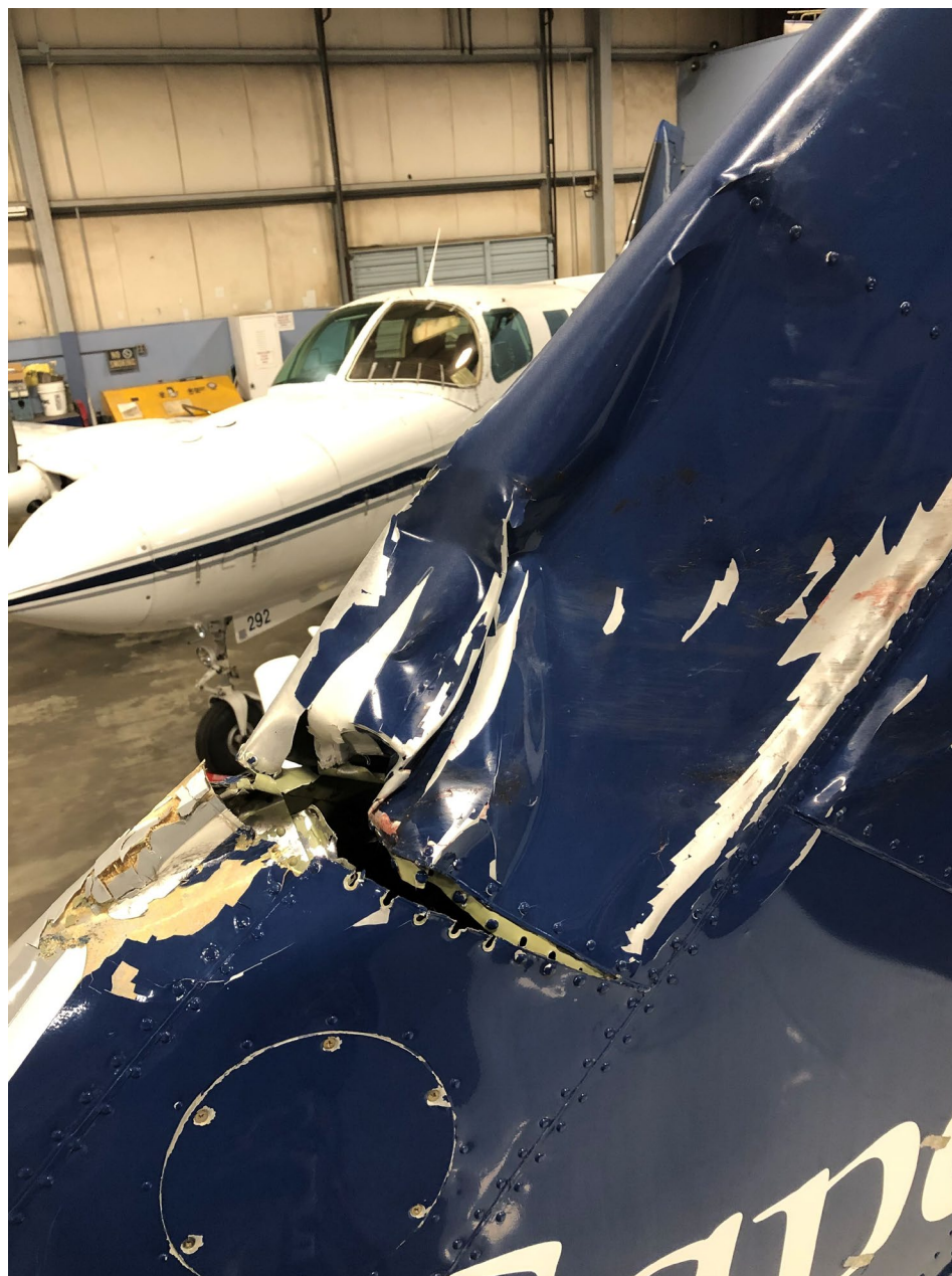
Photo 1 – View of damaged leading edge of vertical stabilizer
