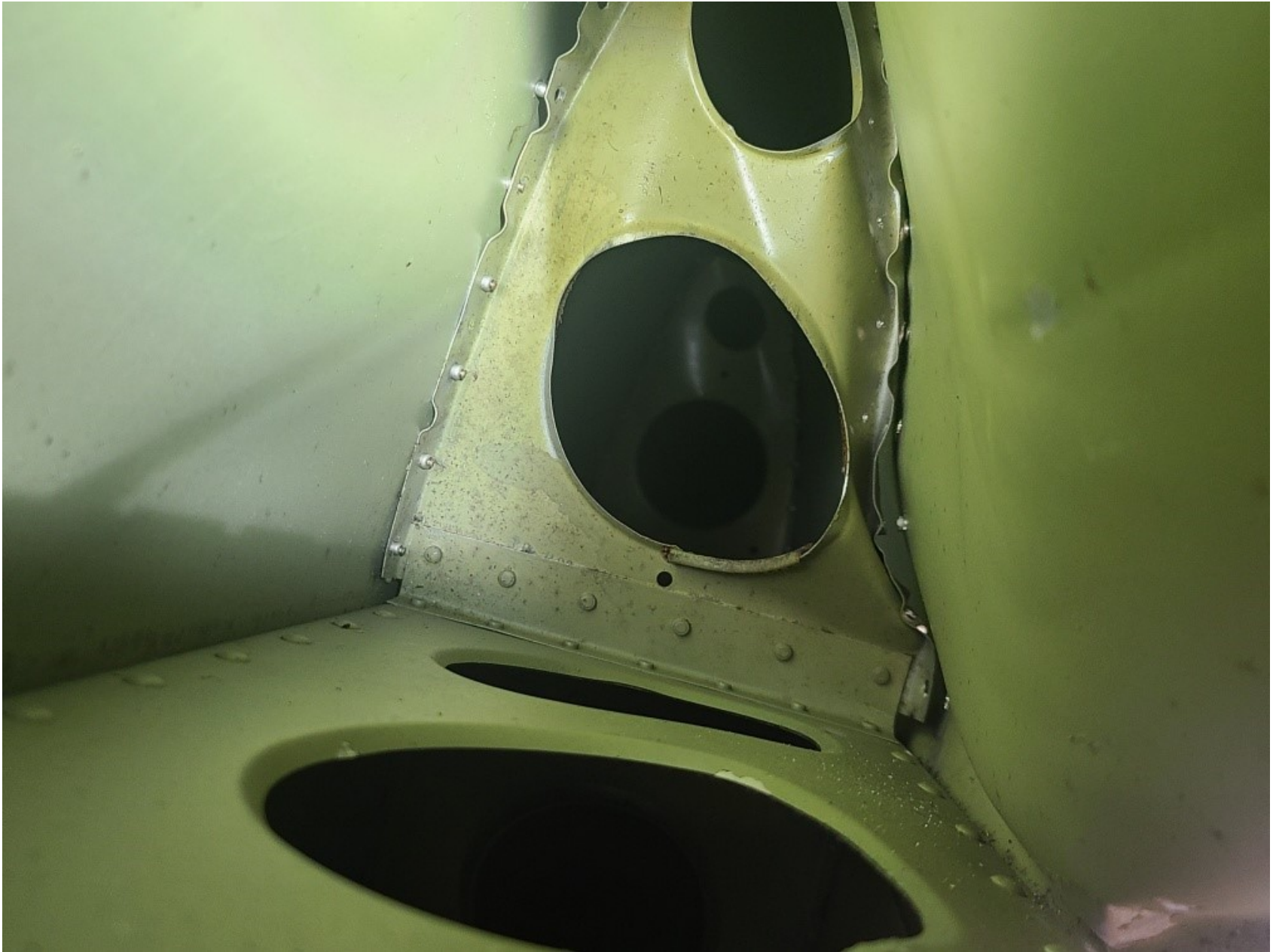
Photo 2 -View of buckled vertical stabilizer spar.
