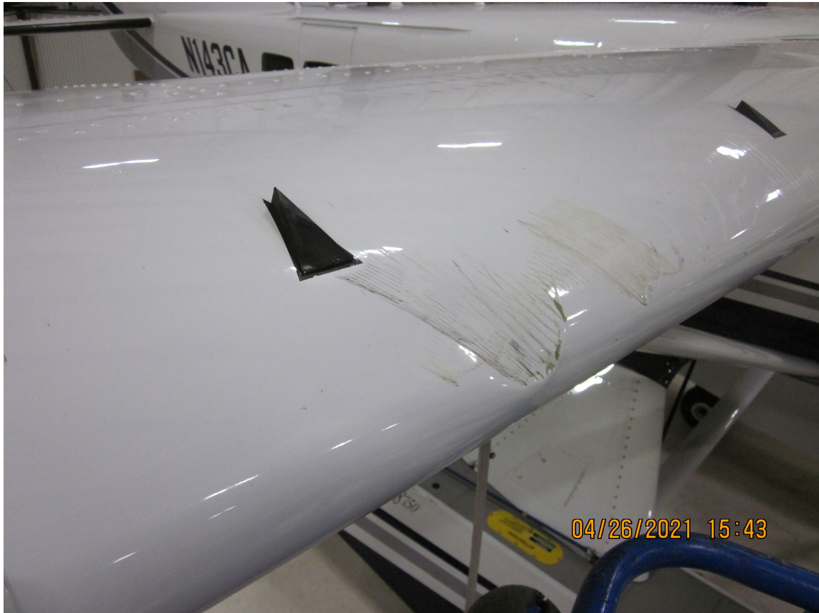
Photo 1 – View of leading edge of right wing damage. Note dent and wire strike impression marks. (Courtesy of FAA)
