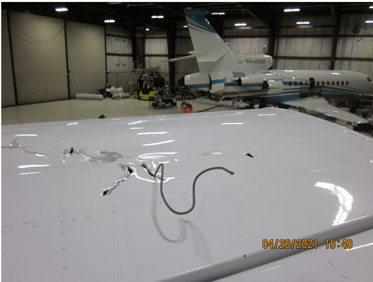
Photo 3 – View of top surface damage to right wing. Note multiple dents and tears in the skin and foreign object/wire protruding from surface. (Courtesy of FAA)
