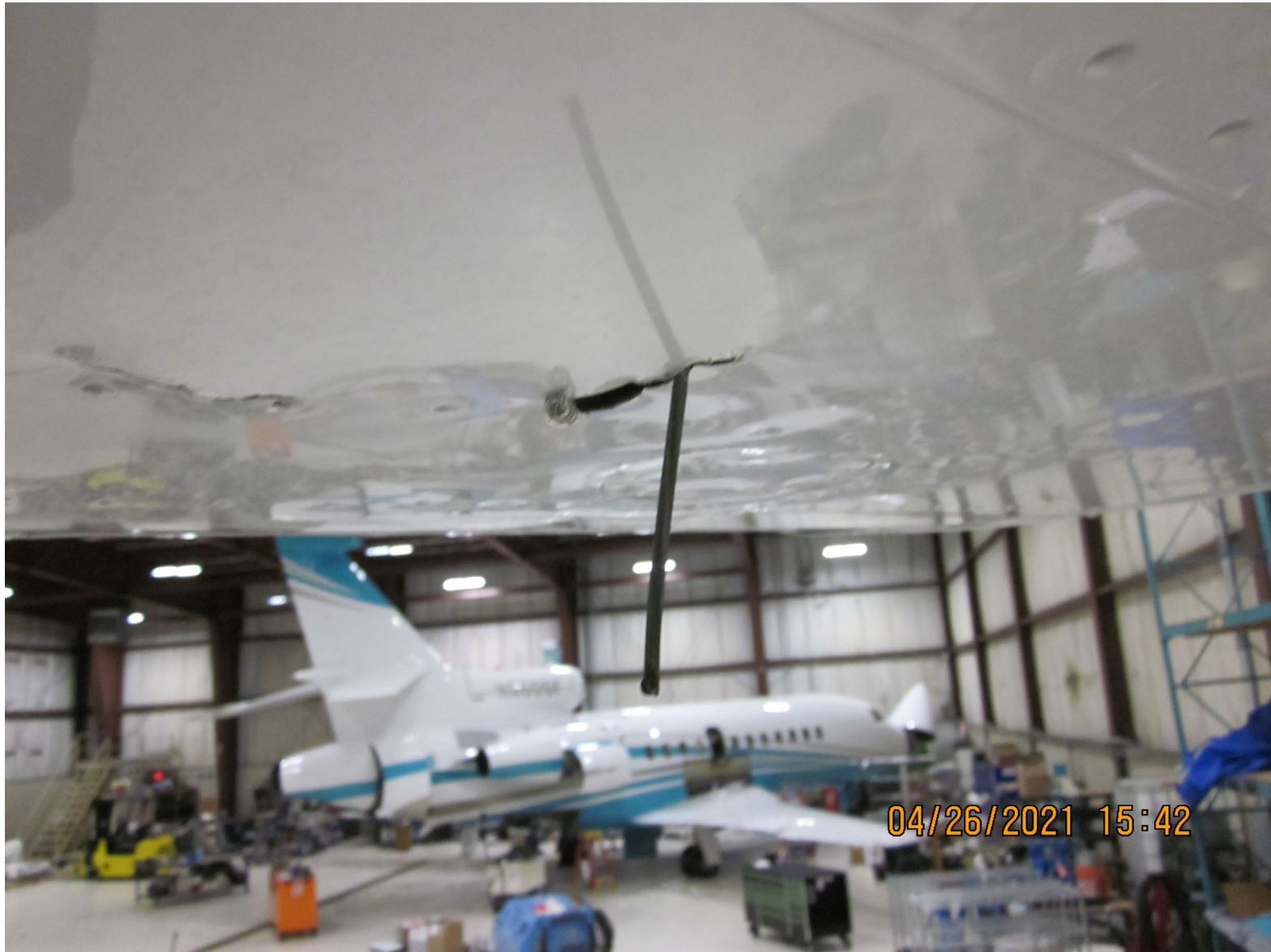
Photo 6 – View of tear to underside of right wing and foreign object/wire protruding from the interior of wing. (Courtesy of FAA)
