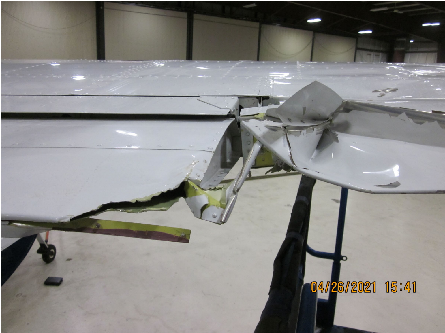
Photo 2 – Aft view of right wing outboard flap and inboard aileron damage. (Courtesy of FAA)
