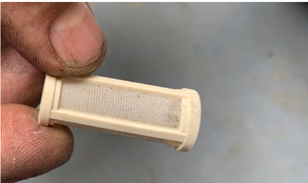
Figure 5: IMG_0183 Fuel Strainer
