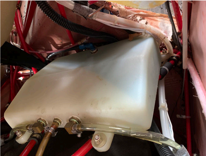
Figure 3: IMG_0151 Header Tank
