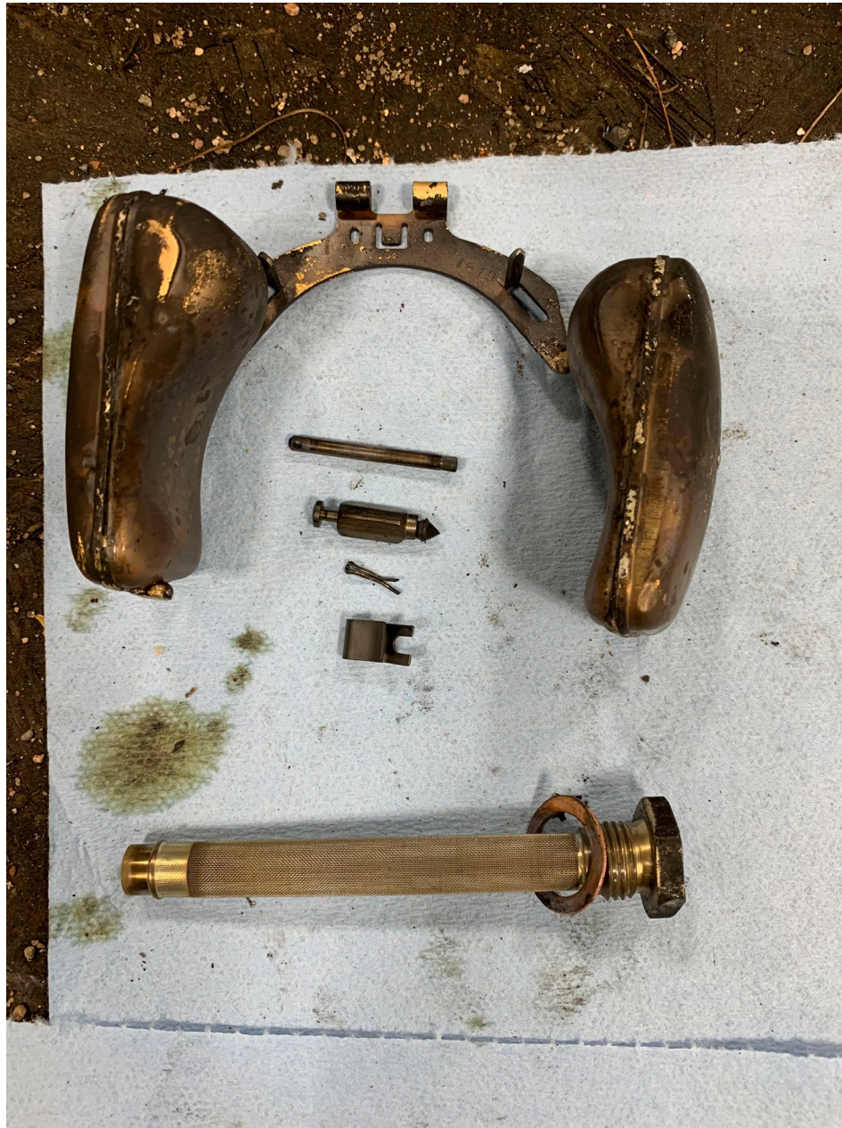
Photo 10 – Carburetor Floats and Fuel Screen (NTSB Photo)
