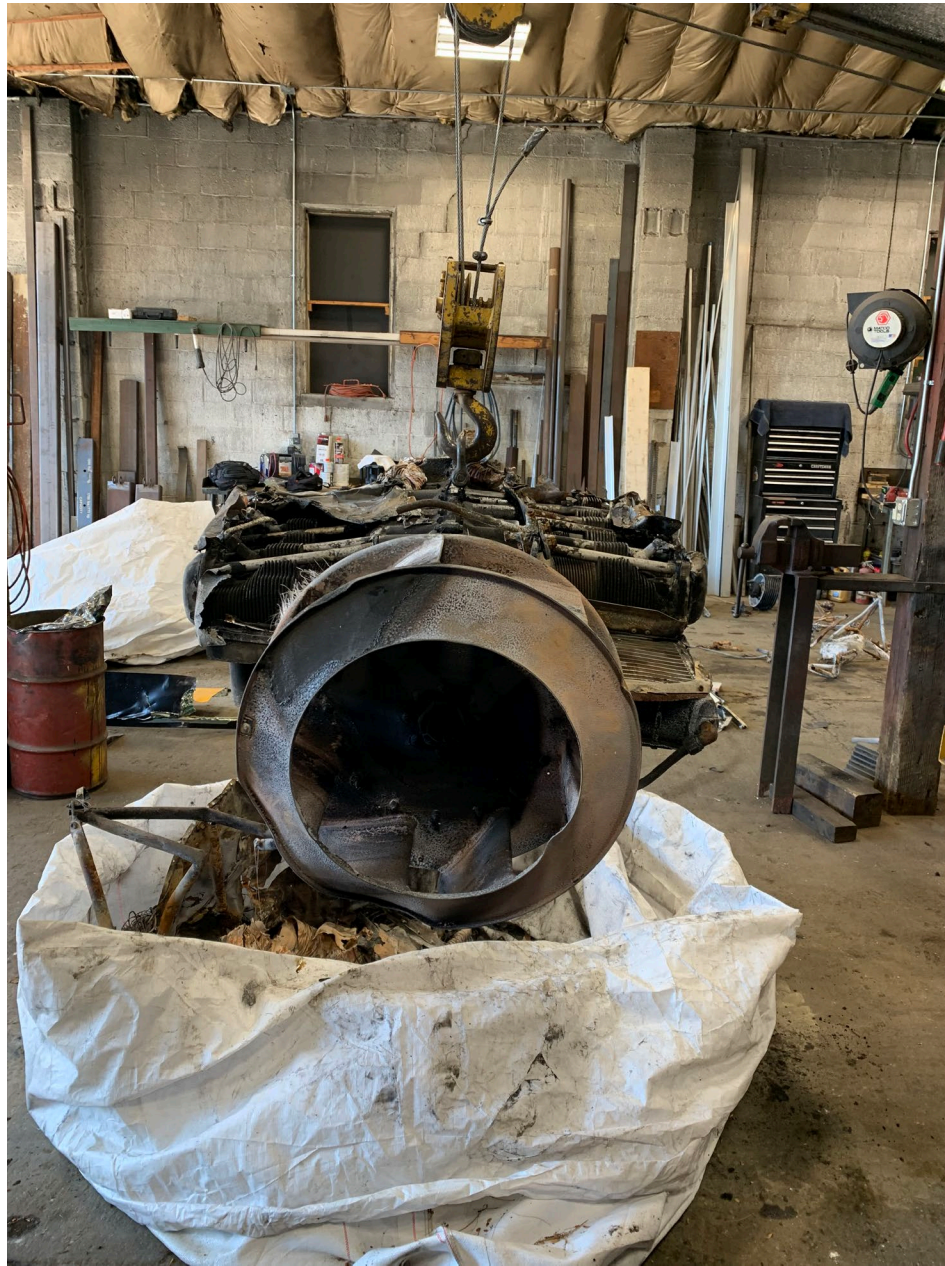
Photo 8 – Engine and Cooling Scroll (NTSB Photo)
